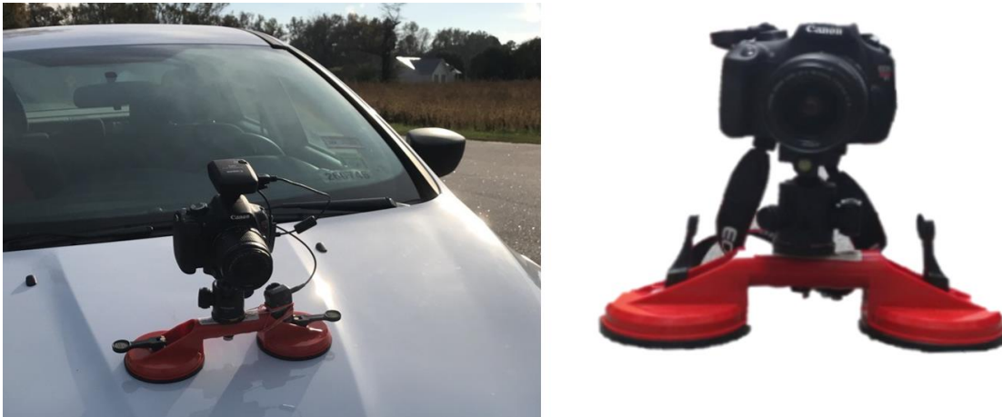
Figure 3.2. Camera with GPS unit attached mounted to hood of car.
