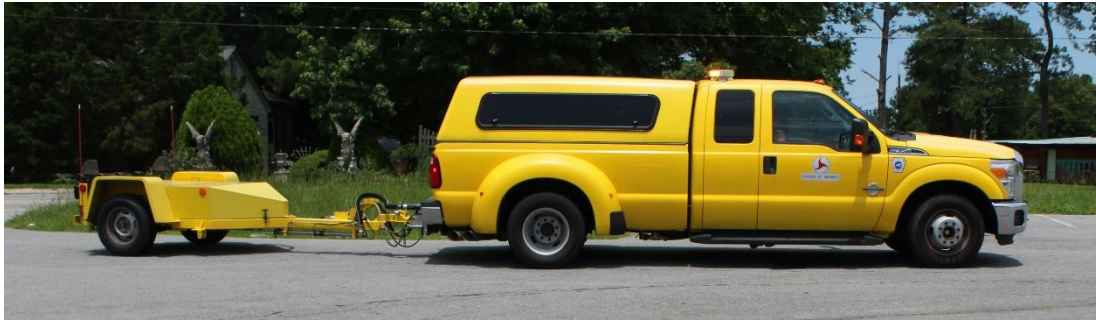
Figure 3.1. Locked-Wheel Skid Tester.
