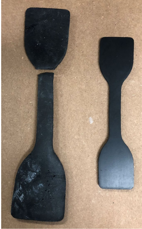
Figure 10: Swelling of neoprene specimen due to the prolonged exposure to benzene (13 weeks) at a high temperature of 140 °F. Left: Swollen specimen. Right: Unaged specimen for comparison.
