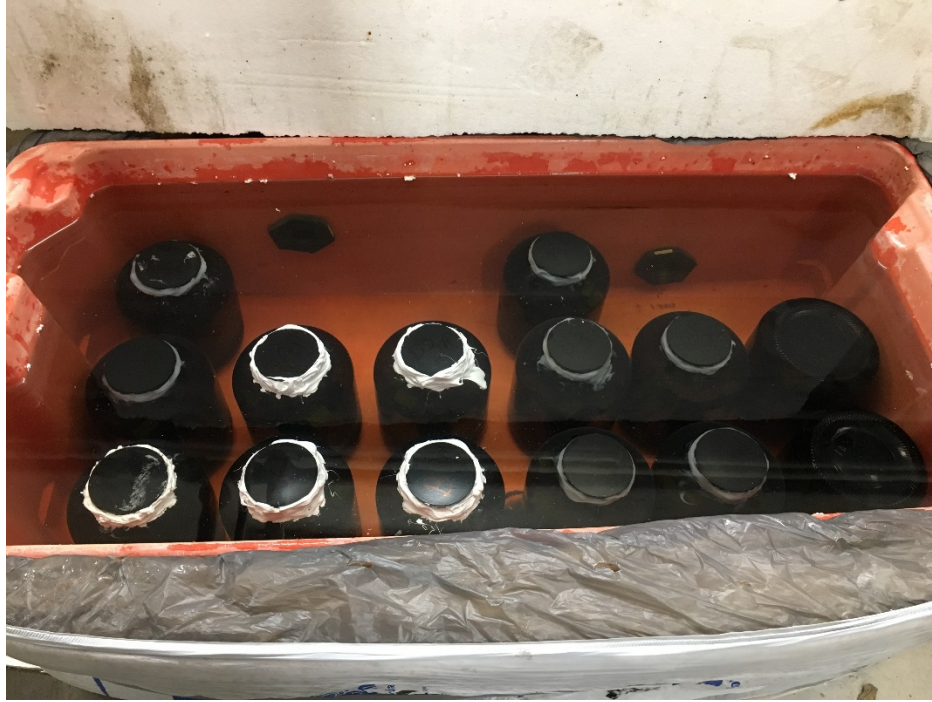
Figure B3: Insulated water bath with a control temperature system used for aging PVC pipe and rubber gasket specimens.
