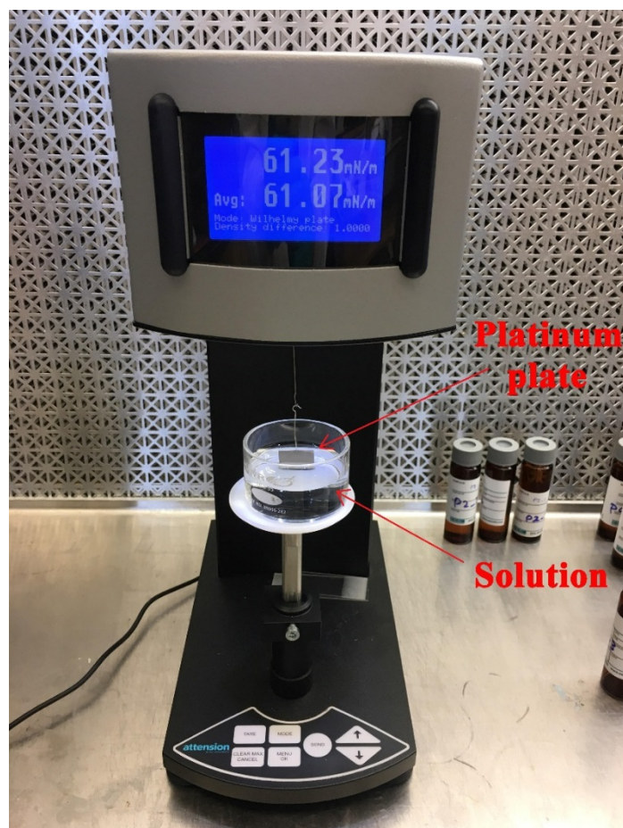
Figure B7: Liquid surface tension measurement test setup.
