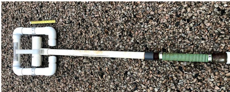
**Figure 12.** 2-inch skimmer with 13mm plug orifice
