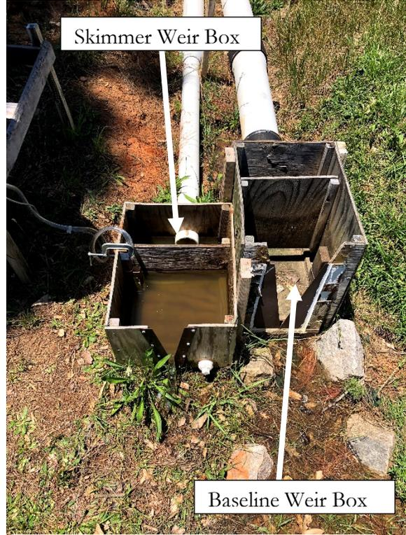
**Figure 21.** Outlet weir boxes with un-pictured ISCO sampler to the left
