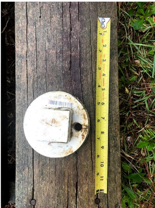
**Figure 7.** Baseline outlet orifice drilled into outlet pipe cap
