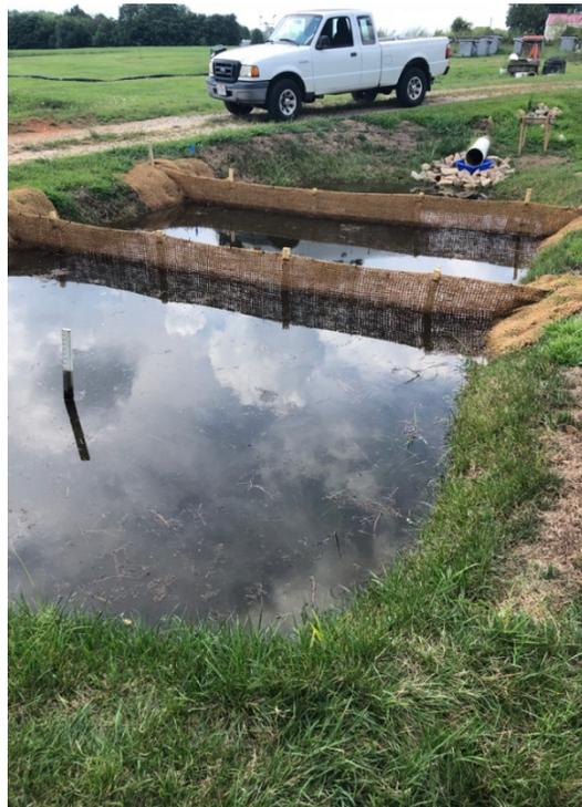
**Figure 10.** DDB with porous baffles
