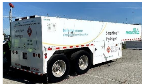
Figure 3-7: Hydrogen Distribution and Storage in Gas Tube Trailer 200 bar trailer on the left and 450 bar mobile refueler on the right (Hoffrichter, 2009, 2019)
