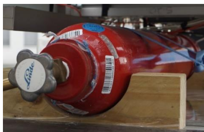
Figure 3-8: 200 bar Compressed Hydrogen Cylinder Installed in a Hydrogen Locomotive Courtesy and Copyright Jonathan Tutcher, 2012
