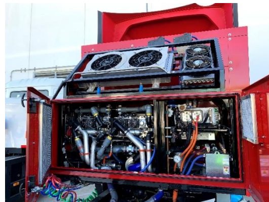
Figure 3-16: Examples of Fuel Cell Systems; train module (left) and truck (right) (Hoffrichter, 2019)
