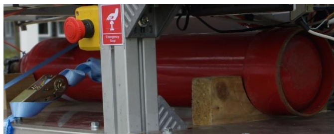
Figure 3-8: 200 bar Compressed Hydrogen Cylinder Installed in a Hydrogen Locomotive Courtesy and Copyright Jonathan Tutcher, 2012
