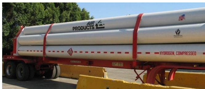
Figure 3-7: Hydrogen Distribution and Storage in Gas Tube Trailer 200 bar trailer on the left and 450 bar mobile refueler on the right (Hoffrichter, 2009, 2019)
