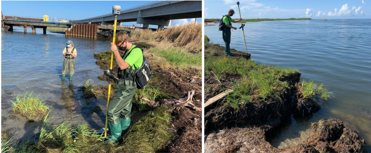
**Figure 6.** Trimble GPS System and Shoreline Surveys (August 2020).
