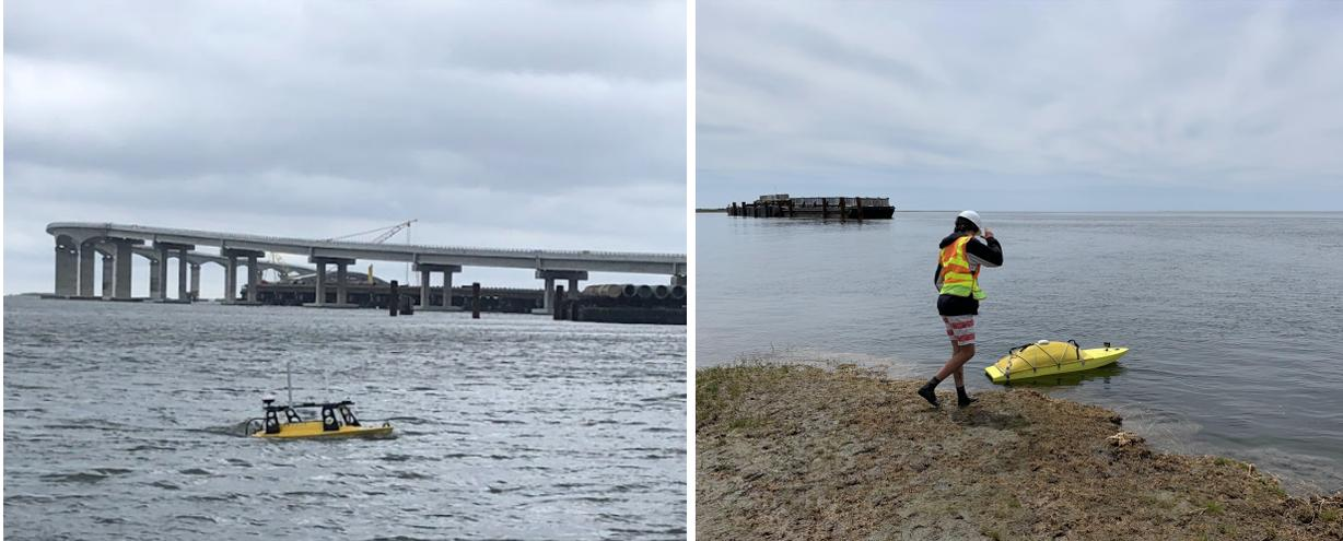
**Figure 7.** Z-boat measuring channel bathymetry using a single-beam echosounder (left hand image, October 2019); remotely-driven kayak measuring bathymetry (right hand image, April 2021).
