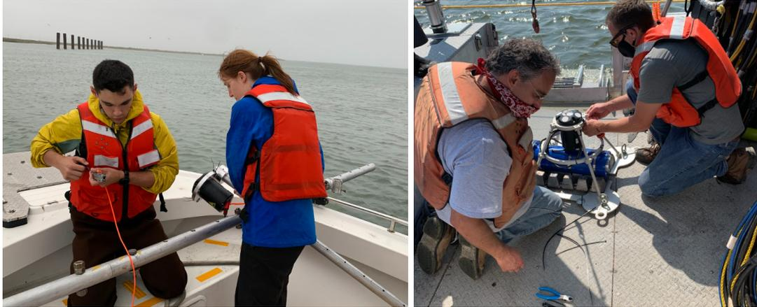
**Figure 4.** Spatial variability in currents were measured from a boat in 2019 and 2021 (left hand image, October 2019) and temporal variability in currents were measured from a bottom structure in 2020 (right hand image, August 2020).
