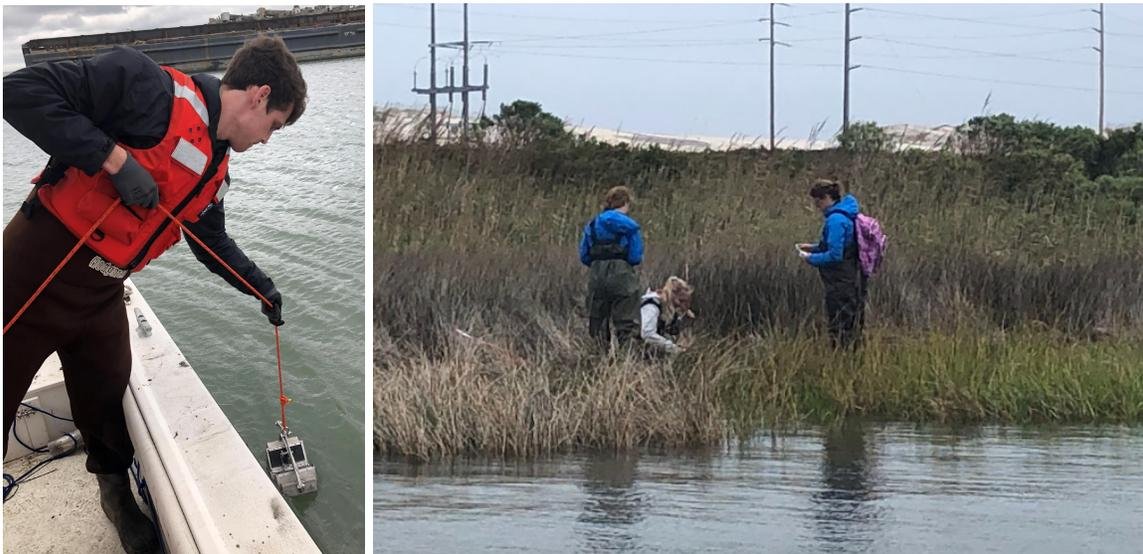
**Figure 8.** Seafloor sediment samples were taken with a grab sampler (left hand image, October 2019) and sediment samples on land were gathered with a trowel (right hand image, October 2019).
