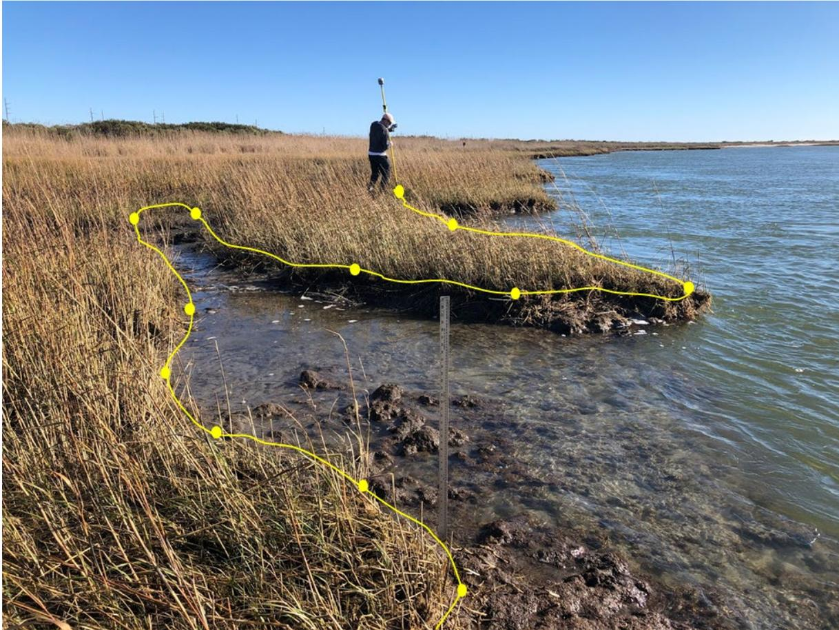
Figure 1. Marsh edge survey in progress, November 25, 2019. Points were surveyed via GPS at approximately 2 m to 25 m spacing, depending on marsh edge morphology.
