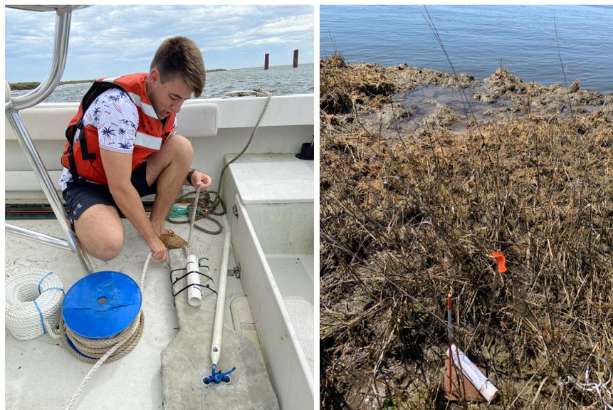
**Figure 5.** To measure water levels, pressure gauges were deployed in PVC cases on concrete structures near the shoreline edge (left hand image, September 2021). Marsh flood depth was measured by a pressure gauge in a PVC case fixed to the ground (right hand image, March 2020).
