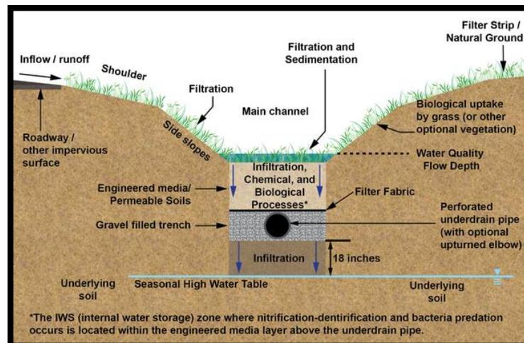
Figure A-2: Typical cross-section of a bioswale and its stormwater treatment processes (taken from Ekka and Hunt, 2020).
