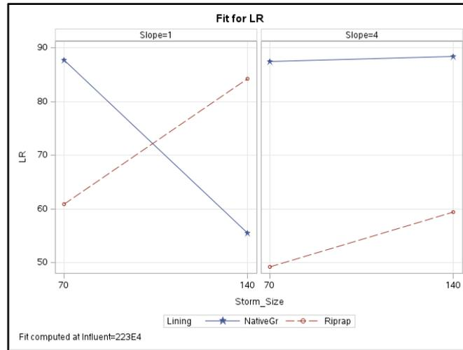
Figure G-13: Zn load reduction lining\*storm size interaction plot.
