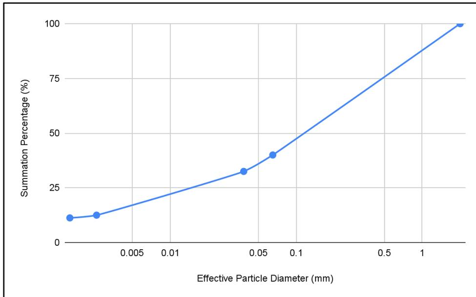
Figure D-8: Particle size distribution of onsite soil.
