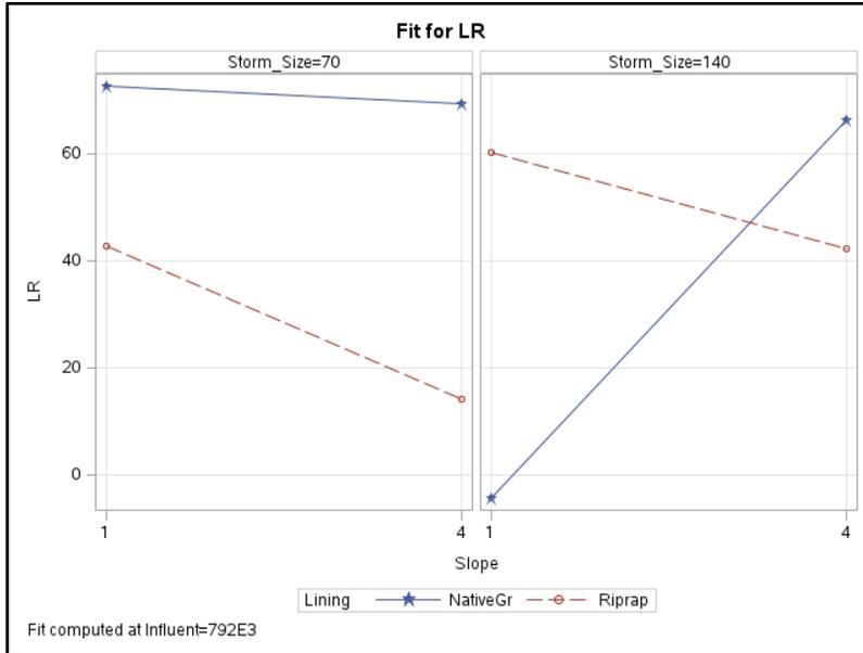
Figure G-2: NH<sub>3</sub> load reduction lining\*slope interaction plot.
