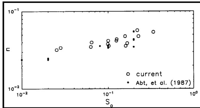
Figure A-7: Manning's  $n$  vs. bed slope (taken from Rice et al., 1998).
