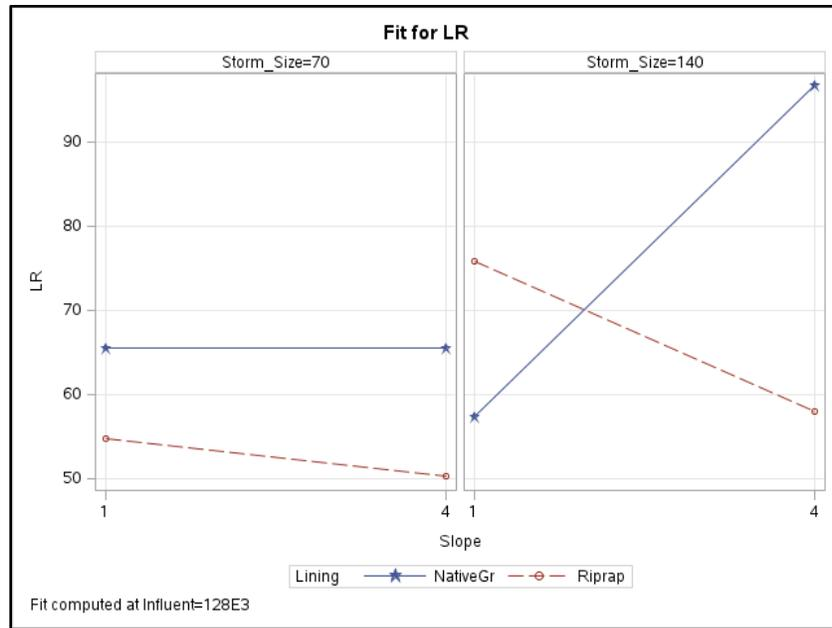
Figure G-11: Pb load reduction lining\*slope interaction plot.
