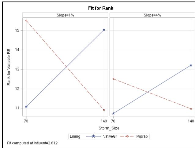
Figure I-5: Cd underdrain lining\*storm size interaction plot.
