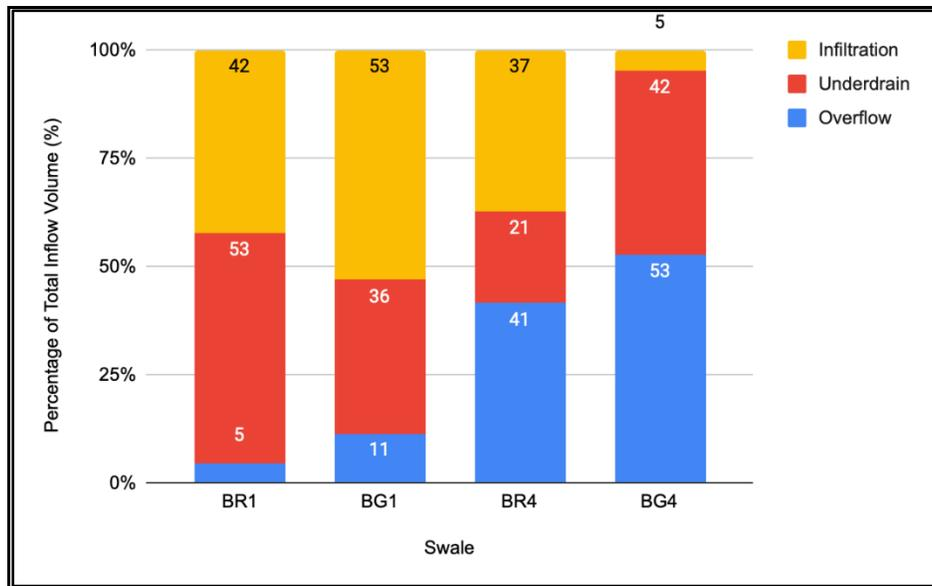
Figure3-1: Hydrologic pathways in bioswales as a percentage of the total inflow volume measured during medium storm events.
