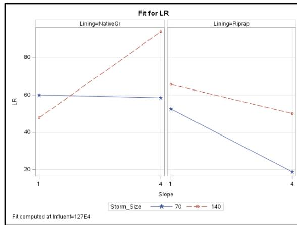
Figure G-8: OP load reduction storm size\*slope interaction plot.
