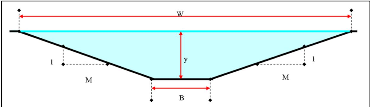
Figure N-5: Schematic of swale cross-section (taken from NCDEQ, 2017).
