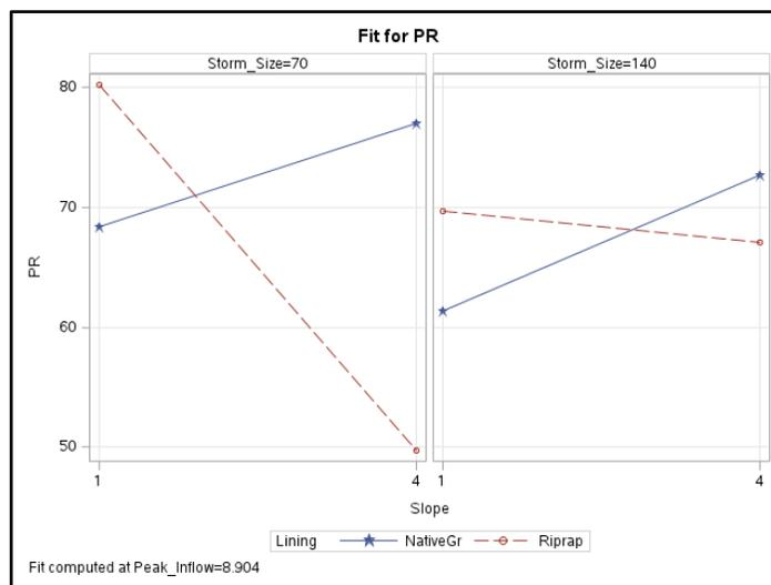
Figure E-2: Peak flow reduction lining\*slope interaction plot.
