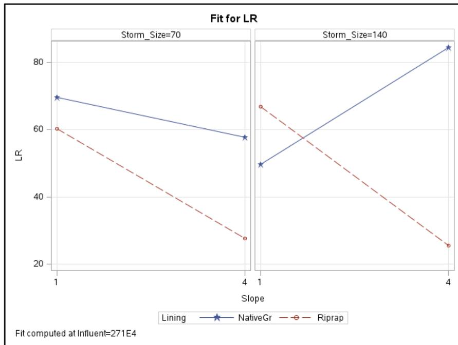
Figure G-6: TP load reduction lining\*slope interaction plot.
