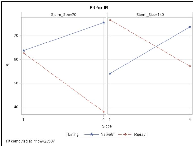
Figure E-1: Volume reduction lining\*slope interaction plot.
