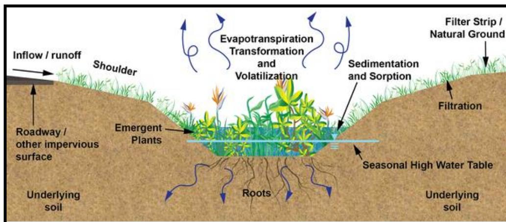
Figure A-6: Typical cross-section of a wet swale and its stormwater treatment processes (taken from Ekka and Hunt, 2020).
