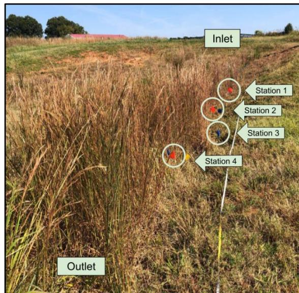
Figure N-1: Flags (circled) placed according to depth of flow.
