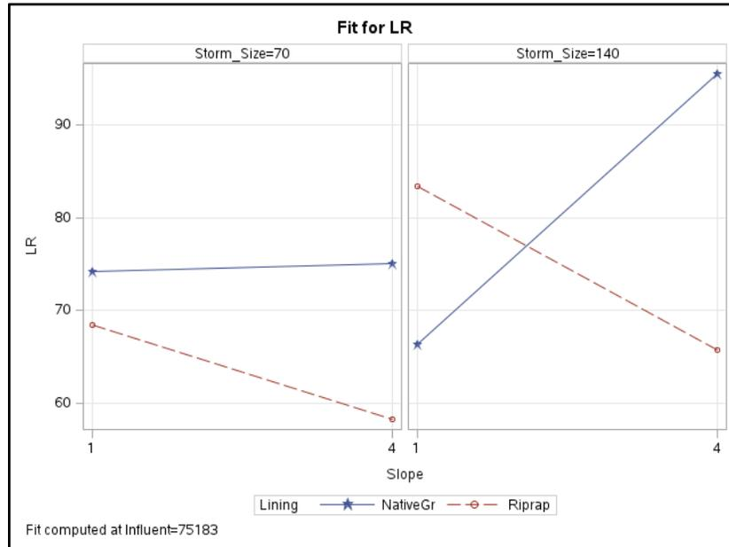
Figure G-9: Cd load reduction lining\*slope interaction plot.
