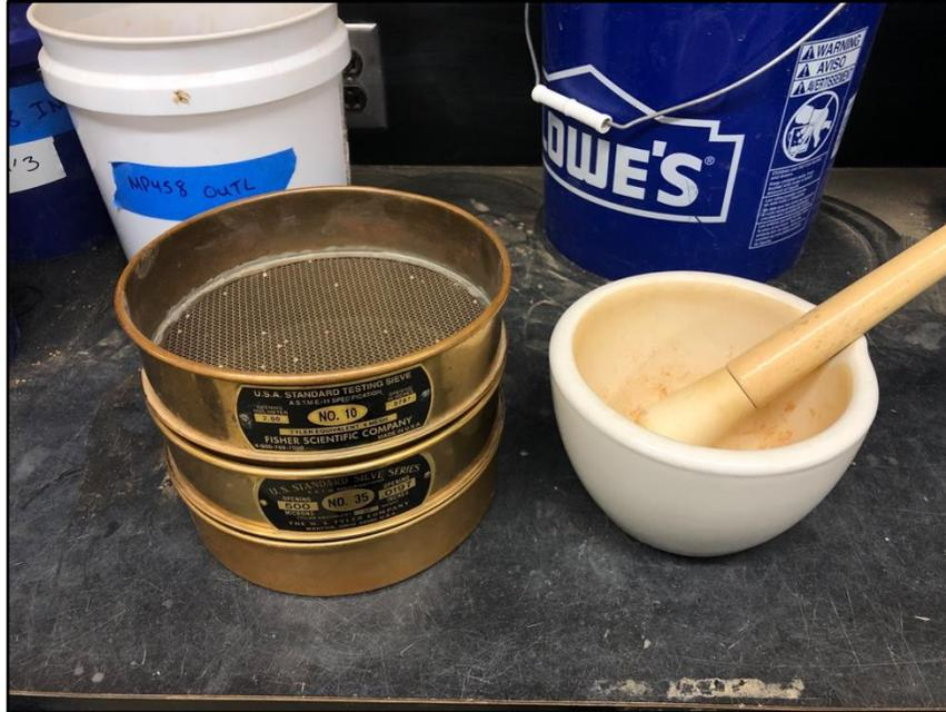
Figure D-3: ASTM sieves #'s 10 and 35 with mortar and pestle used to prepare pollutant spikes.
