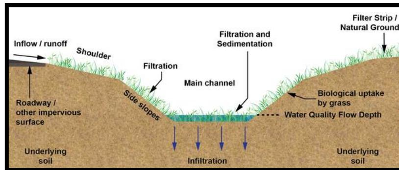
Figure A-1: Typical cross-section of a grass swale and its stormwater treatment processes (taken from Ekka and Hunt, 2020).
