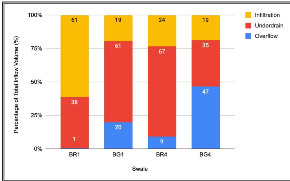
Figure 3-2: Hydrologic pathways in bioswales as a percentage of the total inflow volume measured during large storm events.
