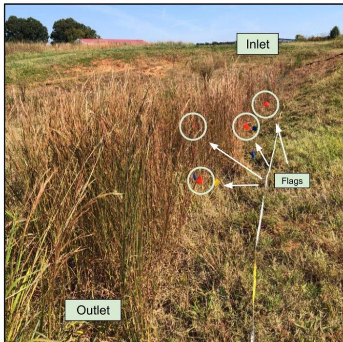
Figure D-9: Flags placed for Manning's roughness experiment.
