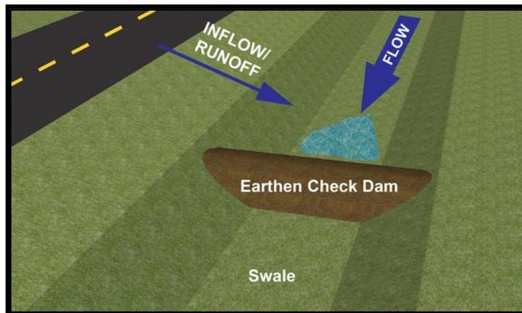
Figure A-4: Stylized cross-section of an infiltration swale with inclusion of a check dam (taken from Ekka and Hunt, 2020).
