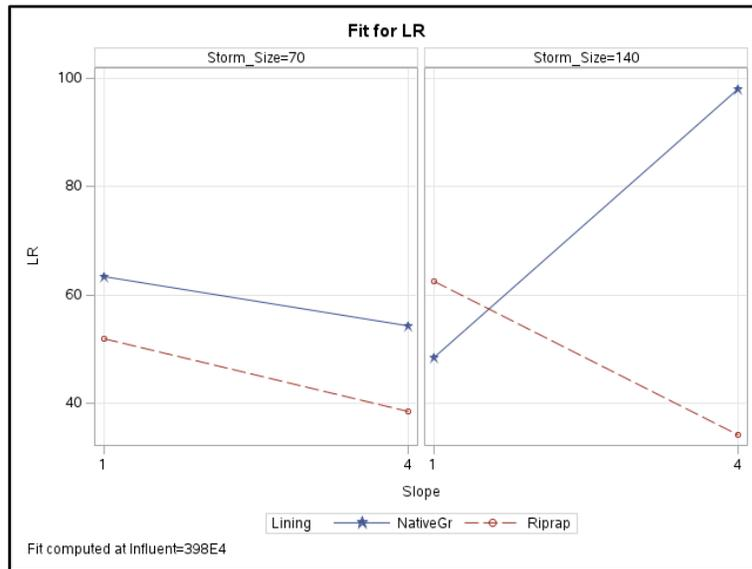
Figure G-4: NO<sub>x</sub> load reduction lining\*slope interaction plot.
