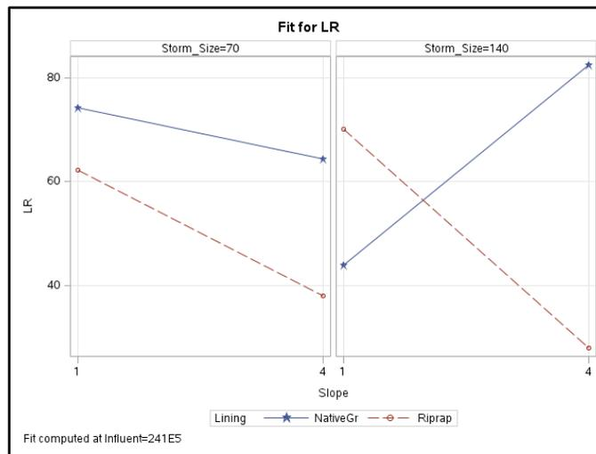
Figure G-5: TN load reduction lining\*slope interaction plot.
