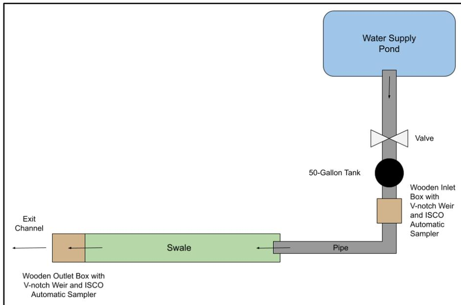
D-2: Conceptual swale experimental setup.
