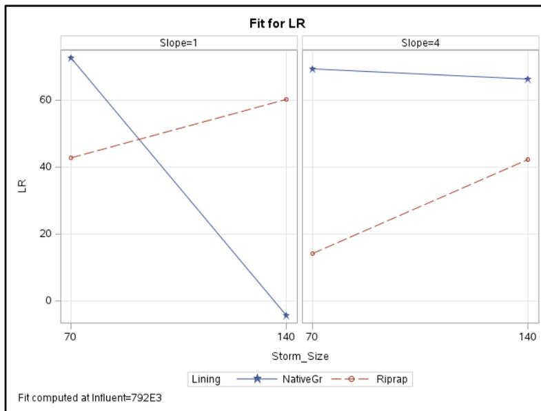
Figure G-3: NH<sub>3</sub> load reduction lining\*storm size interaction plot.
