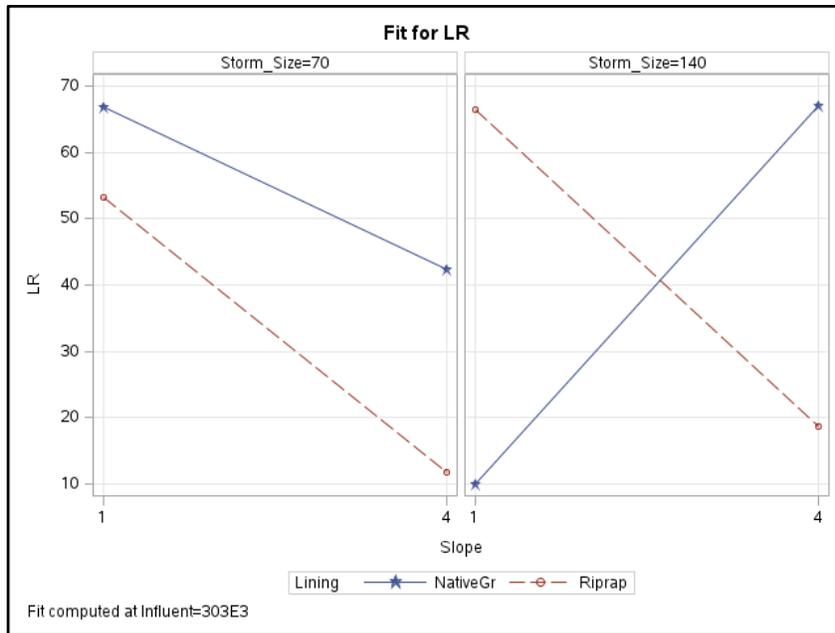
Figure G-10: Cu load reduction lining\*slope interaction plot.
