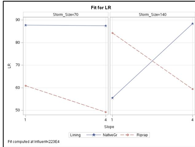
Figure G-12: Zn load reduction lining\*slope interaction plot.
