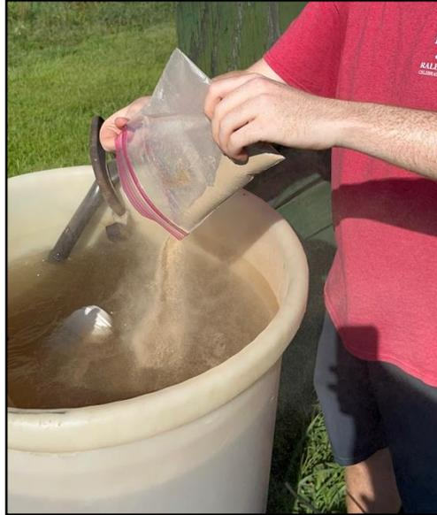
Figure D-4: Spiked sample mixing with water.
