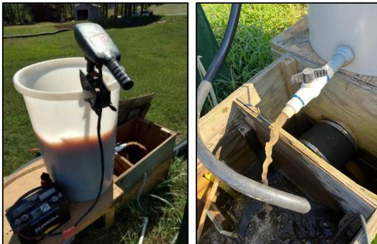
Figure 1-3: 50-gallon tank to simulate synthetic runoff (left). Spiked pond water discharging from tank into inlet box (right).
