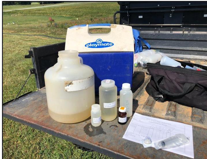
Figure D-5: Composite samples for lab analyses.
