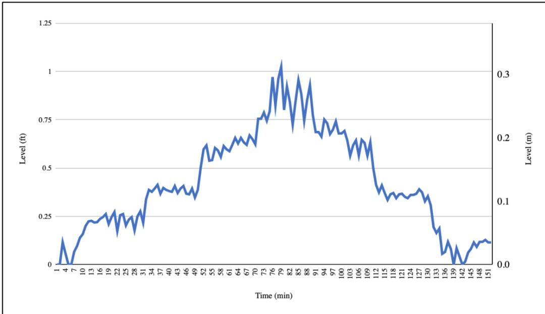
Figure D-1: Example center-weighted hydrograph for experiment of swale BG4 on 7/7/2022.
