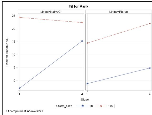
Figure I-2: Total volume reduction storm size\*slope interaction plot.
