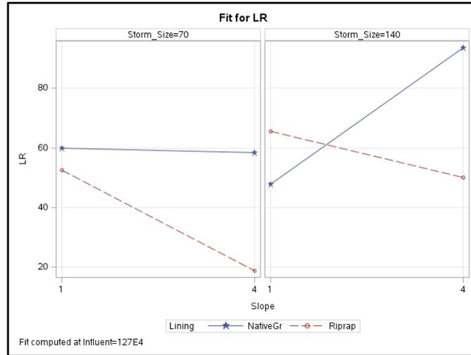
Figure G-7: OP load reduction lining\*slope interaction plot.
