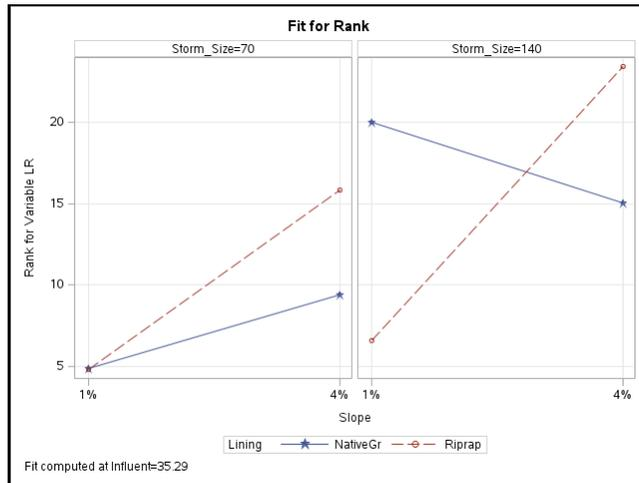
Figure I-7 OP load reduction slope\*storm size interaction
