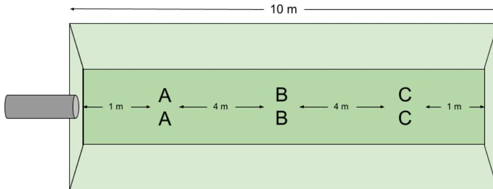
Figure D-7: Bulk density sampling placement.
