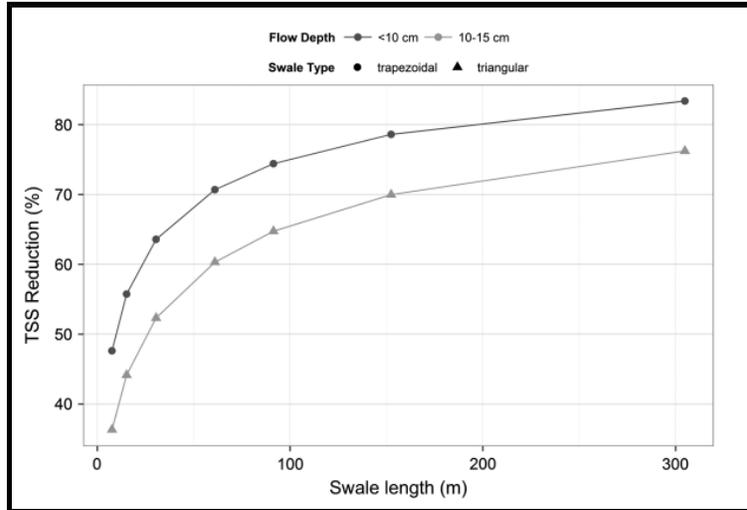
Figure A-5: TSS reduction (%) as a function of swale length for triangular and trapezoidal swales with 6:1 side slope, 1.5% longitudinal slope, and 0.1-ha catchment area (taken from Winston et al., 2017).
