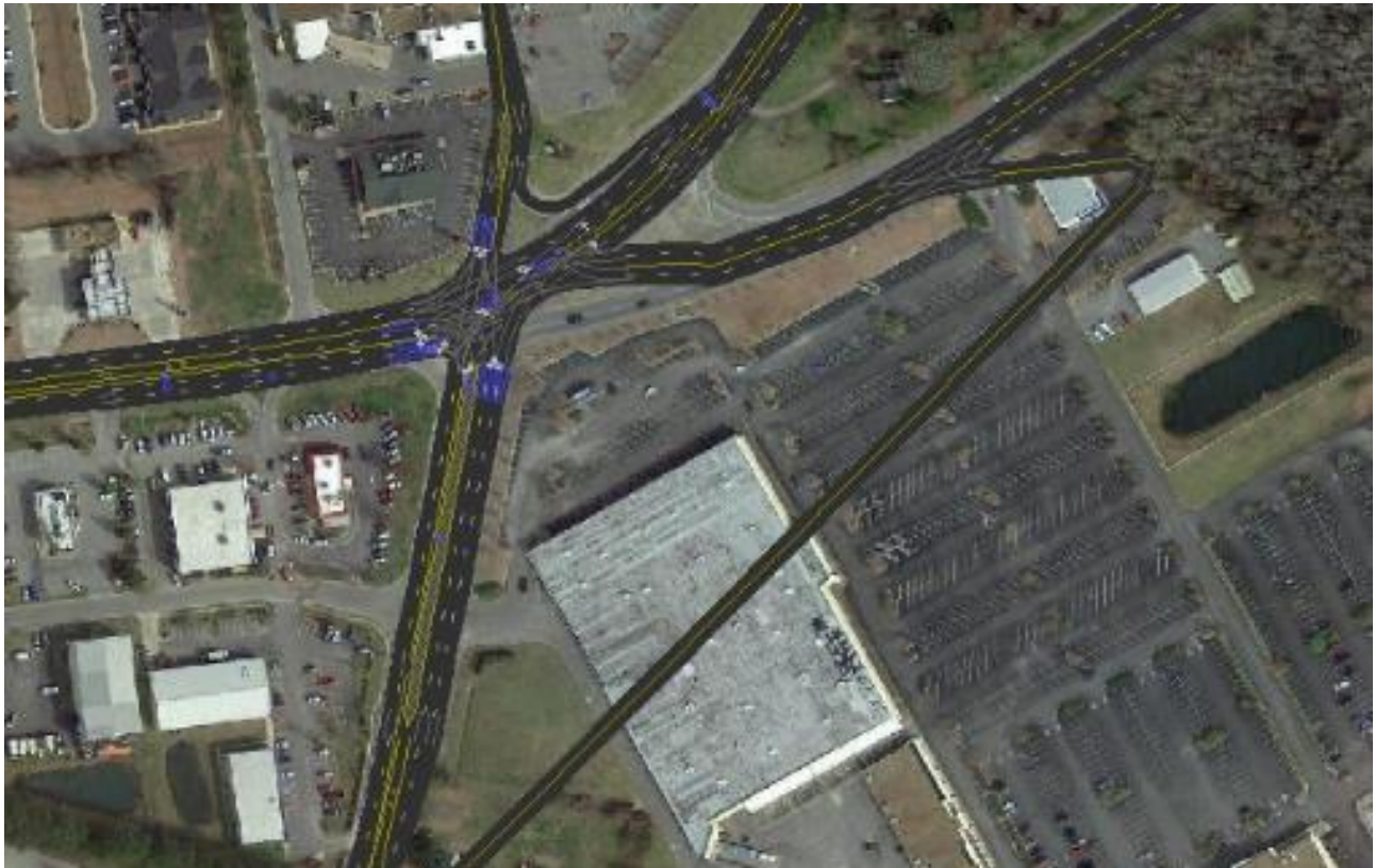
Figure 15. Example of the faulty road connections found and corrected in the road network.
