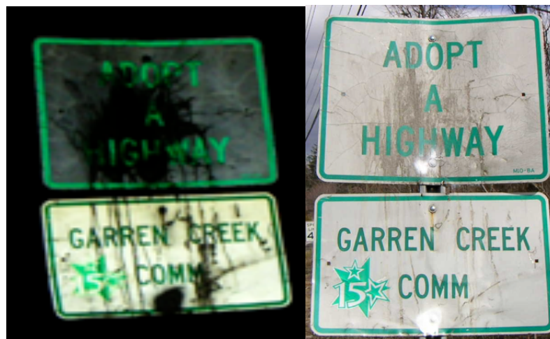
Figure 7.9. Night and Day Time Comparison of Sign Damaged with Paint Ball, Egg, and Sticker
