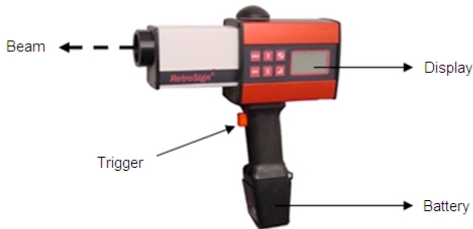
Figure 4.1. A handheld retroreflectometer (RetroSign®4500)
