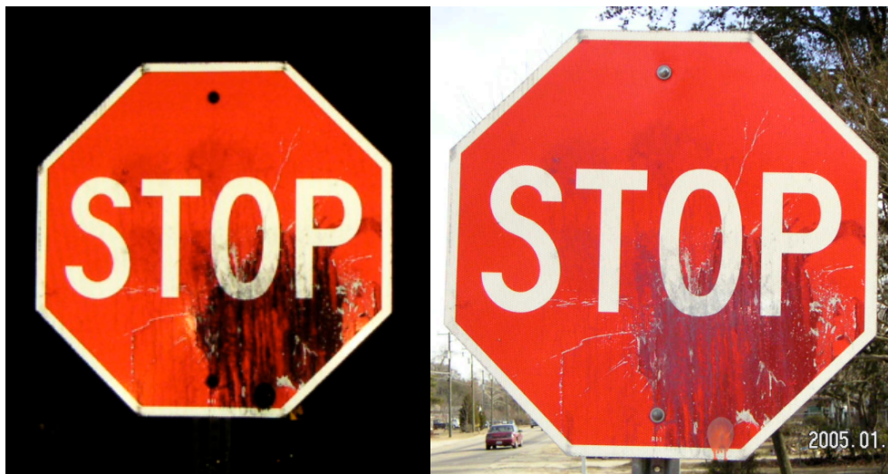
Figure 7.10. Night and Day Time Appearance of Sign with Paint
