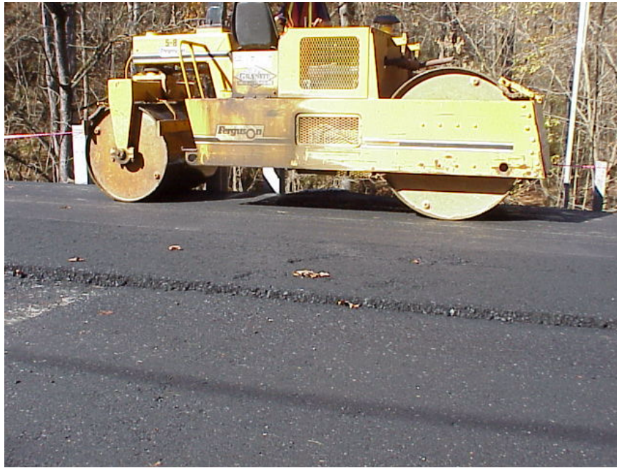
Figure 25: Vibratory Drum Roller
