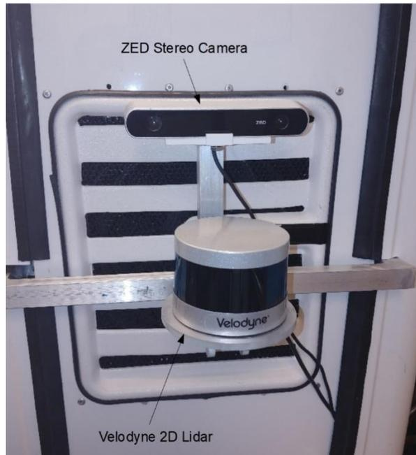
Figure 7 Front of vehicle showing Stereo Camera and 2D Lidar.
