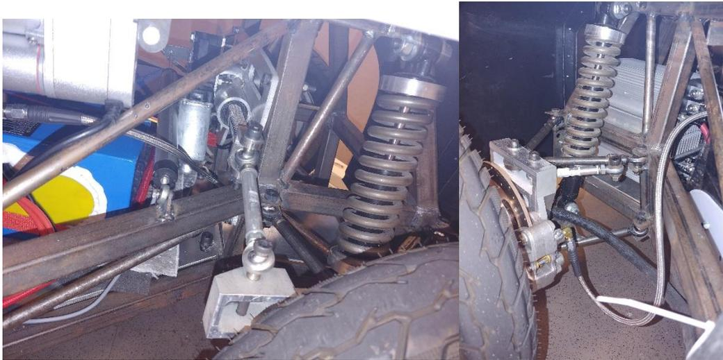
Figure 8 Front and back suspension geometries for generation 2.5 vehicle.
