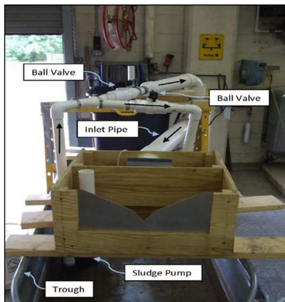
Figure E-3: Pump and Pipe Network
