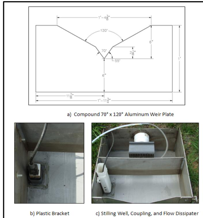
Figure 3.7 Weir Box Components
