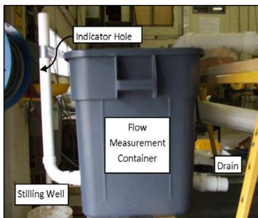
Figure E-4: Flow measurement container
