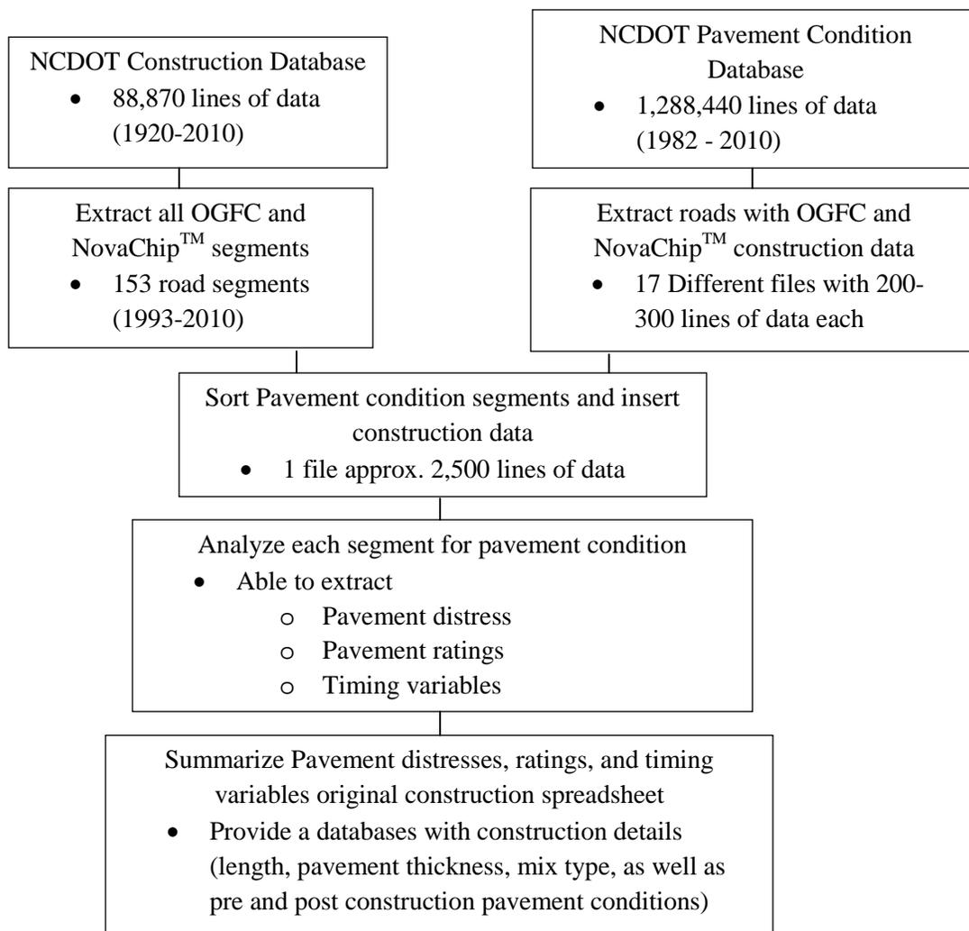
Figure 2.1 Data retrieval from NCDOT Pavement Construction and Condition Database
