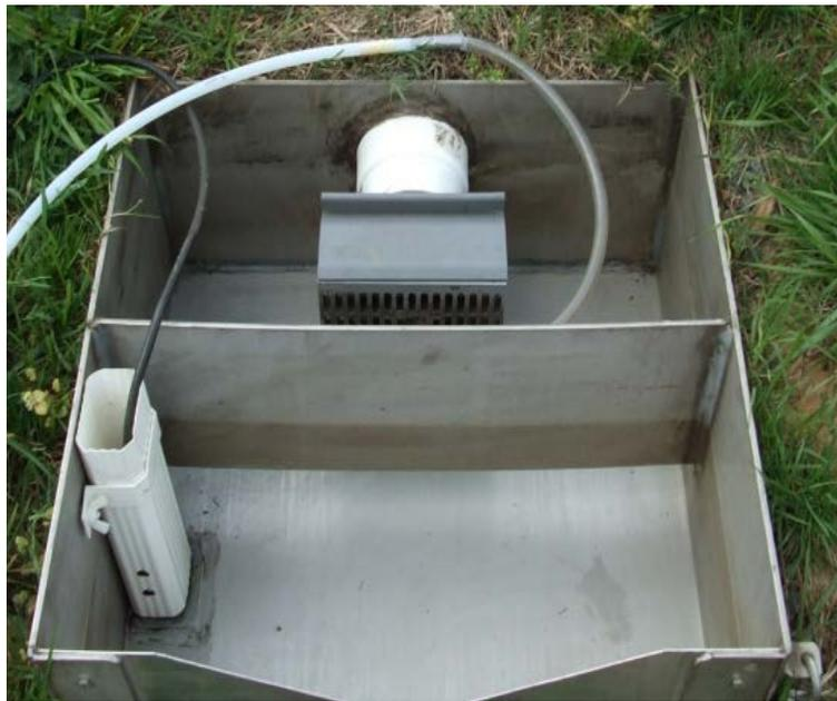
Figure E-2: Stilling well and Flow Dissipater
