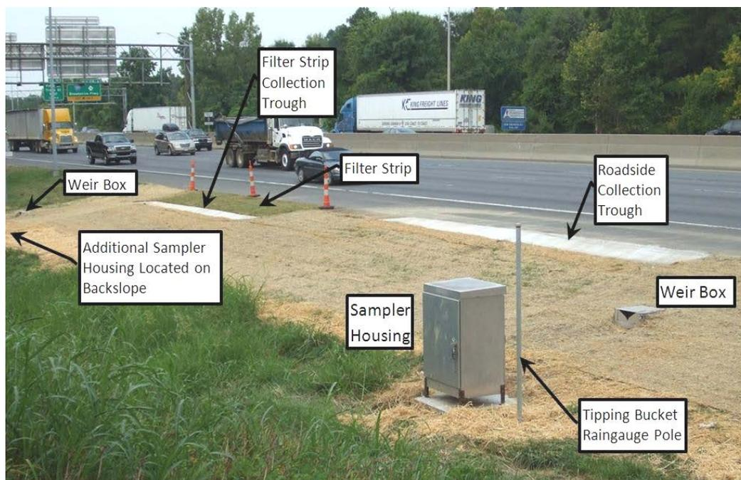
Figure 3.6 Photograph of Post Construction Site Setup
