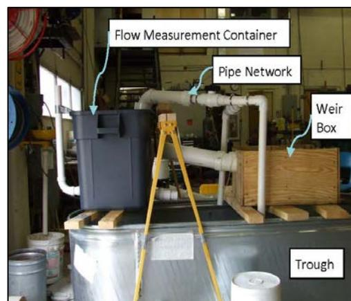
Figure E-5: Fully assembled testing apparatus
