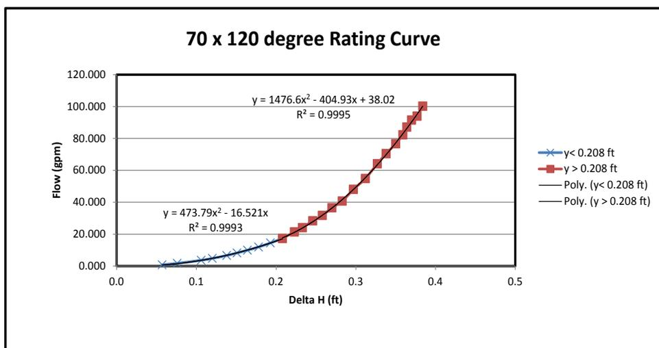
Figure E-6: 70 x 120 Degree Compound V-notch Rating Curve
