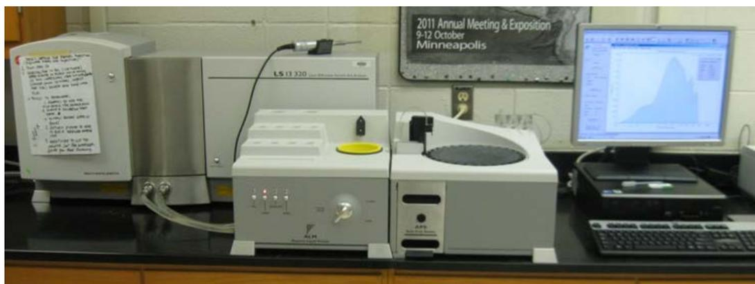
Figure 7.1 Beckman Coulter LS 13 320 Laser Diffraction Particle Counter Settleable Solids
