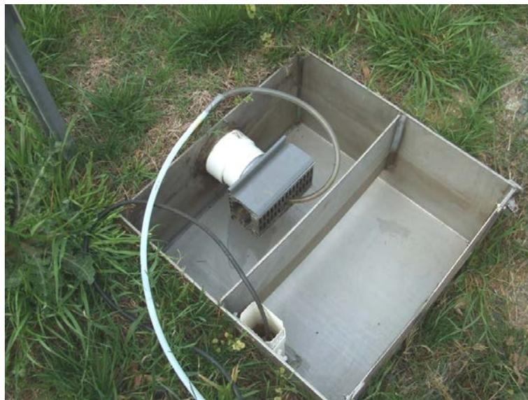
Figure 3.8 Pre-Storm Event Weir Box Setup
