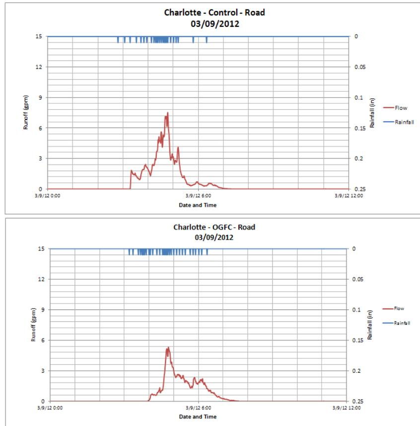
Figure 4.2 Hydrograph Lag Observed at COR\_EOP and CCR\_EOP Sites for Storm No. 16
