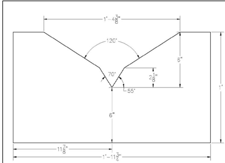
Figure E-1: 70 x 120 degree Compound Weir Plate
