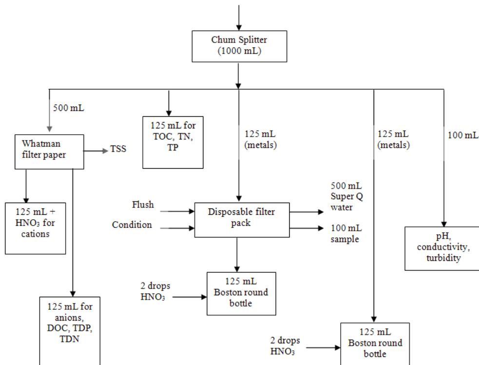
Figure D-1: Sampling Processing Flow Chart
