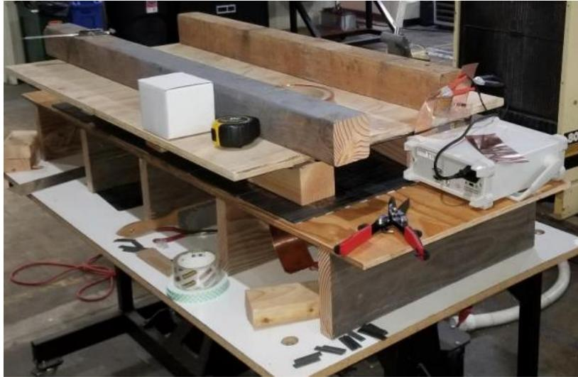
*Figure 3.48 Preliminary subscale system assembly for measurement of inductance, resistance and coupling factor used in further simulations*
