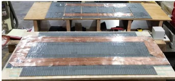
Figure 3.50 Mockup Hardware of single turn 4 pad transmitter and 2 turn receiver
