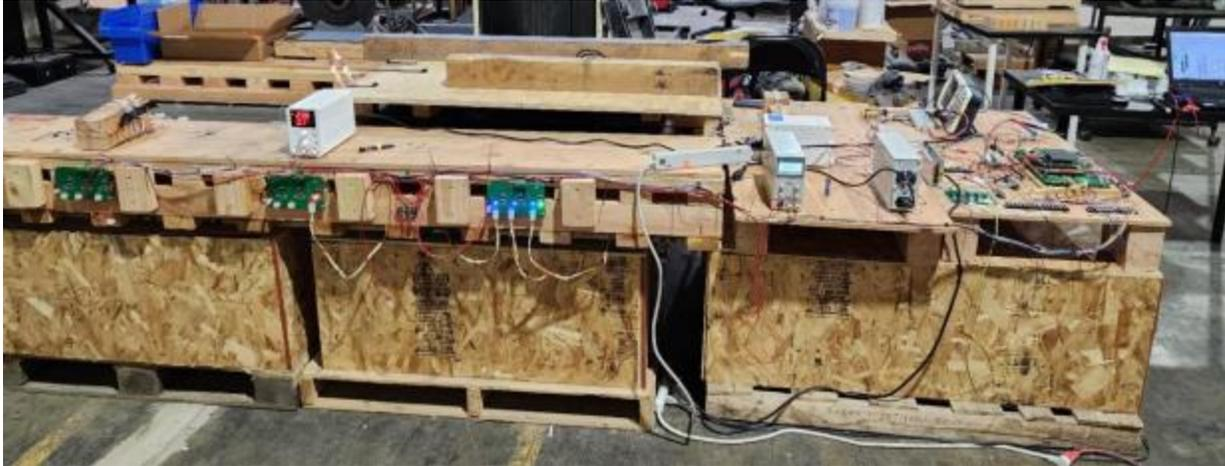
*Figure 3.54 Static subscale system setup with 4 transmitters and 30 Volt power supplies*
