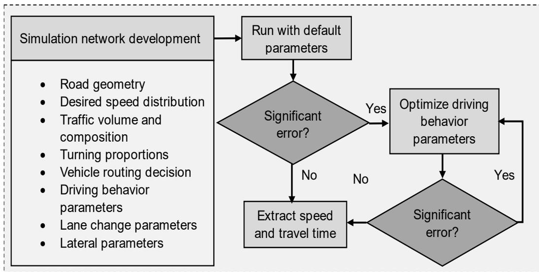
Figure 3. Simulation calibration methodology
