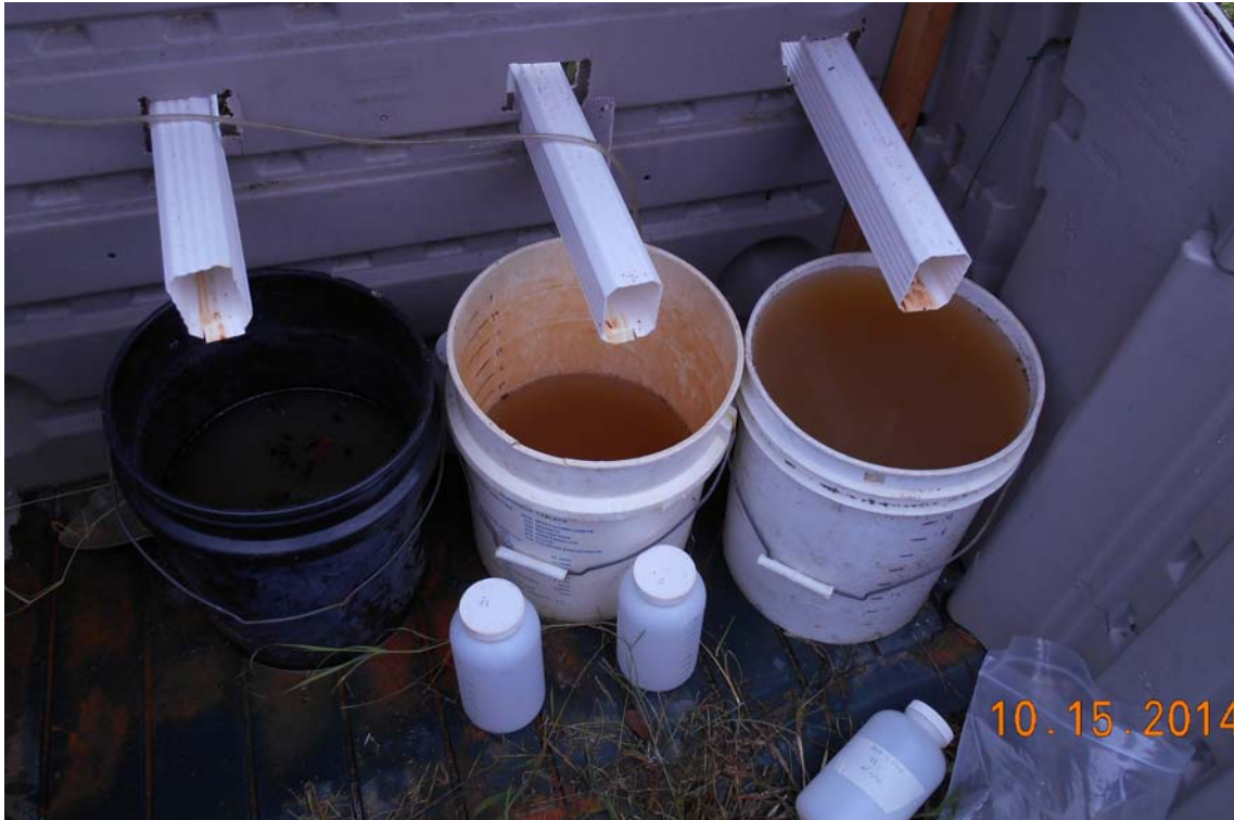
Figure 7. Buckets of runoff following 10/14/2014 storm.
