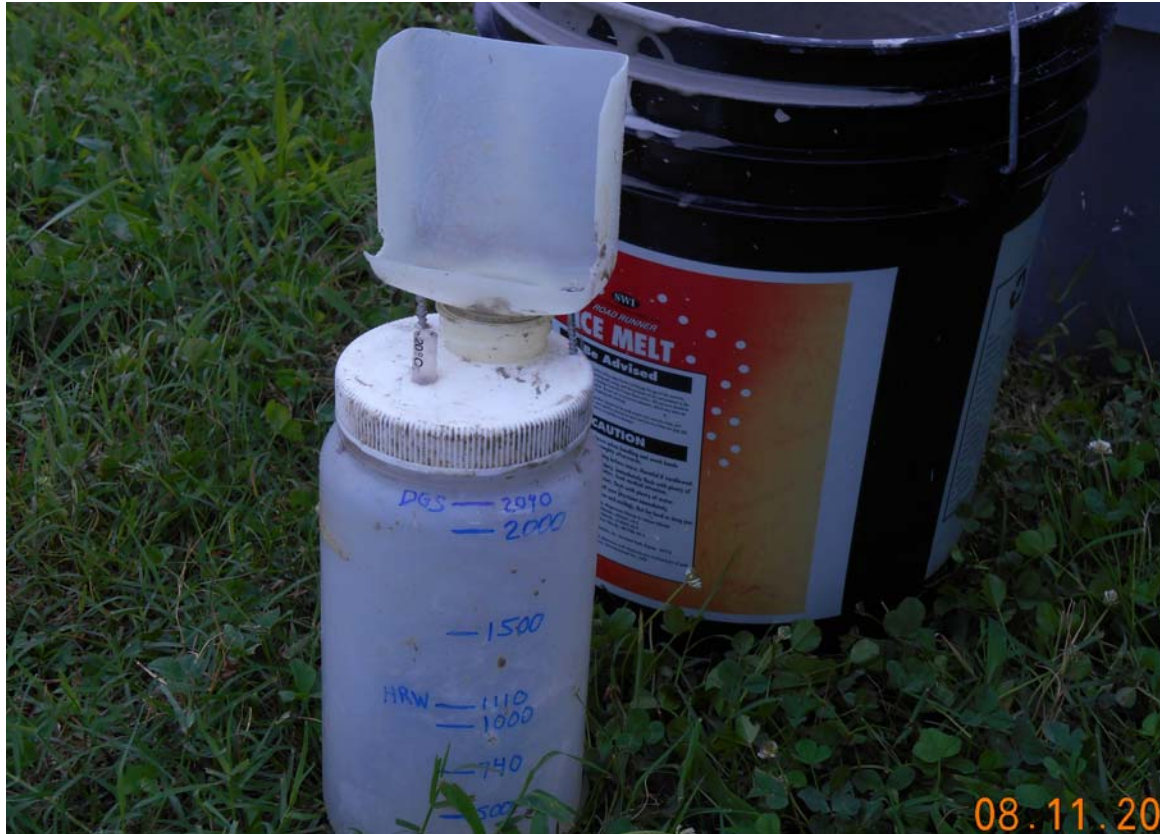
Figure 5. Application device for DGS and HRW.
