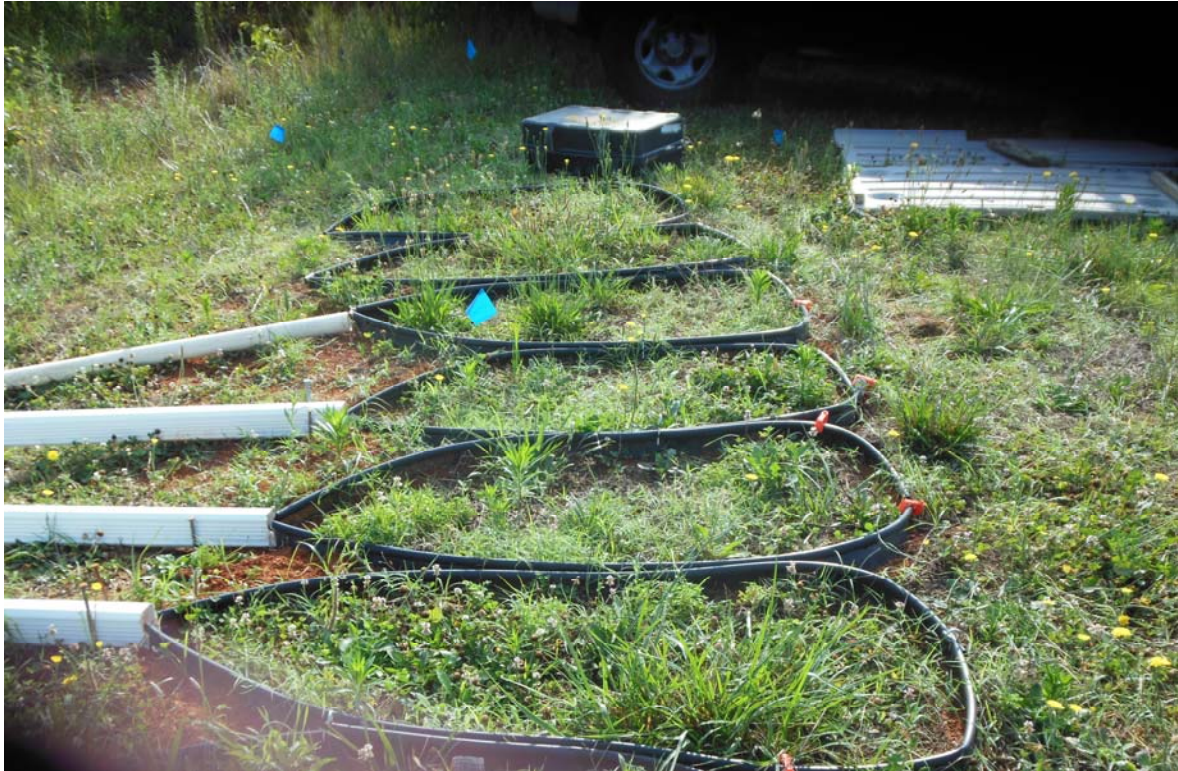
Figure 4. Runoff conveyance system for plots at the field trial.
