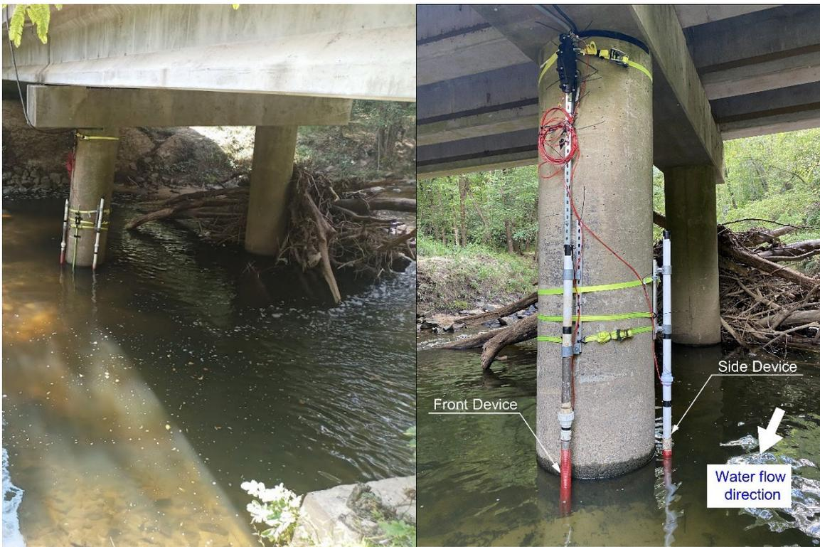
**Figure 10:** The used FO-DTS scour-monitoring devices and how they were secured to the bridge pier.
