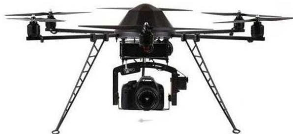
DUML flew two UAS over the Gallants Channel Bridge, each was a Ready to Fly (RTF) kit instead of an integrated UAS product from a major manufacturer. The Mikrokopter Hexa XL and Freely Cinestar 6 are carbon frame aircraft with a lifting capacity 3.3 and 5.8 lbs respectively. Both use Mikrokopter control electronics that allow for autonomous flight by pre-programmed Points of Interest (POI), GPS and
