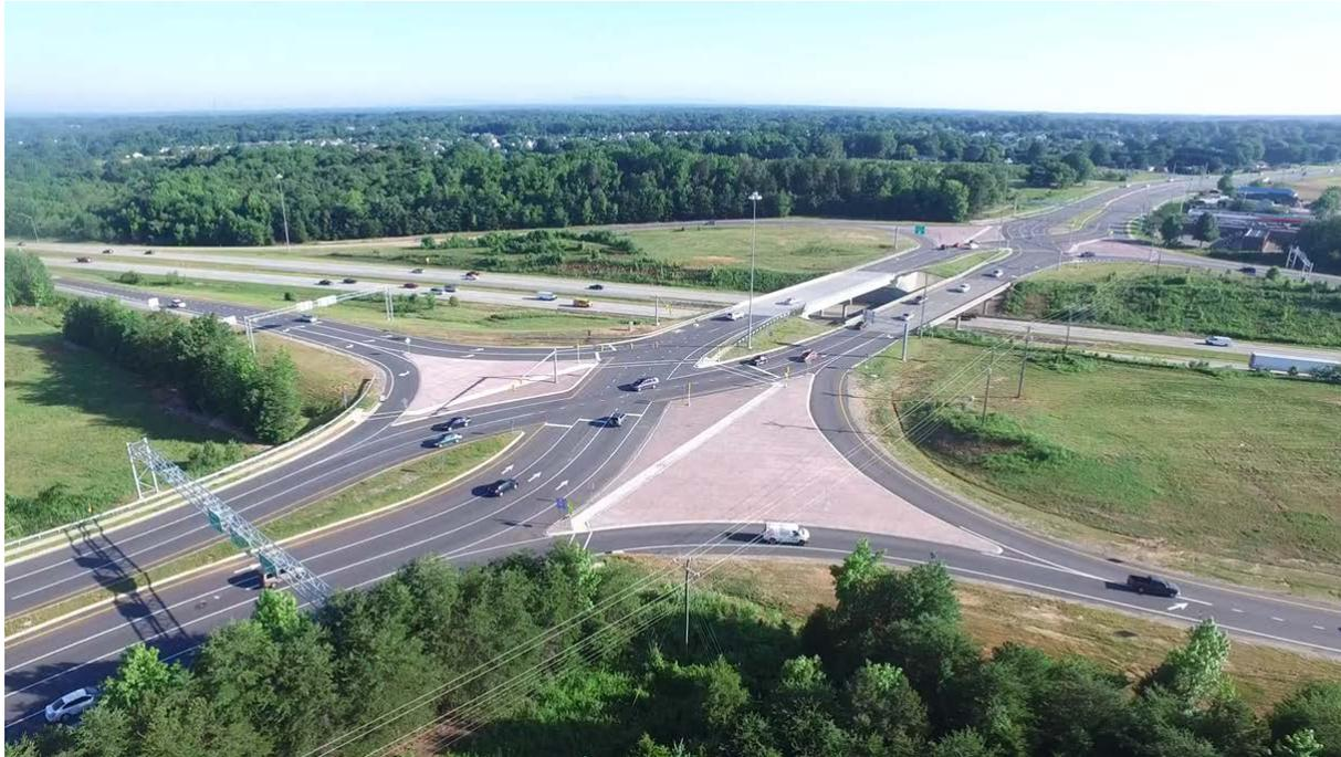
*Figure 23: Diverging Diamond Interchange Image from UAS Video*
