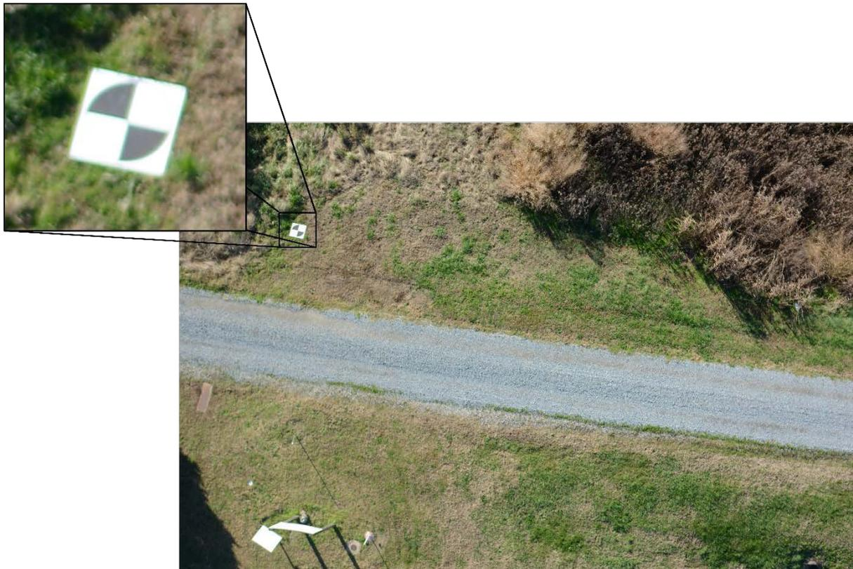
Figure 28: GCP from 67 feet flight with GSD 0.589 cm/pixel
