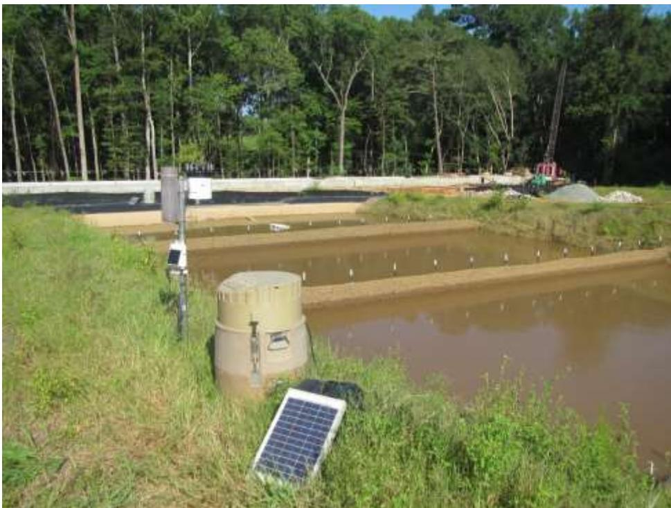
**Figure 3.4.** Picture of Basin 4 showing the samplers and rain gauges.
