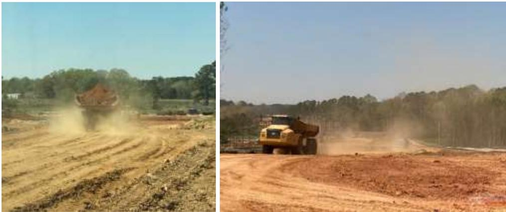
**Figure 1.0.** Examples of dump trucks generating dust on a haul road.
