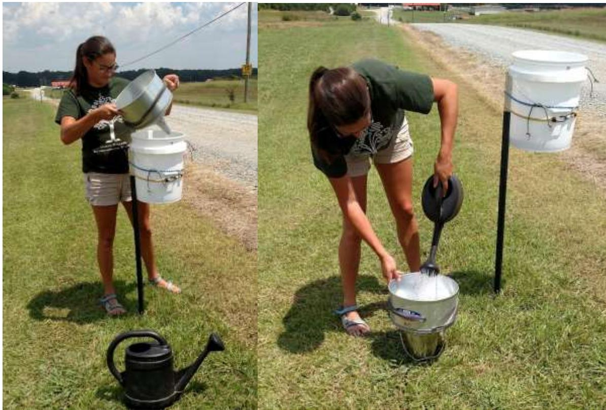
**Figure 1.7** Dust collection at the Chi Road site. The funnel was removed (left) and the dust collection bucket taken out of the larger bucket. Residual dust was rinsed into the dust collection bucket and the rinsate was poured into a sample bottle for filtering and weighing in the lab. The timing of sampling varied by location and date (Table 1.0).
