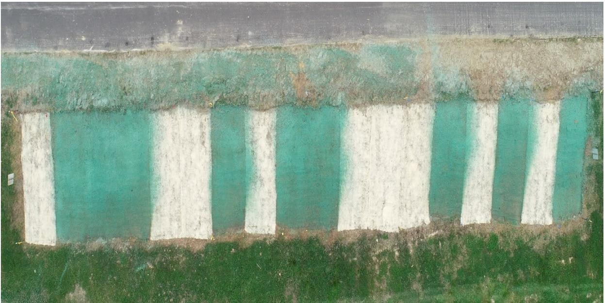
**Figure 38.** Drone image at plot establishment (16 April, 2021). The green strips are the hydromulch plots (actual color of the hydromulch).
