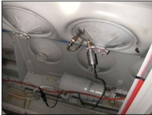
(c) Manifold Absolute Pressure And Temperature Sensor
