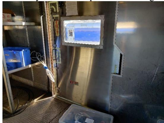
(c) PEMS exhaust outlet hoses and zero air inlet hoses exiting the baggage car
