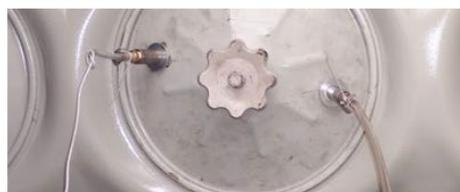
(e) Air box pressure and temperature sensors
