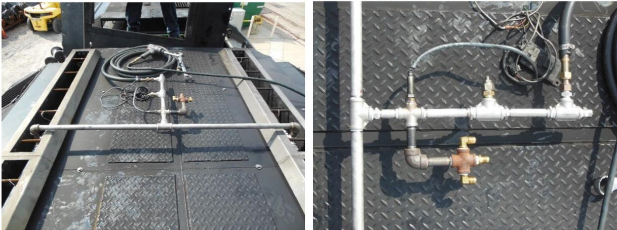
Figure 5-4. Configuration of previously installed blended after-treatment system (BATS) exhaust channels on locomotive NC 1859 (Frey and Rastogi, 2018). NCDOT has fabricated a “sampling rake” that collects exhaust from both channels with ports and fittings for multiple PEMS sample lines. The channel dimensions and sampling geometry may differ in the proposed study.
