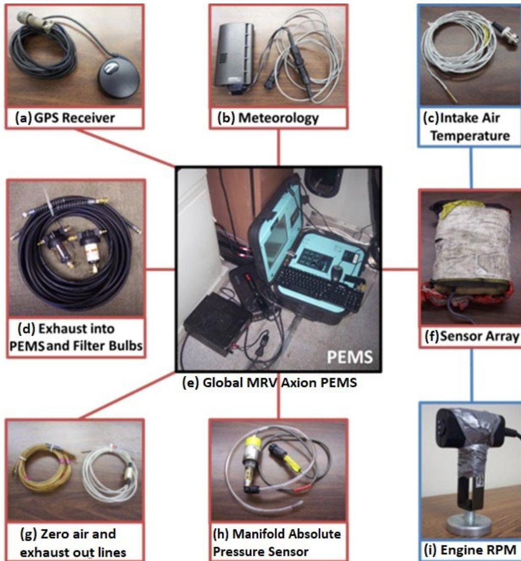
**Figure A-2. The Global MRV Axion PEMS And Components: (a) GPS Receiver; (b) Meteorology Sensor; (c) Intake Air Temperature Sensor; (d) Exhaust Sample Lines; (e) Axion PEMS; (f) Engine Sensor Array; (g) Zero Air And Exhaust-Out Lines; (h) Manifold Absolute Pressure Sensor; and (i) Engine Revolutions Per Minute Sensor.**
