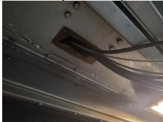
(b) Exhaust hoses and sensor array cables from prime mover engine entering the baggage car
