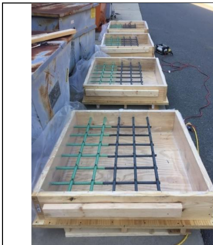
Figure 5.6a: Slab mockup forms
