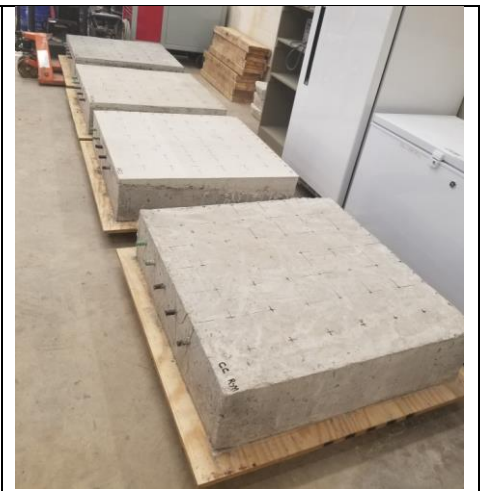
Figure 5.6c: Mockups with overlay slabs placed (rear three mockups)
