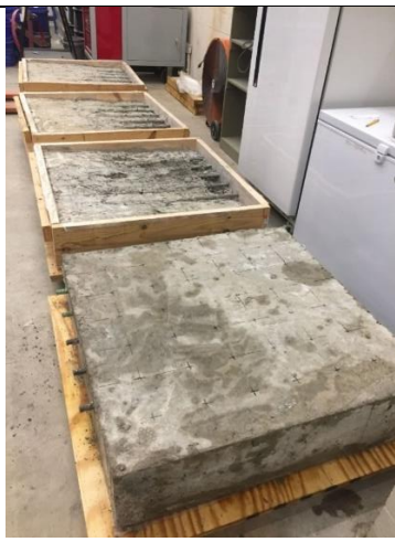
Figure 5.6b: Mockups after AA deck slab was placed, but prior to overlay placement
