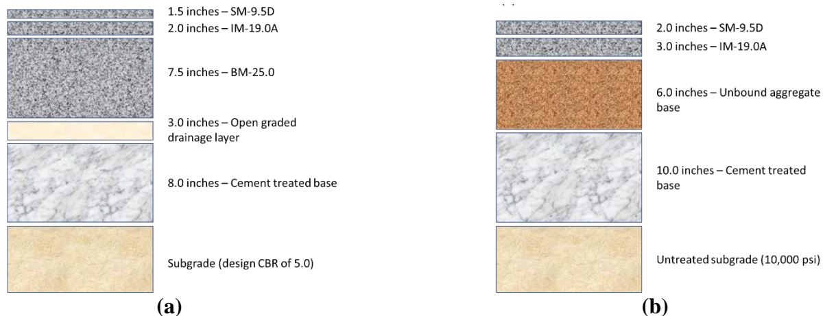
Figure A.15. (a) Conventional pavement section, (b) Inverted pavement section from Bull Run, Virginia [Weingart 2010].
