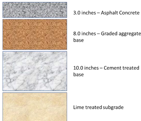
Figure A.13. I-25 New Mexico inverted pavement design for I-25 study.
