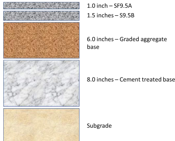
Figure A.14. Pineville Quarry haul road inverted design.
