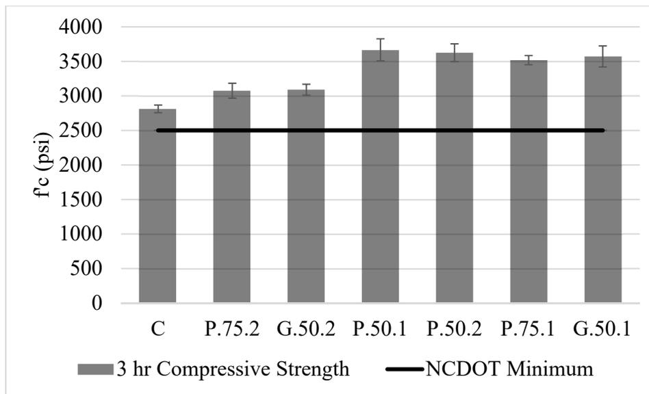
Figure 3-1: Preliminary Compressive Strength with Uncontrolled Citric Acid
