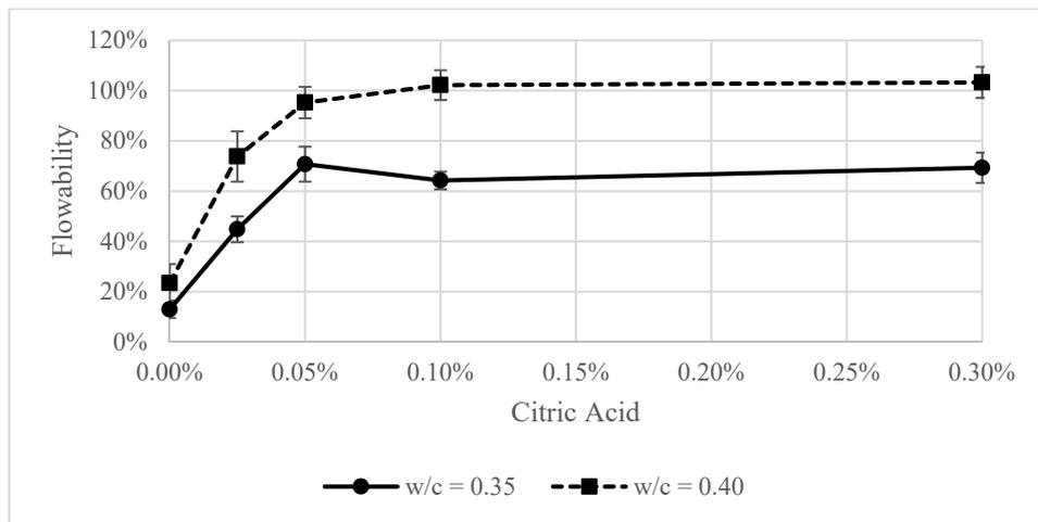
Figure 4-4: Average Flowability vs Citric Acid at 6 Minutes.
