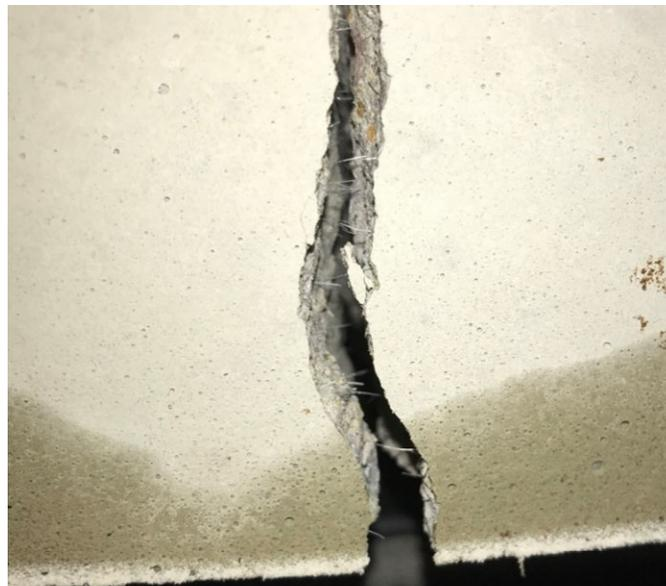
Figure 3-10: P.50.1 Crack Bridging and PVA Fiber Pullout.
