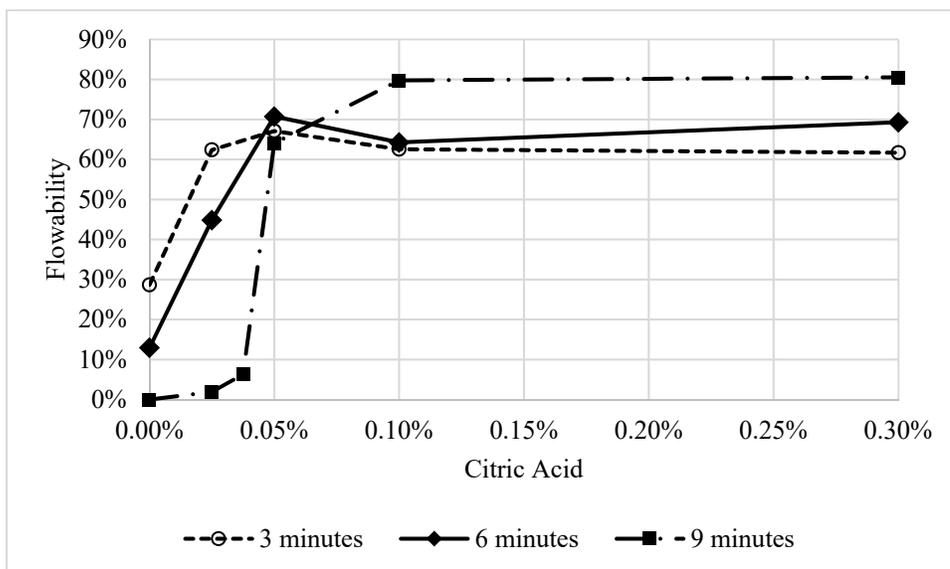
Figure 4-1: Flowability vs Citric Acid Content at w/c=0.35.
