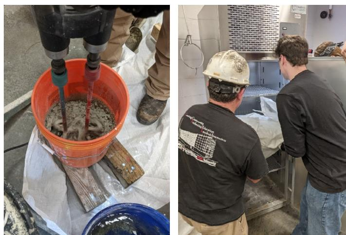
Figure 5-10: Mixing (left) and Curing (right) Specimens for Temperature-Effect Testing.
