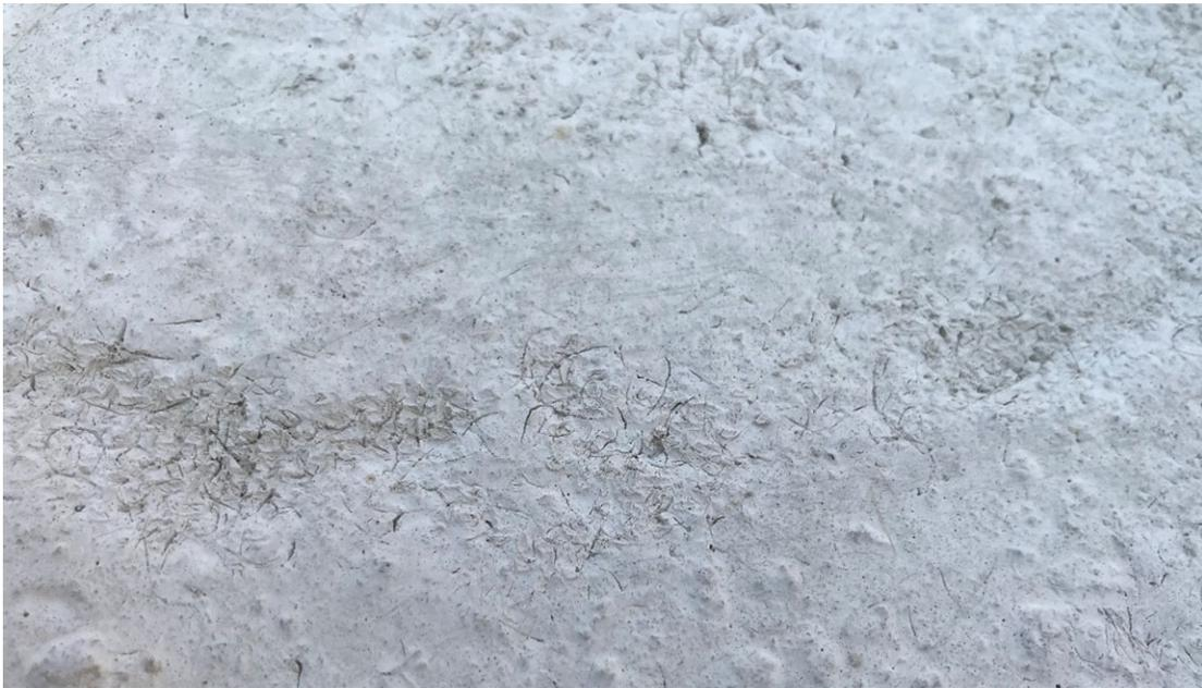
Figure 5-13: Very Minor Surface Cracking in CA Specimens.
