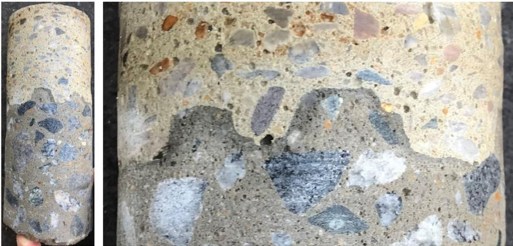
Figure 5-17: G.50.2 3-inch Slab Core (overlay material on top and OPC slab on bottom).
