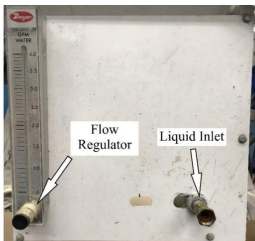
Figure B-3: Liquid Control Panel.
