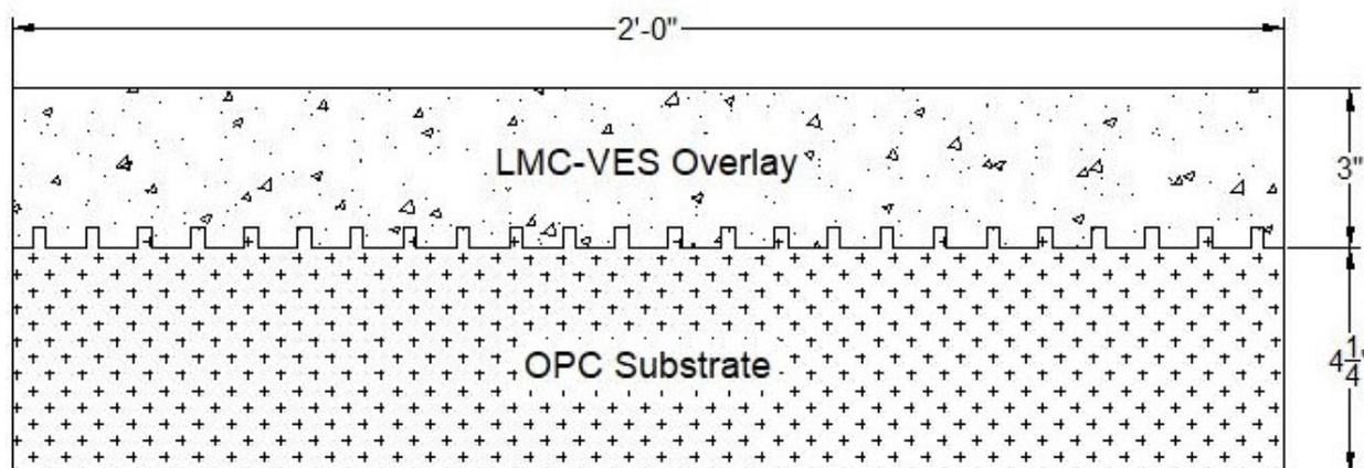
Figure 5-1: 3" Overlay Slab Cross Section.
