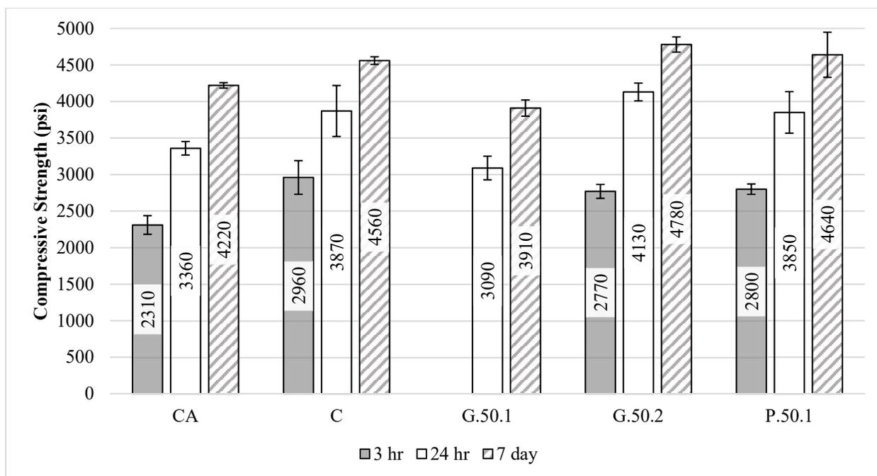
Figure 3-3: Second Set of Compressive Strength Results.
