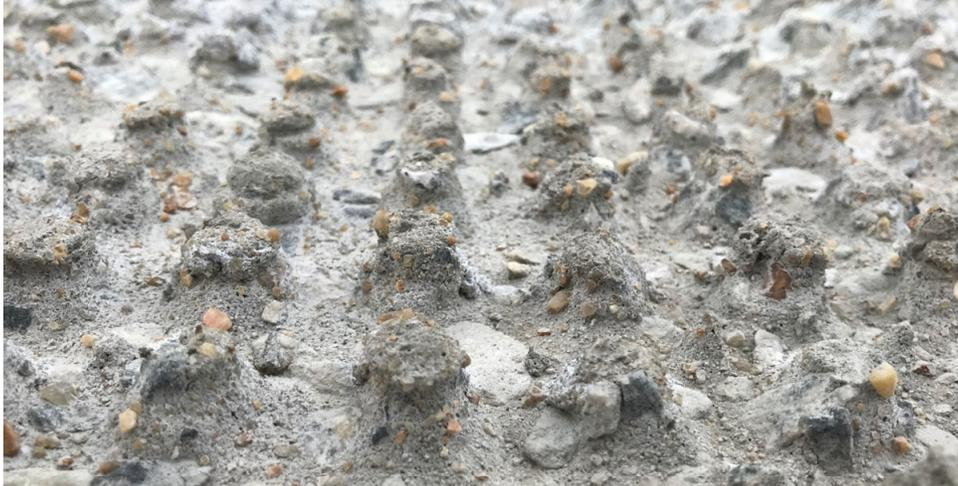
Figure 5-6: Final Base Slab Roughened Surface in the Laboratory.
