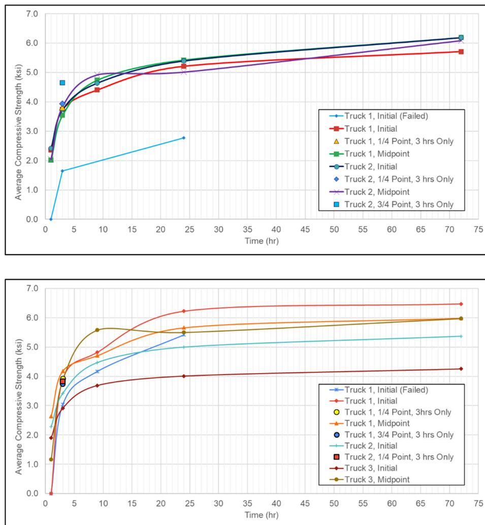
Figure 6-13 (a) and (b): Compressive Strength Results for Lane 1 (above) and Lane 2 (below).
