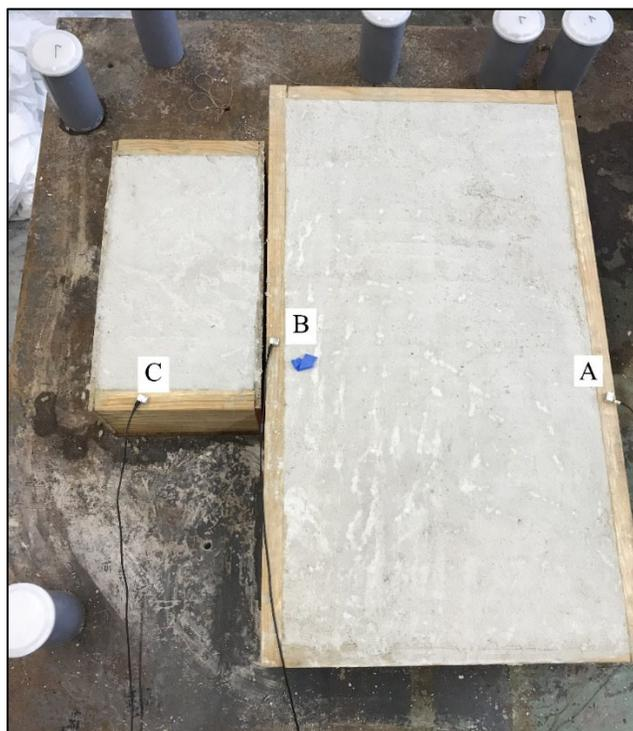
Figure 5-9: Accelerometer Placement.
