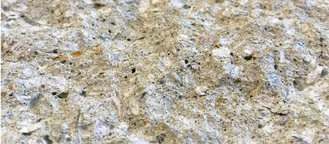
Figure 3-9: G.50.1 Flexural Failure Surface.
