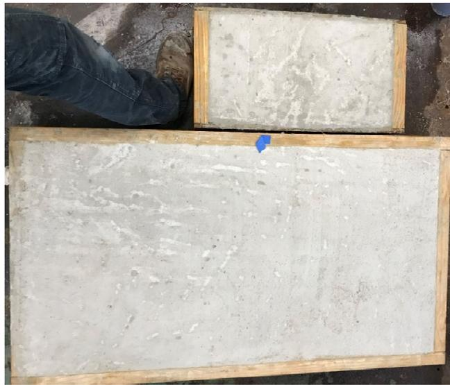
Figure 5-11: C Vibrated Specimen Surface at 3 Hours (no cracks).
