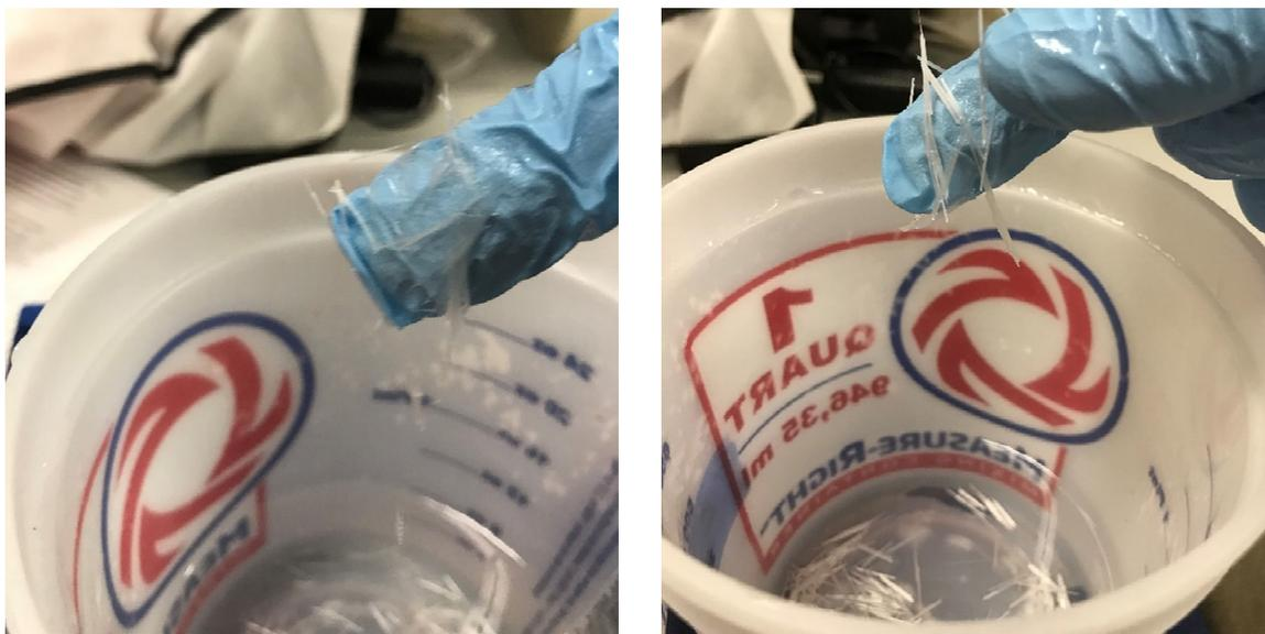
Figure 6-9: Dispersion after 5 Minutes in Water for Lab Fibers (left) and Field Fibers (right)
