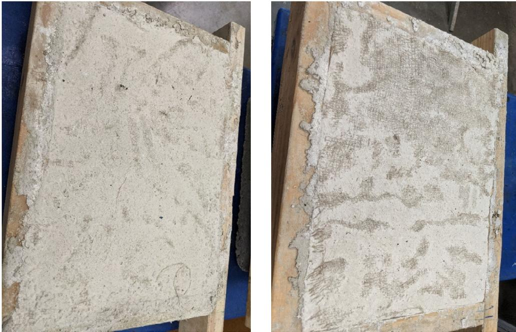
Figure 5-20: High Citric Acid Specimens at 3" (left) and 1" (right) in Depth.
