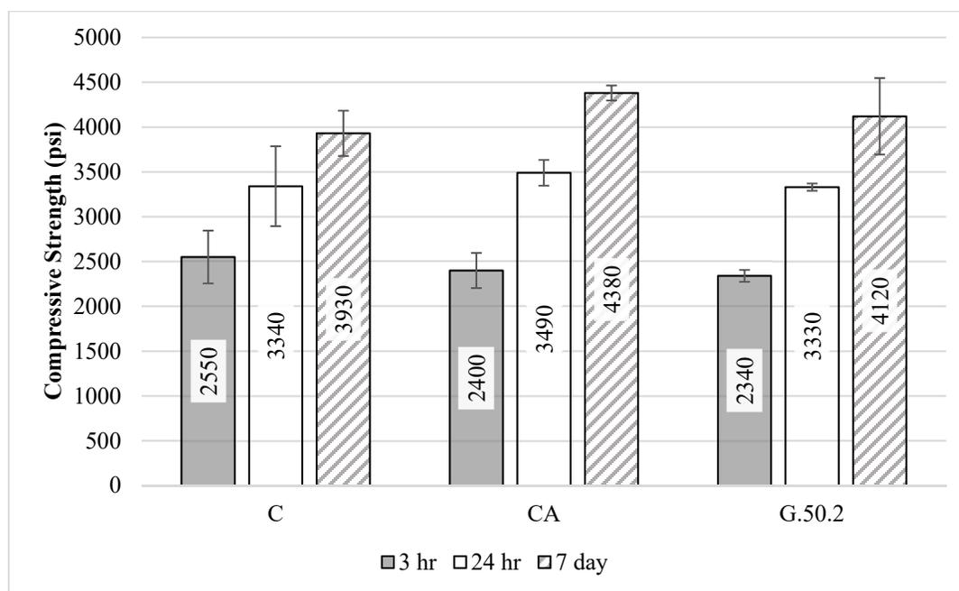
Figure 3-4: Third Set of Compressive Strength Results.
