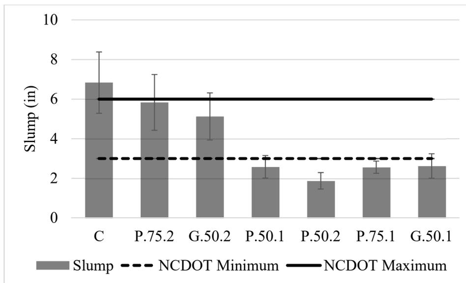
Figure 3-2: Preliminary Slump Results with Uncontrolled Citric Acid
