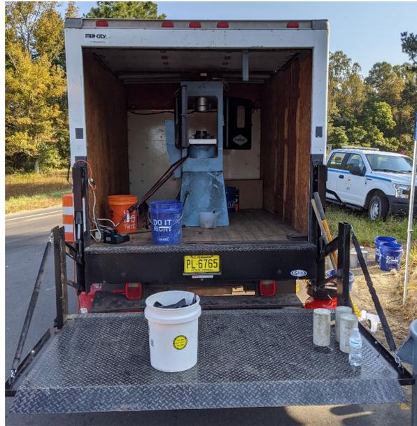
Figure 6-11: Compression Testing Equipment (in a Truck) on the Field Trial.
