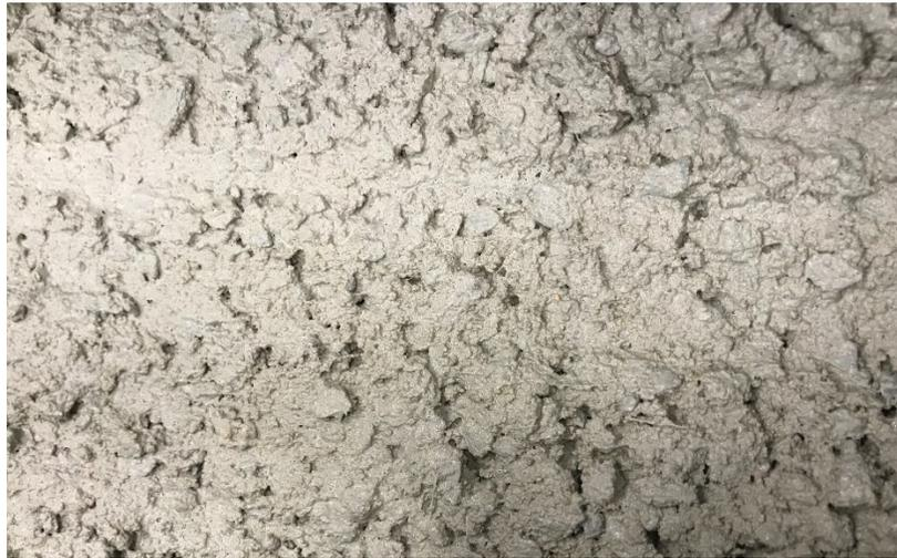
Figure B-10: Fully Mixed Concrete.
