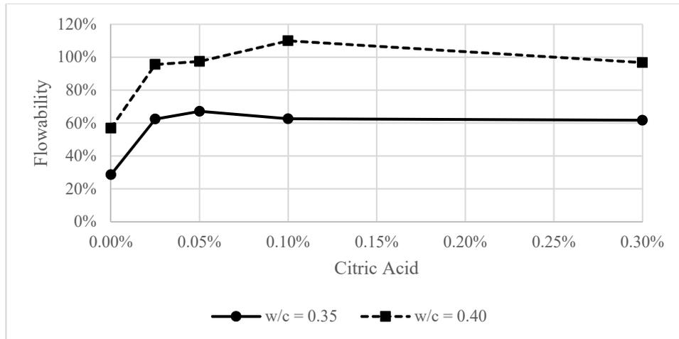
Figure 4-3: Flowability vs Citric Acid at 3 Minutes.
