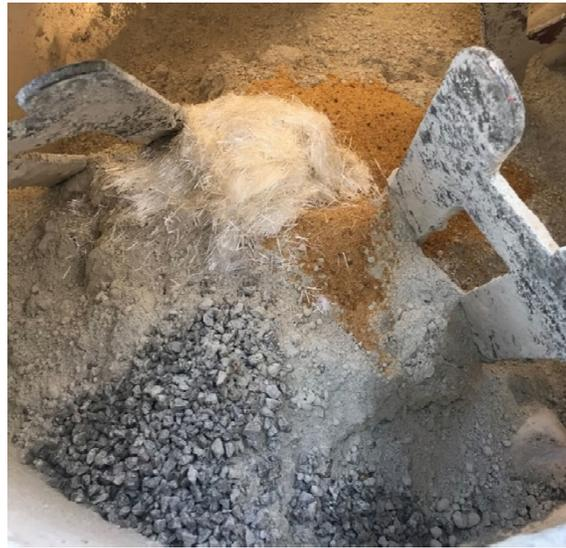
Figure B-6: Dry Materials in Drum Mixer before Dry Mixing.
