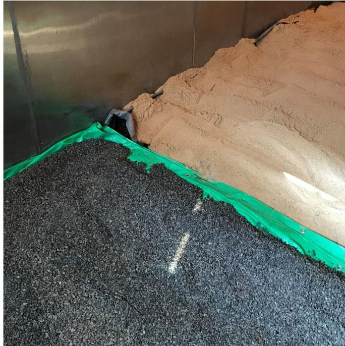
Figure B-5: Drying Aggregates by Evaporation in a Large Environmental Chamber.
