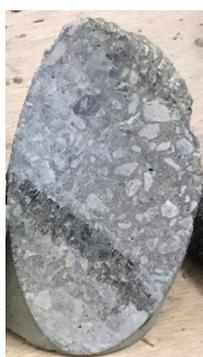
Figure 3-6: Typical sawed surface with minor defects such as a tapered edge.
