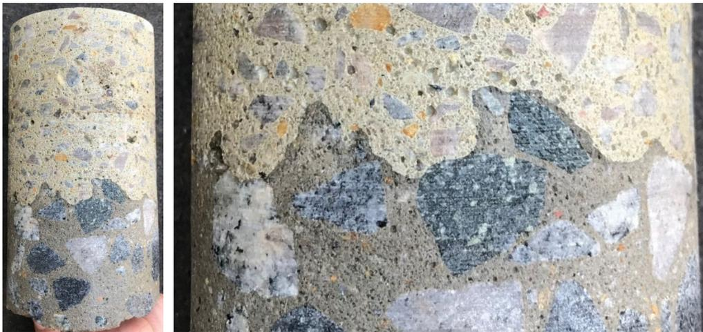
Figure 5-12: C 3-inch Slab Core (Overlay on top, OPC base slab on bottom).
