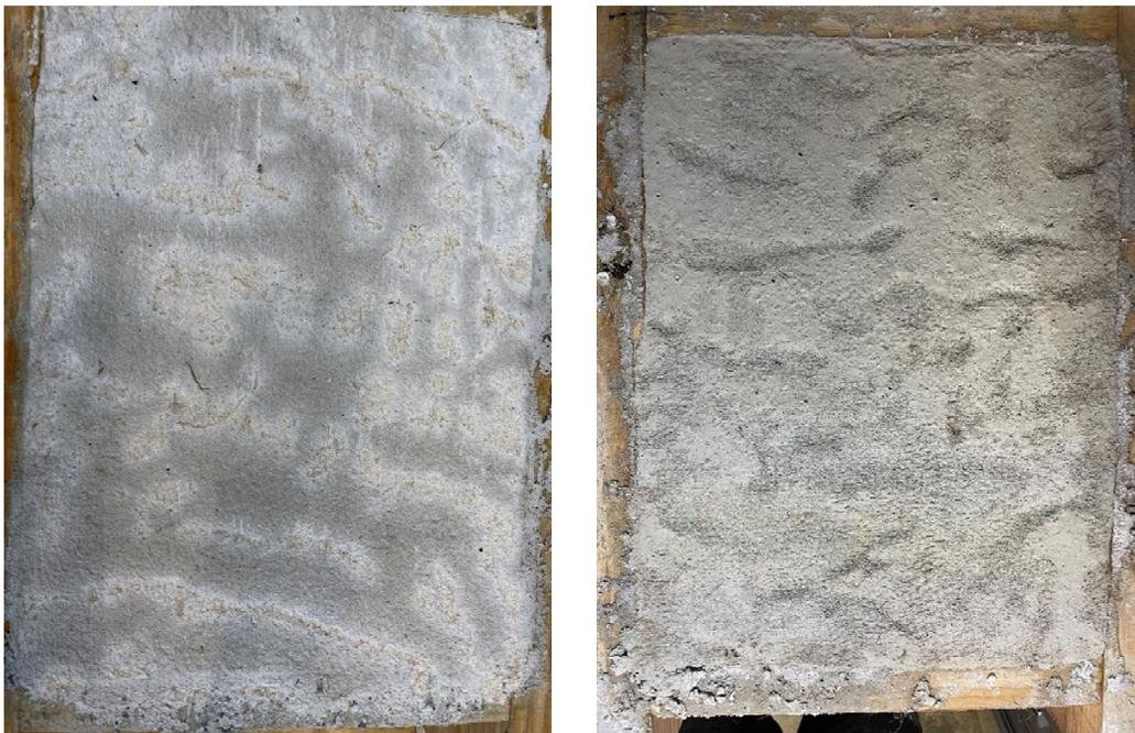
Figure 5-19: CA Citric Acid Specimens at 3" (left) and 1" (right).
