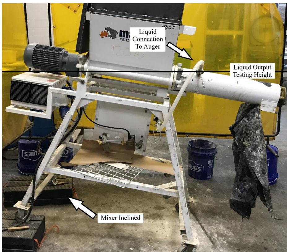
Figure B-8: Inclined Continuous Mixer.
