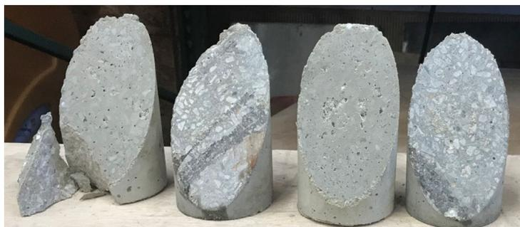
Figure 3-7: Shear Bond Failure (left pair) and Combination Failure (right pair).
