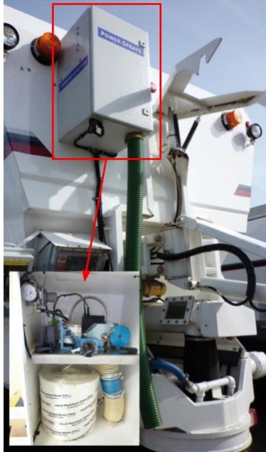
Figure A-1: Spooled Fiber Feeder.
