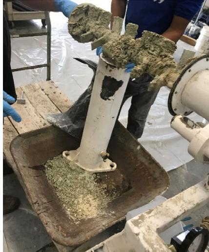
Figure B-11: Cleaning Auger.
