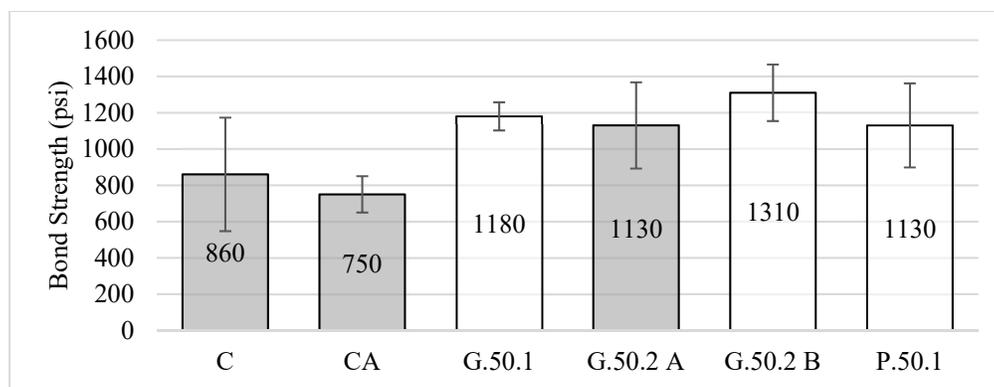
Figure 3-5: Slant Shear Bond Strength.
