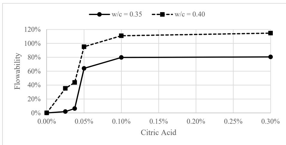
Figure 4-5: Flowability vs Citric Acid at 9 Minutes.
