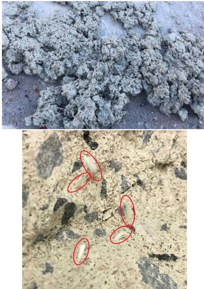
Figure 6-8: Poor Fiber Dispersion in Fresh (top) and Hardened (bottom) Concrete.
