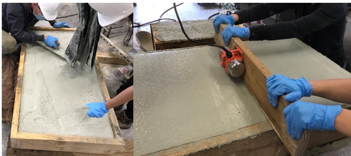
Figure 5-8: Casting and Finishing Laboratory Overlay Slabs.
