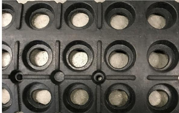
Figure 5-3: Rubber for Roughening Slab Surfaces.
