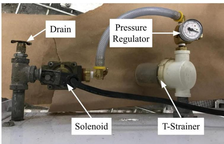
Figure B-4: Liquid System (Behind Liquid Control Panel).
