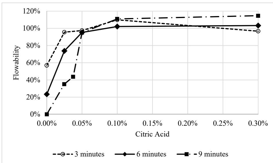
Figure 4-2: Flowability vs Citric Acid Content at w/c=0.40.
