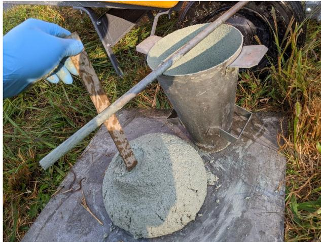
Figure 6-12: Typical Slump Test at the Field Trial
