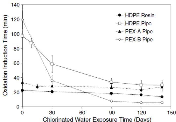
Figure 2. Change in oxidation induction time for HDPE resin, HDPE pipe, PEX-A pipe and PEX-B pipe during accelerated aging in 45 mg/L as Cl<sub>2</sub>, 50 mg/L as CaCO<sub>3</sub> at 37° C (after, Whelton et al. 2011).
