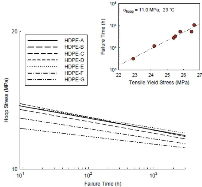
Figure 2. Pipe hoop stress versus failure time data for all subject HDPE pipes at 23°C. At least 15 failure data points were fitted to produce the best-fit lines shown in the plot. The inset shows failure time for an applied hoop stress of 11.0 MPa plotted as a function of the tensile yield stress of the polymer (after Krishnaswami 2005)
