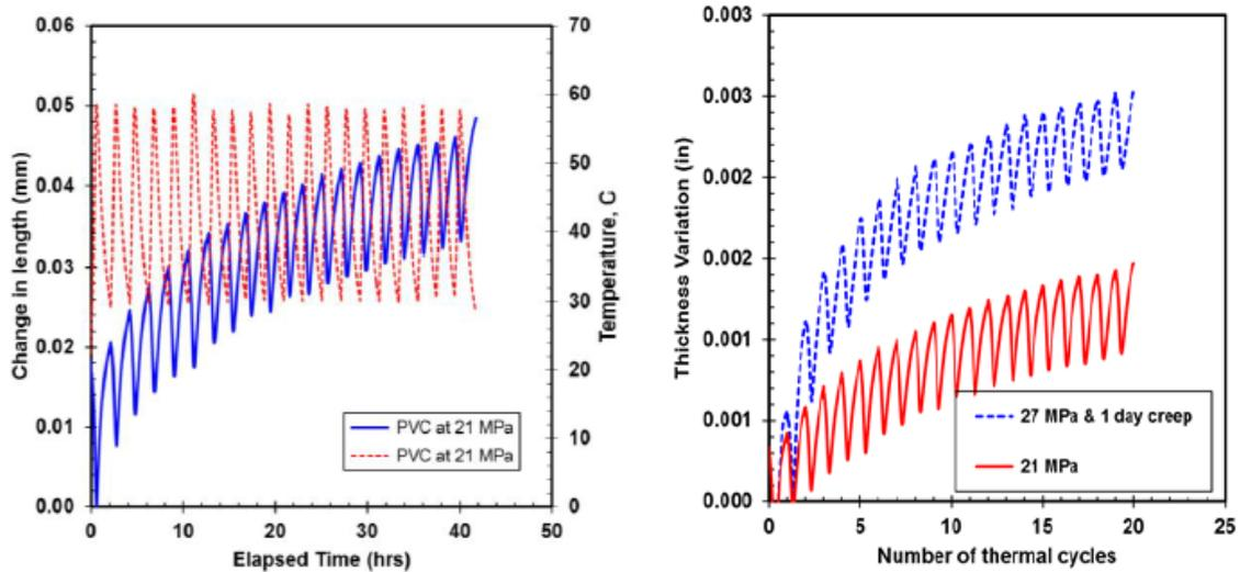
Figure 6. Change in length under thermal ratcheting of a (a) PVC with 1 day creep at 21 MPa (b) HDPE with and without 1 day creep at 14 Mpa (after Jeya et al. 2017)
