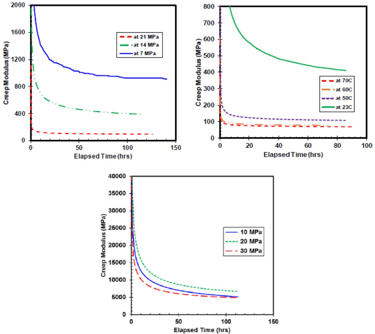
Figure 5. Creep modulus (a) HDPE under different loads at room temperature, (b) DDPE under 14 MPa at different temperature, (c) PVC under different loads at 45°C (after Jeya et al. 2017)
