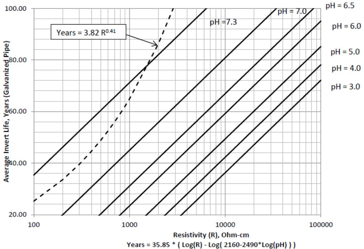
Figure 10. Average invert life (years) for 16 Gage galvanized steel pipe
