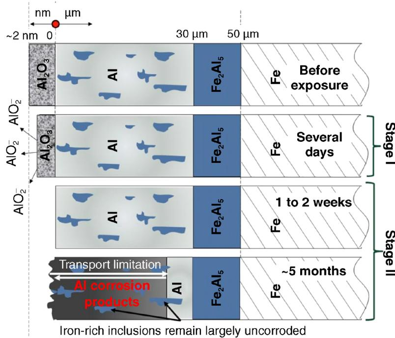
Figure 35. Mechanism of aluminized Type 2 steel corrosion in limestone-saturated flowing water condition (Akhoondan and Sagüés, 2013)
