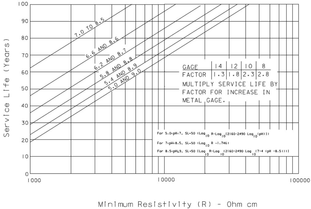
Figure 6. Estimated service life versus pH and resistivity for aluminized Type 2 pipe using FDOT method (courtesy of FDOT)
