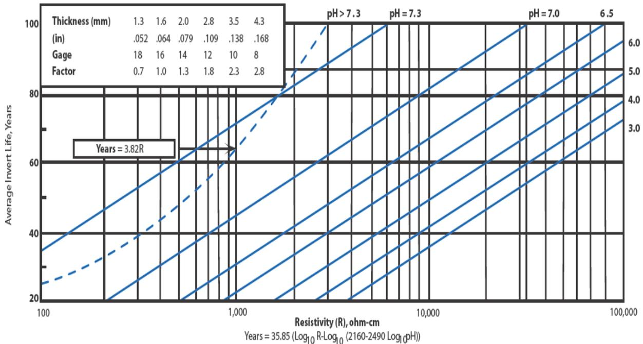
Figure 5. AISI chart for estimating average invert life for galvanized CSP (Courtesy of AISI)
