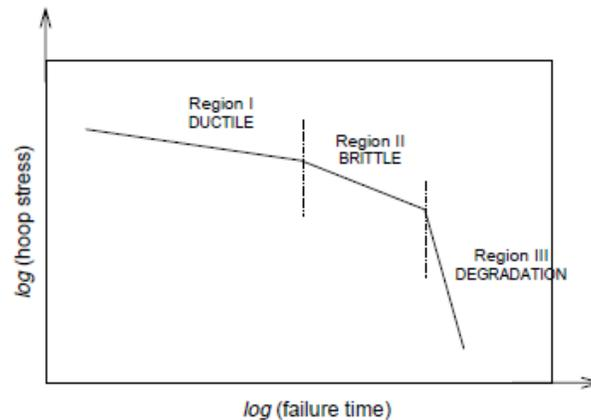
Figure 1. Schematic of the typical hoop stress versus failure time plot for polyethylene pipe (after Krishnaswami 2005)
