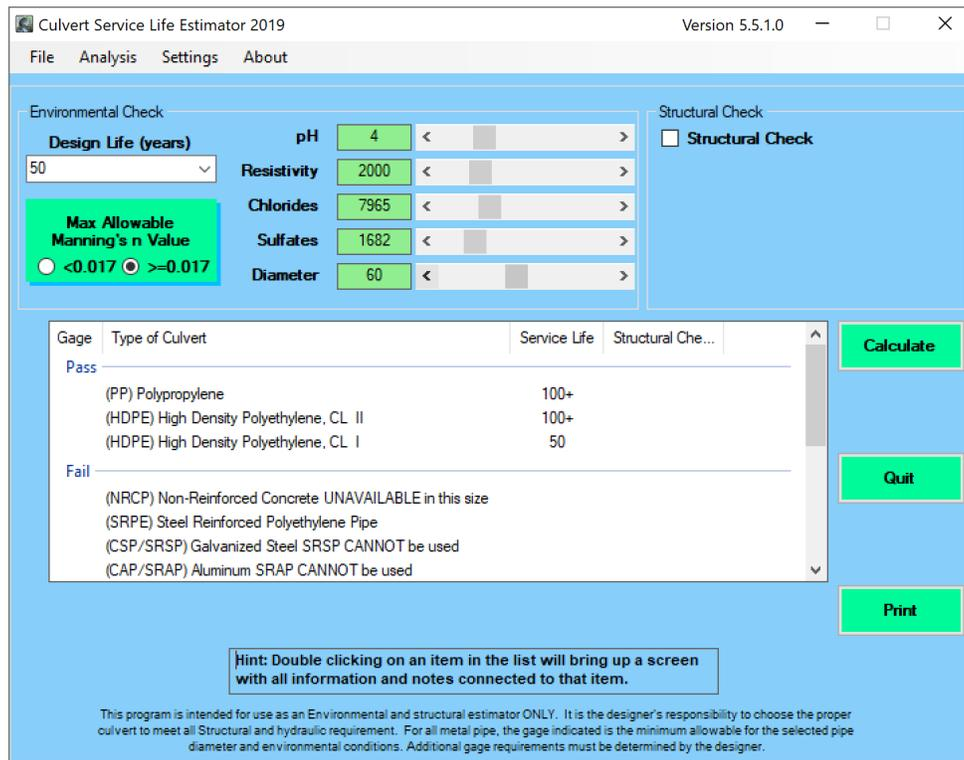
Figure 9. FDOT culvert service life estimator 2019 (Courtesy of FDOT)
