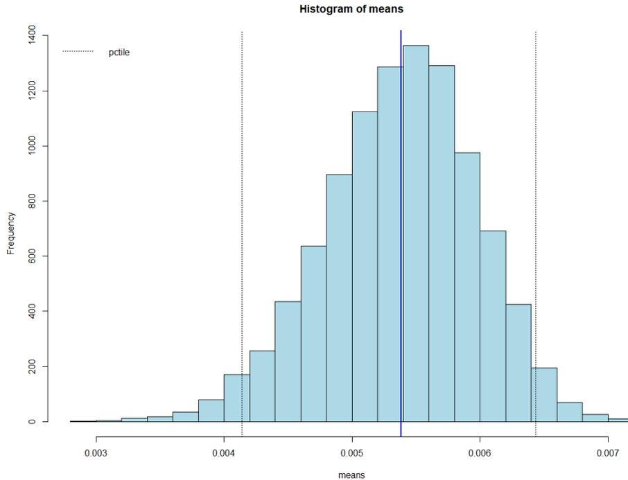
Figure 33. Bootstrap result of the corrosion rate of aluminized pipe samples
