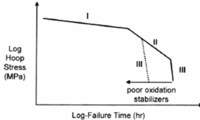
Figure 36. A lack of antioxidants will shift stage III failures to the left, potentially limiting the service life (after Pluimer, 2011)
