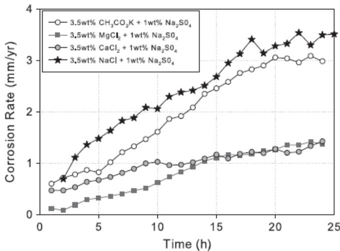
Figure 38. 24 h Linear Polarization Resistance measurements for galvanized steel samples immersed in solutions containing 3.5 wt.% of NaCl, MgCl<sub>2</sub>, CaCl<sub>2</sub>, and CH<sub>3</sub>CO<sub>2</sub>K with 1 wt.% Na<sub>2</sub>SO<sub>4</sub> added at 25°C (after Padilla et al., 2013)
