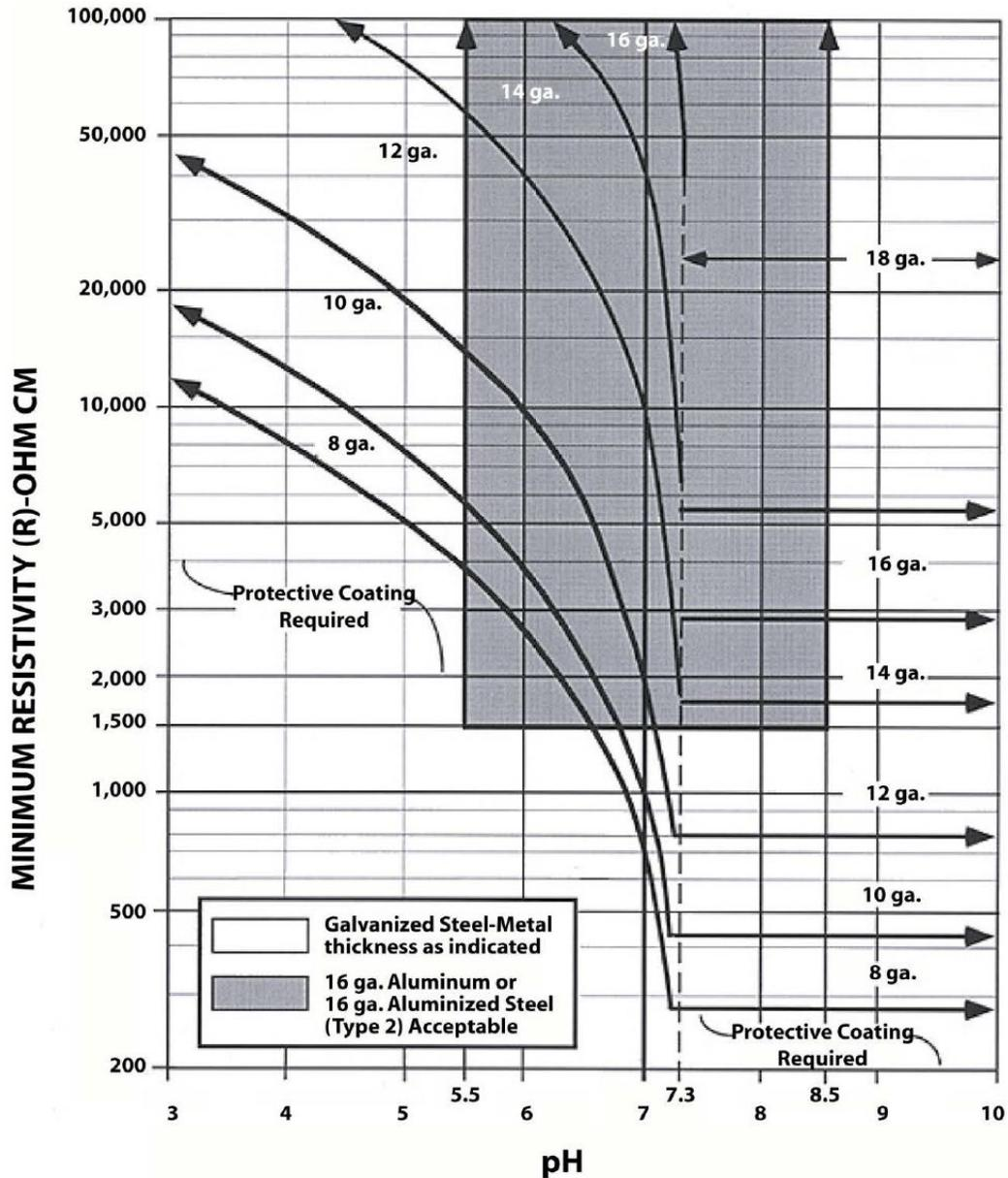
Figure 4. Minimum thickness of metal pipe for 50-year maintenance-free service life
