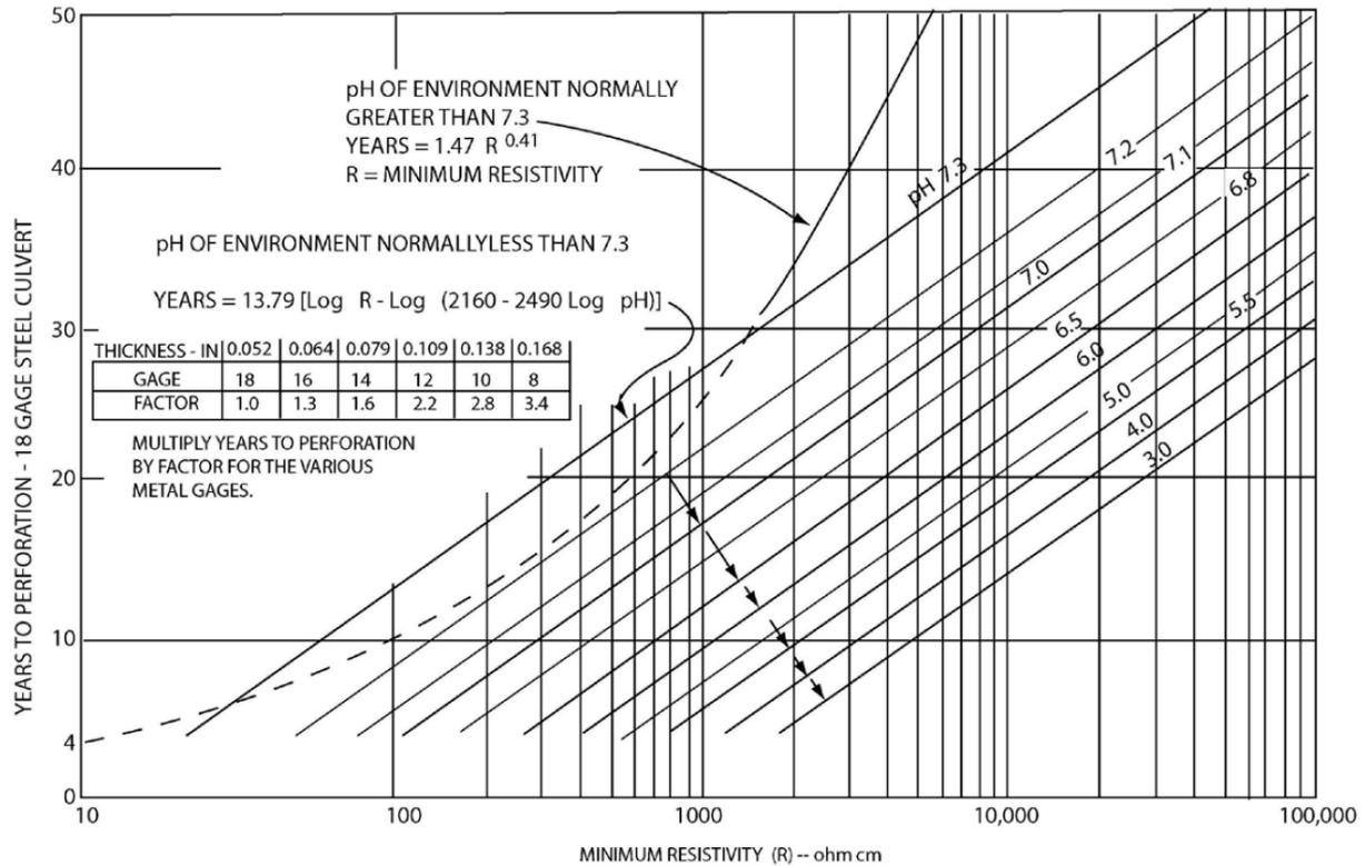
Figure 3. Chart for Estimating Years to Perforation of Steel Culverts
