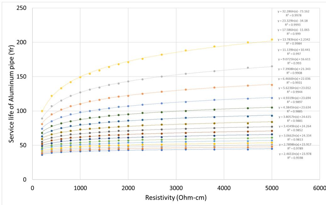
Figure 14. Plotted design service life versus pH and resistivity for 16-gage aluminum culvert pipe using FDOT method (data from FDOT)
