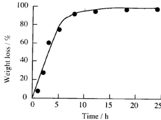
Figure 4. Weight loss curve for rigid-PVC pellet in 15 M NaOH at 250 °C and pressure of 5 MPa (after T.Yoshika et al. ,1999)
