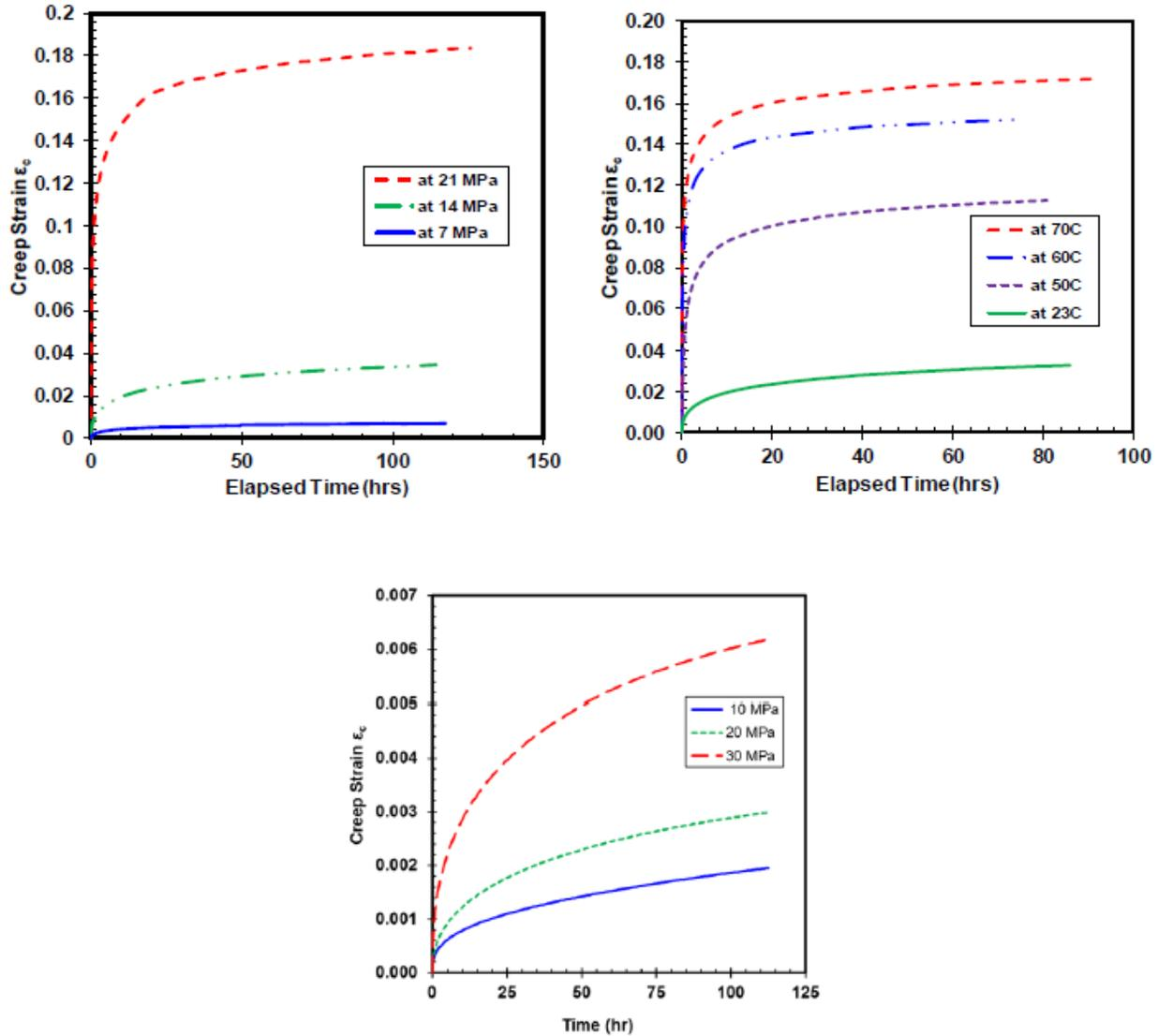
Figure 4. Creep strain (a) HDPE under different loads at room temperature, (b) DDPE under 14 MPa at different temperature, (c) PVC under different loads at 45°C (after Jeya et al. 2017).
