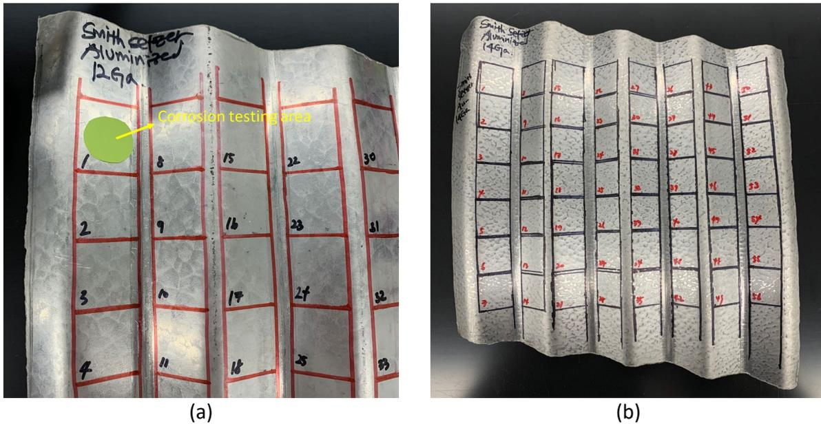
Figure 27. Grids on the surface of a pipe sample
