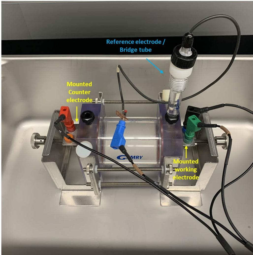
Figure 29. PDP testing set up
