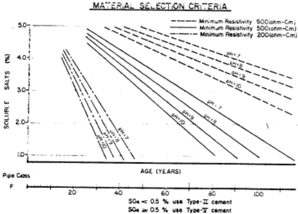
Figure 12. Material selection chart for concrete pipe (Courtesy of Utah DOT)
