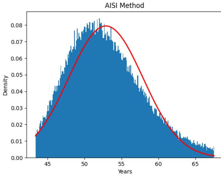
Figure 8: Service Life using AISI Method
