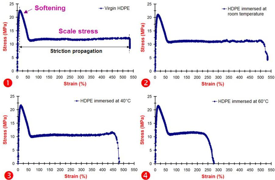
Figure 3. Effect of aging temperature on tensile curves of specimens HDPE: unaged (1), aged at 25 (2), aged at 40°C (3) and at 60°C (4) for 92 days of immersion in acid H<sub>2</sub>SO<sub>4</sub>(pH=1) (after Mouallif et al., 2011)
