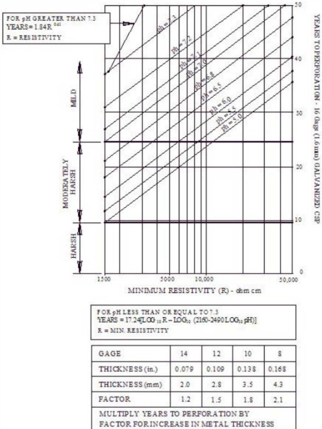
Figure 8. Chart for estimating years to perforation of galvanized corrugated steel pipe (Courtesy of Louisiana DOT)
