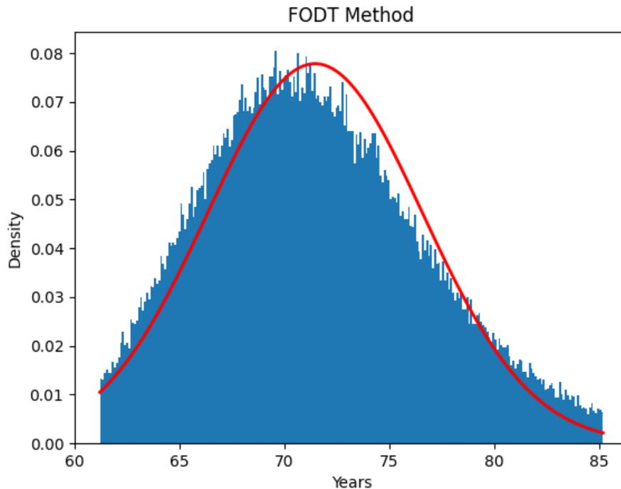
Figure 15: Service Life using FDOT Method
