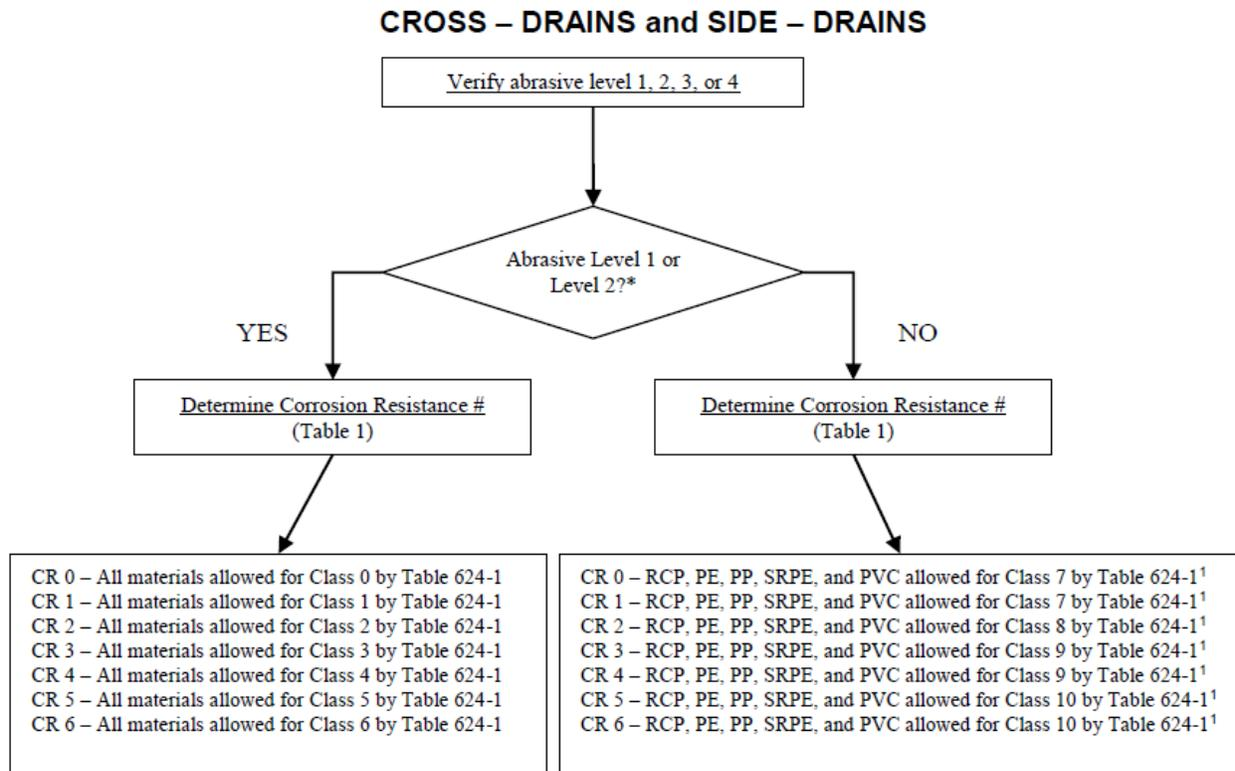
Figure 6. Diagram for selecting pipe materials (Courtesy of Colorado DOT)
