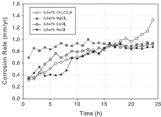
Figure 37. 24 h Linear Polarization Resistance measurements for galvanized steel samples immersed in solutions containing 3.5 wt.% of NaCl, MgCl<sub>2</sub>, CaCl<sub>2</sub>, and CH<sub>3</sub>CO<sub>2</sub>K at 25°C (after Padilla et al., 2013)
