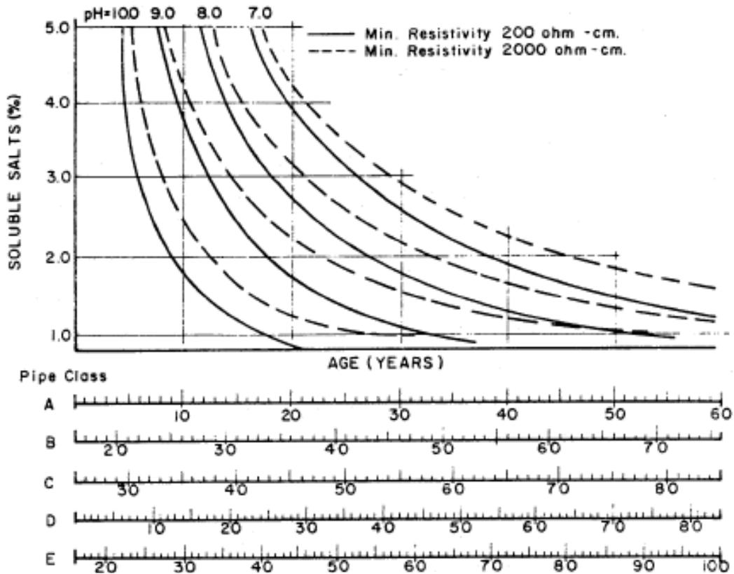
Figure 13. Material selection chart for pipe classes A through E (Courtesy of Utah DOT)
