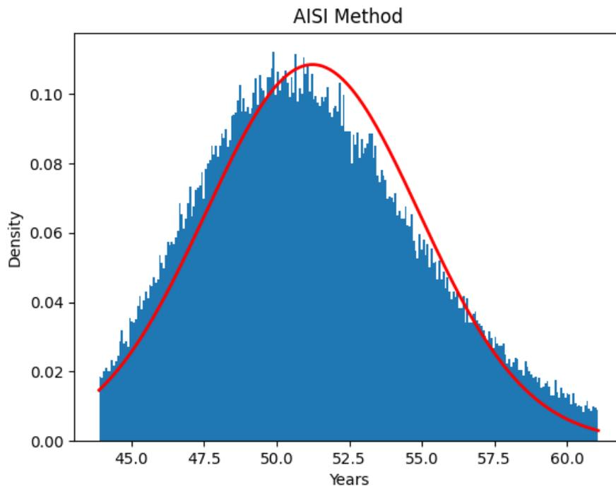
Figure 13: Service Life using AISI Method
