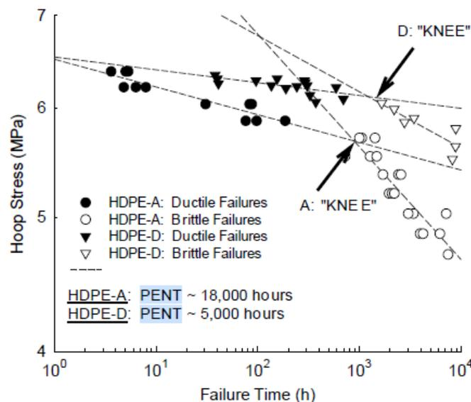
Figure 3. Pipe hoop stress versus failure time data for HDPE-A and HDPE-D at 80°C.
