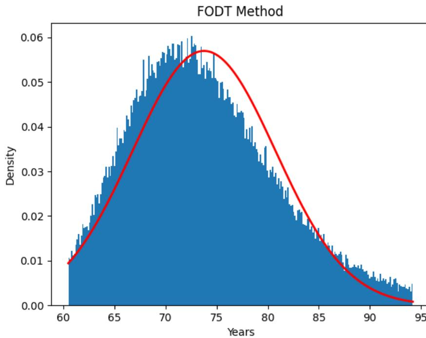
Figure 10: Service Life using FDOT Method
