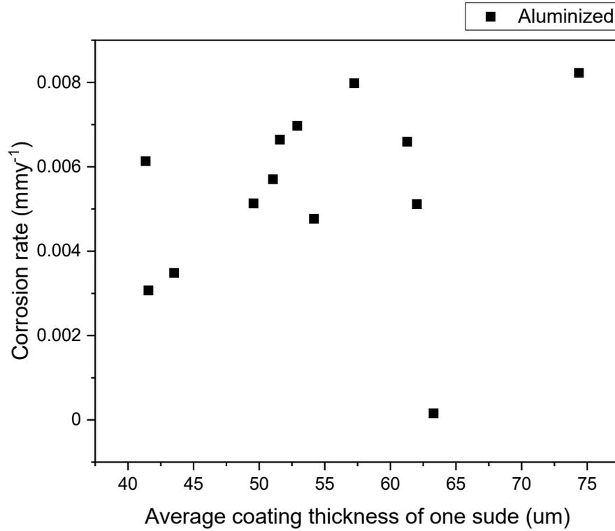
Figure 31. Corrosion rate result of aluminized pipe
