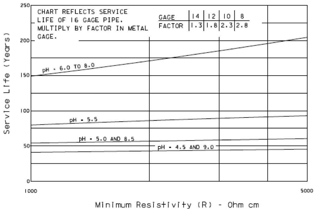
Figure 7. Estimated service life versus pH and resistivity for aluminum pipe using FDOT method (courtesy of FDOT)
