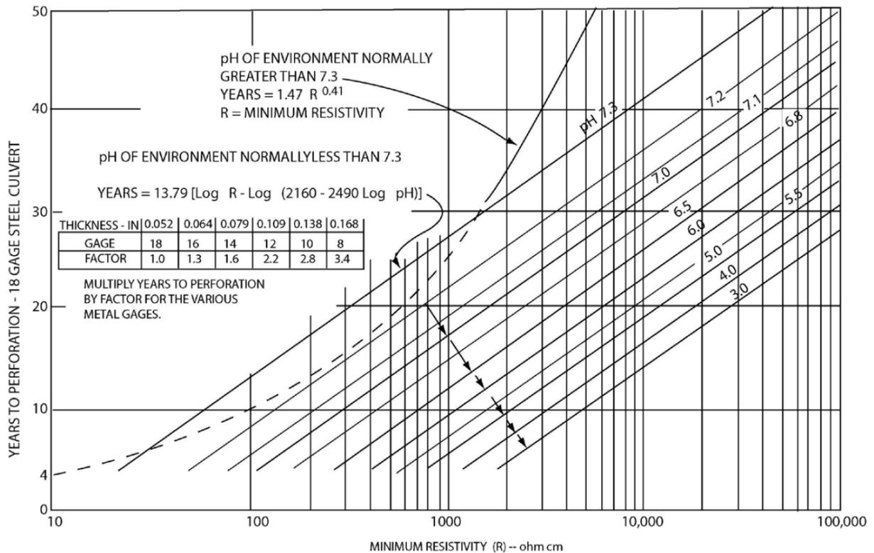
Figure 3. Chart for Estimating Years to Perforation of Steel Culverts (Courtesy of CALTRANS)
