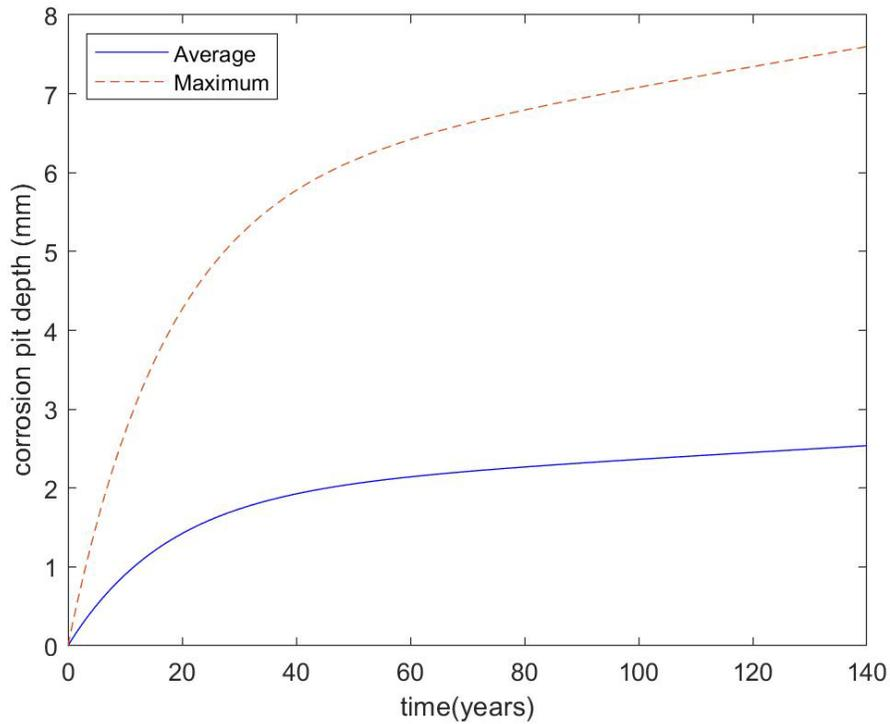
Figure 15. Corrosion pit depth of cast iron
