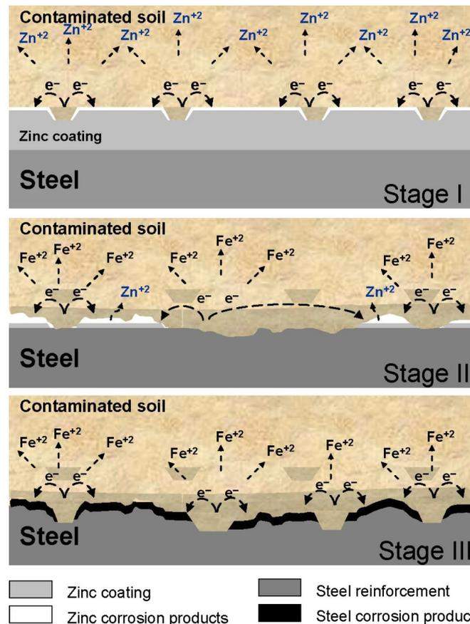
Figure 34. Three stages of galvanized steel corrosion (Padilla et al. 2013)
