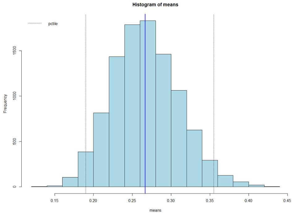
Figure 32. Bootstrap result of the corrosion rate of galvanized pipe samples
