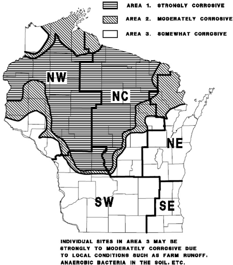
Figure 17. Potential for bacterial corrosion of zinc galvanized steel culvert pipe
