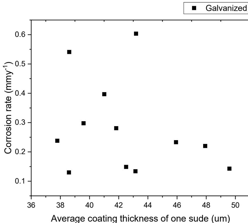
Figure 30. Corrosion rate result of galvanized pipe
