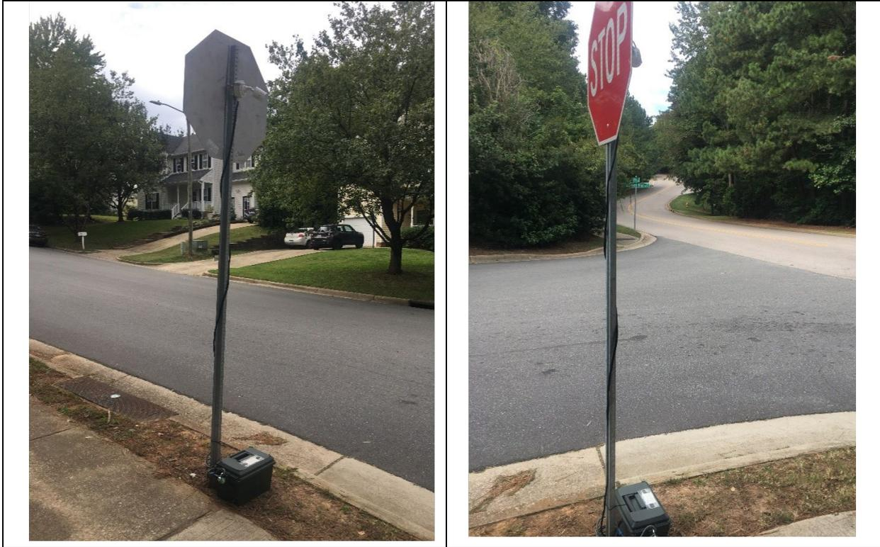
Figure 5. Example camera installation at Raleigh Site 2 with camera mounted to back of STOP sign to capture activity along Lineberry Dr. at the intersection with Trailwood Hills Dr.
