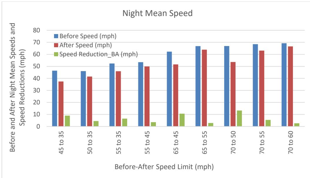
**Figure 8: Nighttime mean speeds in the before and after periods along with the nighttime mean speed reductions (number of sites = 50)**
