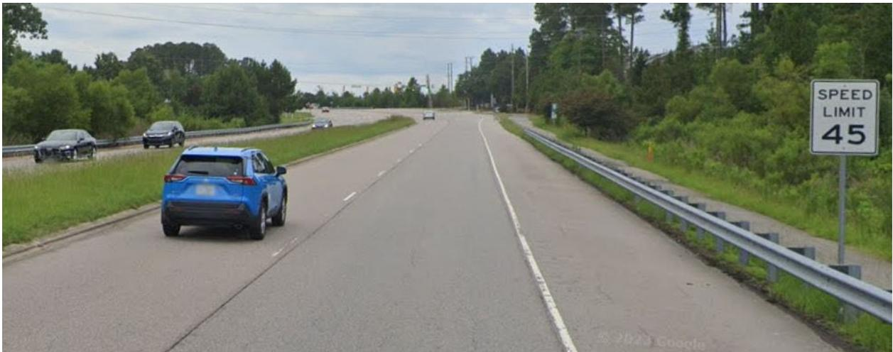
**Figure 188: Conventional speed limit sign**
