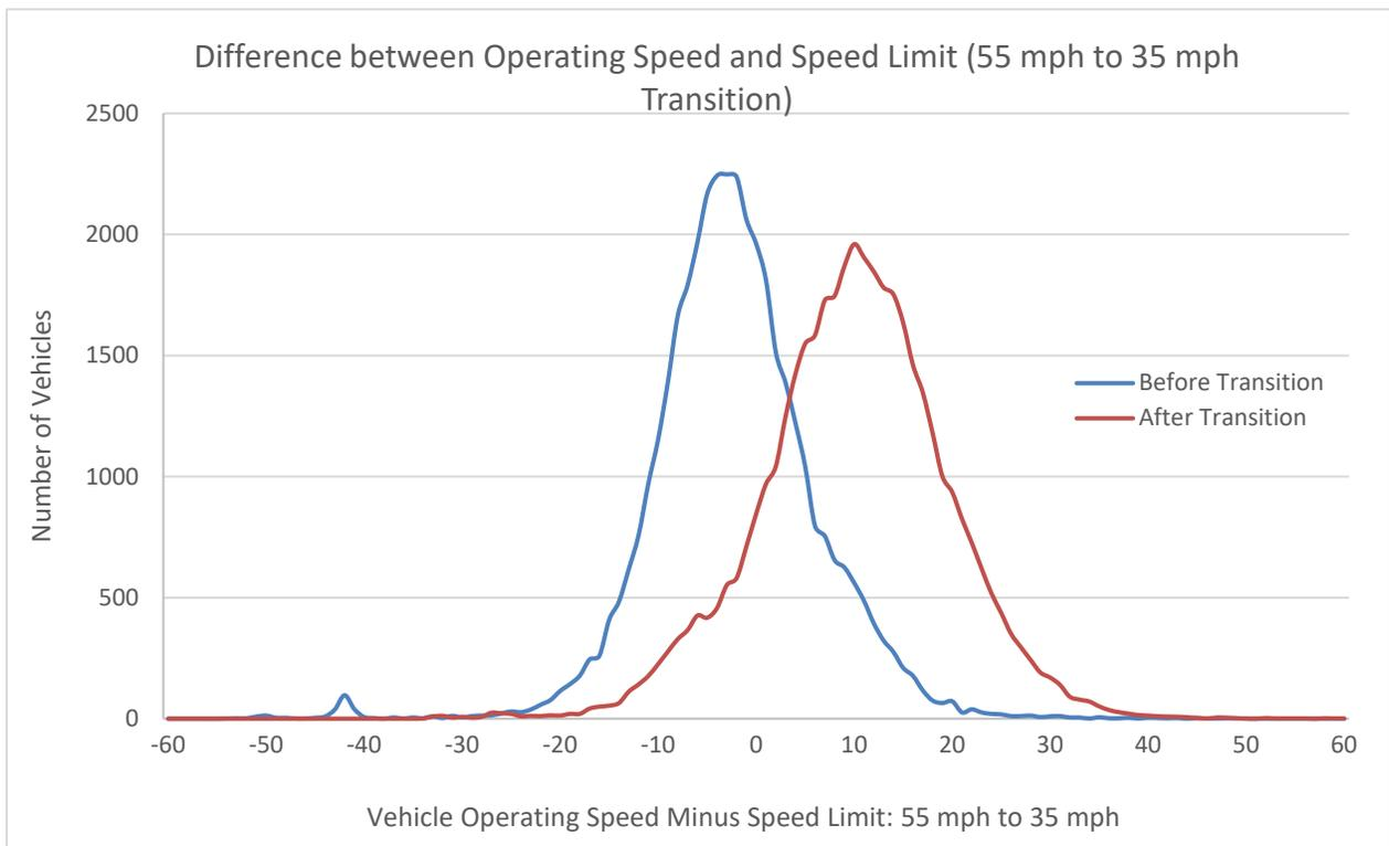
**Figure 15: Difference between vehicle operating speed and speed limits for 55 mph to 35 mph transition (number of sites = 10)**
