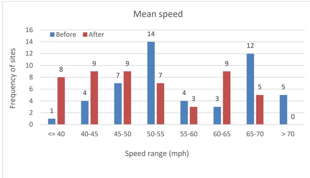
**Figure 3: Number of sites before and after speed transition based on different mean speed ranges (number of sites = 50)**
