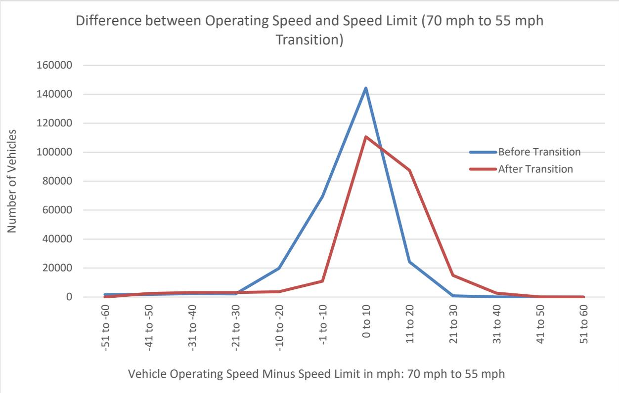
**Figure 17: Difference between vehicle operating speed and speed limits for 70 mph to 55 mph transition (number of sites = 7)**
