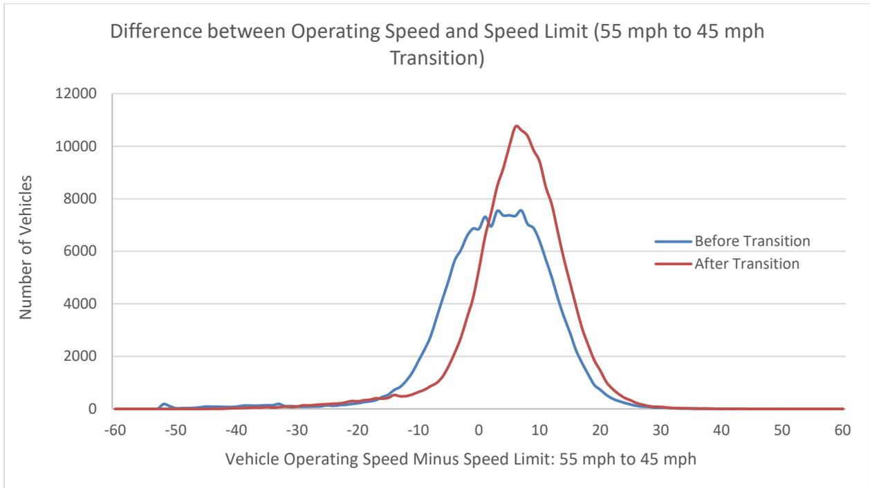
**Figure 16: Difference between vehicle operating speed and speed limits for 55 mph to 45 mph transition (number of sites = 10)**
