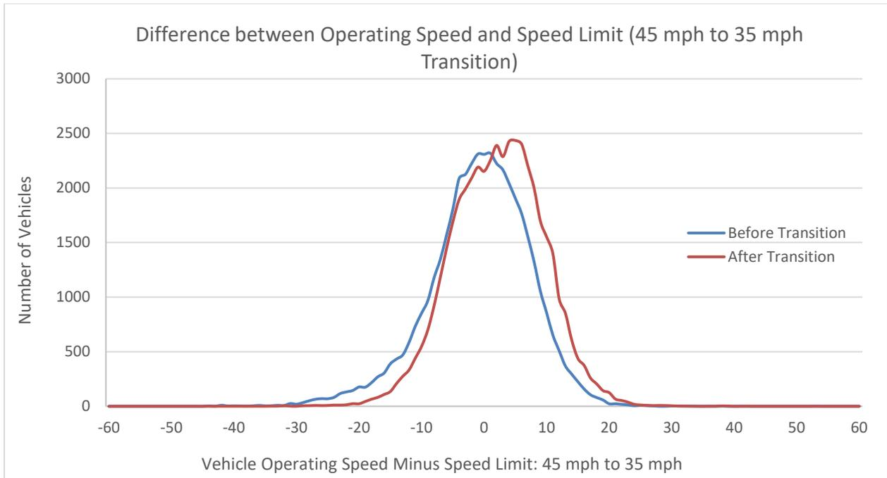
**Figure 14: Difference between vehicle operating speed and speed limits for 45 mph to 35 mph transition (number of sites = 6)**
