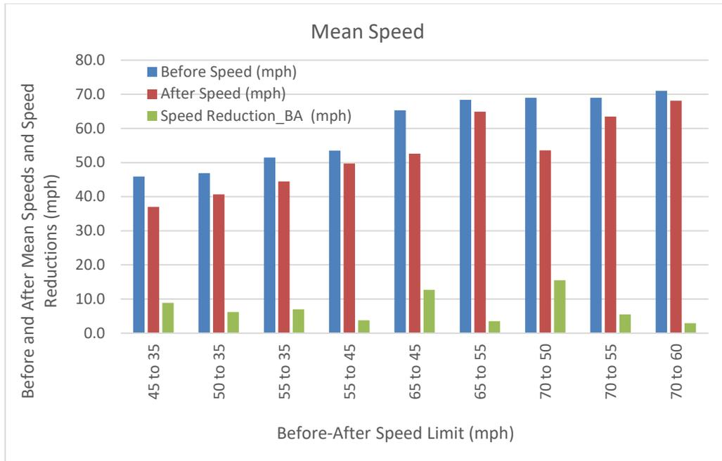
**Figure 6: Mean speeds in the before and after periods along with the mean speed reductions (number of sites = 50)**
