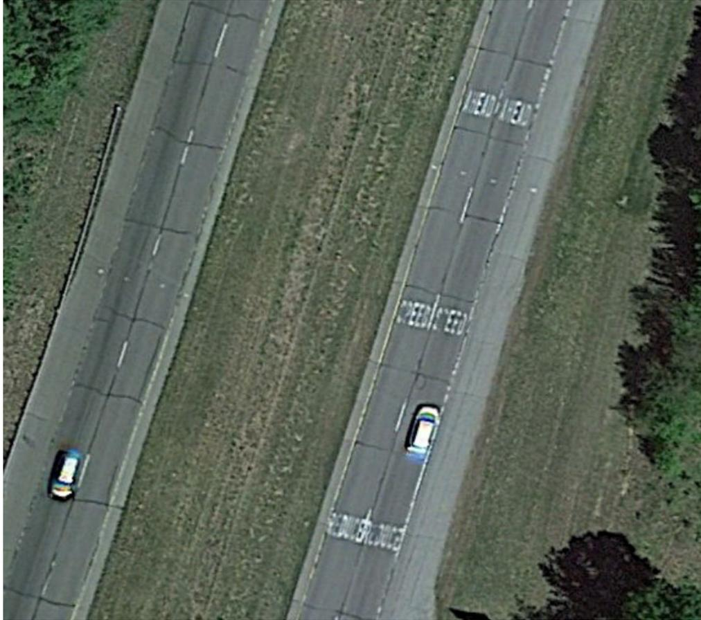
**Figure 1: Example of supplemental pavement markings where the transition zone is indicated by markings painted on the roadway surface.**
