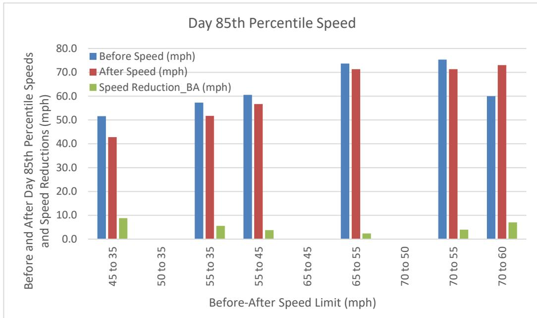
**Figure 11: Daytime 85<sup>th</sup> percentile speeds in the before and after periods along with the daytime 85<sup>th</sup> percentile speed reductions (number of sites = 37)**
