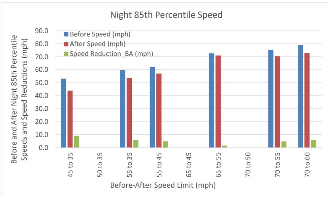
**Figure 9: Nighttime 85<sup>th</sup> percentile speeds in the before and after periods along with the nighttime 85<sup>th</sup> percentile speed reductions (number of sites = 37)**
