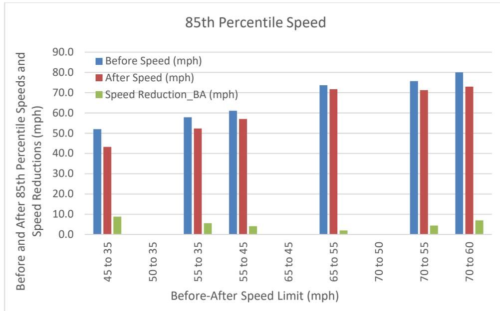
**Figure 7: 85<sup>th</sup> Percentile speeds in the before and after periods along with the 85<sup>th</sup> percentile speed reductions (number of sites = 37)**
