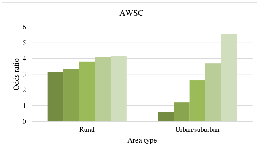
Figure E-2. Relationship between odds ratio and area type for AWSC intersections converted to mini-roundabouts.
