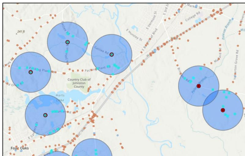
Figure 2-3. Washout locations buffered to select nearby non-washouts.
