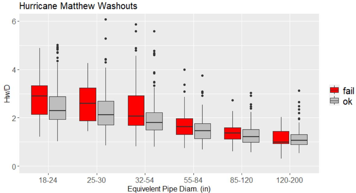
Figure 3-9. Ratio of headwater to structure diameter (Hw/D) for Hurricane Matthew washouts versus non-washouts.
