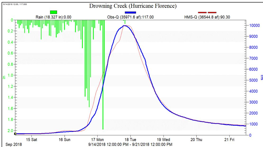
**Figure 6-1. Observed and HMS-simulated discharge hydrograph at the outlet of Drowning Creek.**
