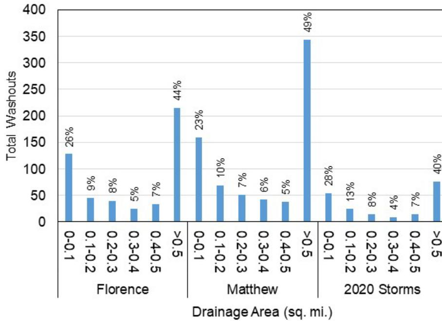
Figure 3-2. Structure washouts by drainage area (less than 0.5 square miles).
