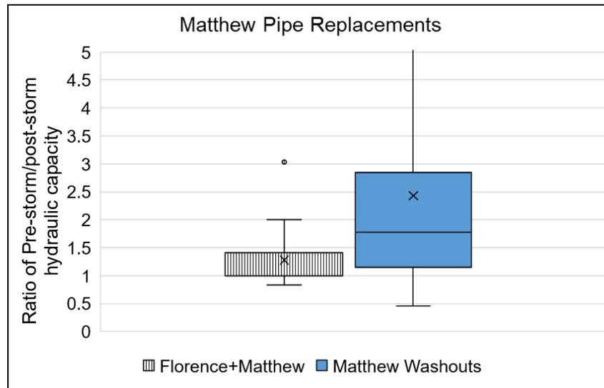
**Figure 3-12. Ratio of pre- to post-Matthew hydraulic capacity of washout locations. The blue box represents locations that washed out during Matthew but not Florence. The hatched box represents locations that washed out during both storms.**
