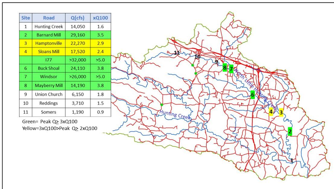
Figure 3-48. Overtopping discharges for North Little Hunting Creek (green highlight is ≥3 times 100-yr Q; yellow highlight is 2-3 times the 100-yr Q; no highlight is <2 times 100-yr Q).
