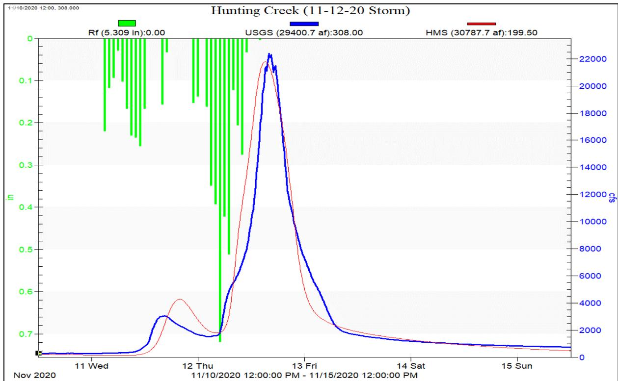
**Figure 6-2. Observed and HMS-simulated discharge hydrograph at the outlet of Hunting Creek.**
