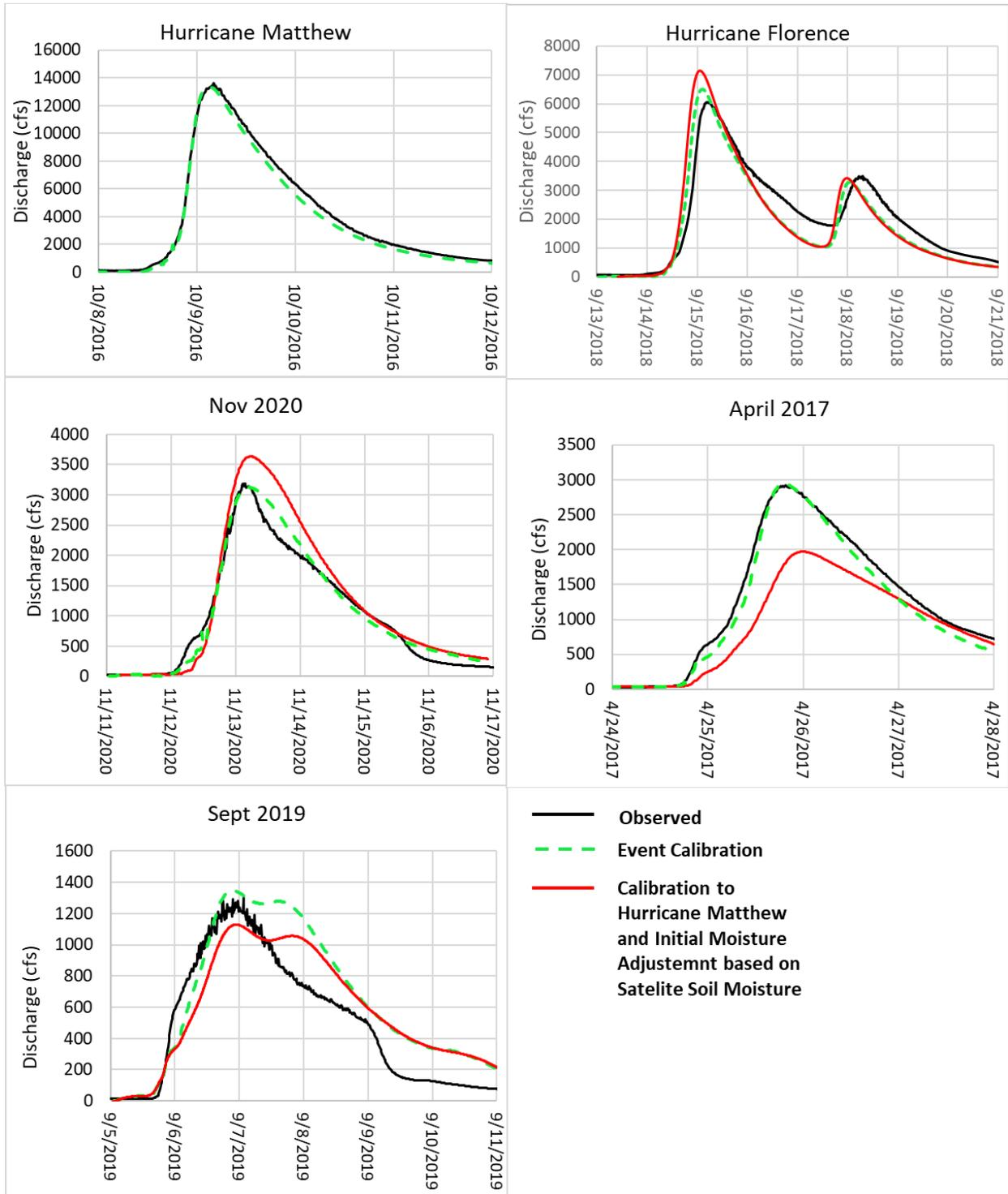
**Figure 3-22. Calibration/validation results for HEC-RAS rain-on-grid model for Nahunta Swamp watershed.**
