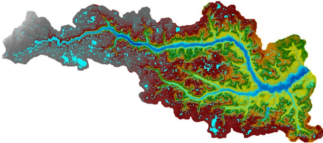
*Figure 3-21. Rain-on-grid model results showing WSE over topography.*
