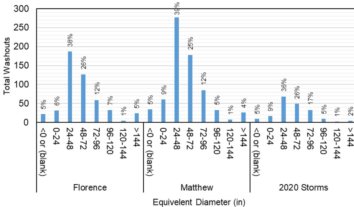
Figure 3-3. Washouts by equivalent pipe diameter.
