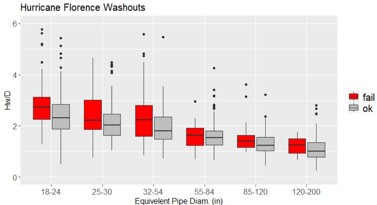
Figure 3-10. Ratio of headwater to structure diameter (Hw/D) for Hurricane Florence washouts versus non-washouts.
