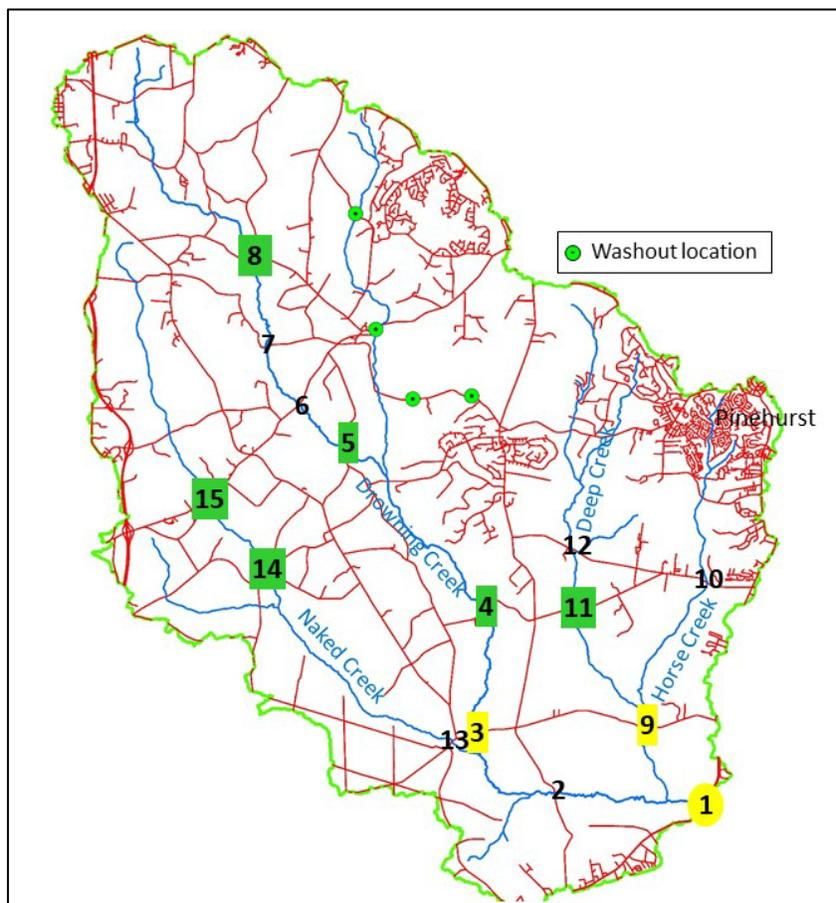
**Figure 3-46. Overtopping discharges for major stream crossings in Drowning Creek (green highlight is  $\geq 3$  times 100-yr  $Q$ ; yellow highlight is 2-3 times the 100-yr  $Q$ ; no highlight is  $< 2$  times 100-yr  $Q$ ).**
