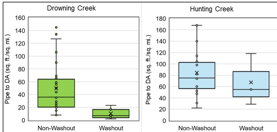
Figure 3-45. Pipe area to drainage area ratio for washout and non-washouts in Drowning and Hunting Creeks.
