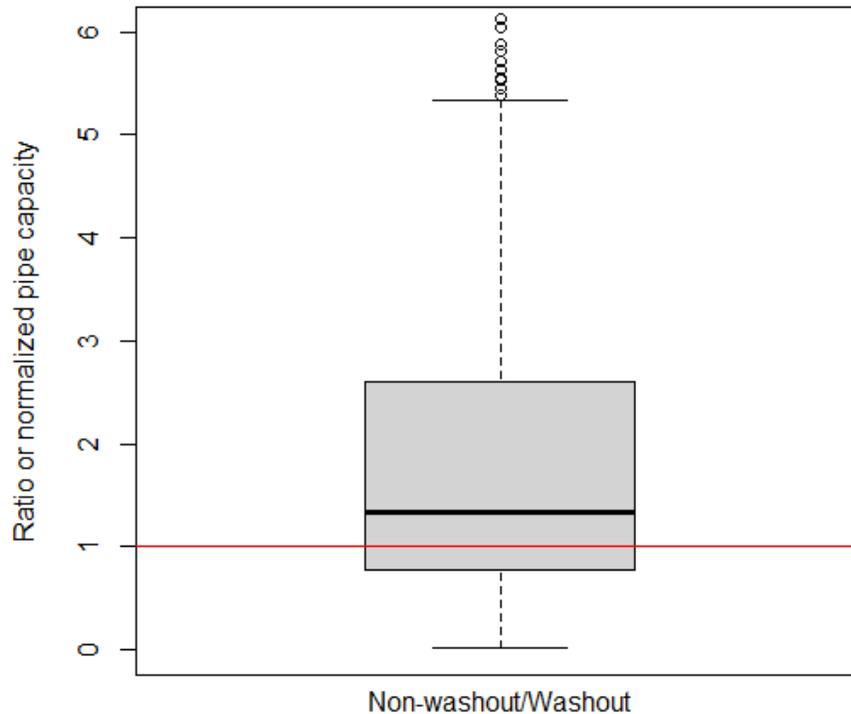
**Figure 3-11. Ratio of normalized pipe capacity (pipe flow area/watershed area) between non-washout and adjacent washout locations. Red line indicates equal normalized size for washout and nearest non-washout.**
