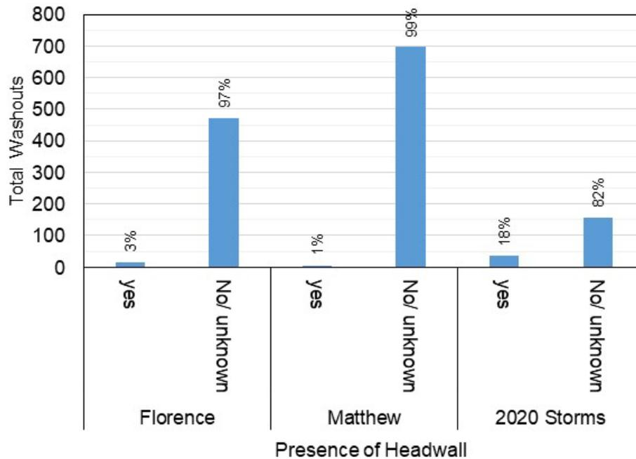
Figure 3-6. Structure washouts by headwall presence.
