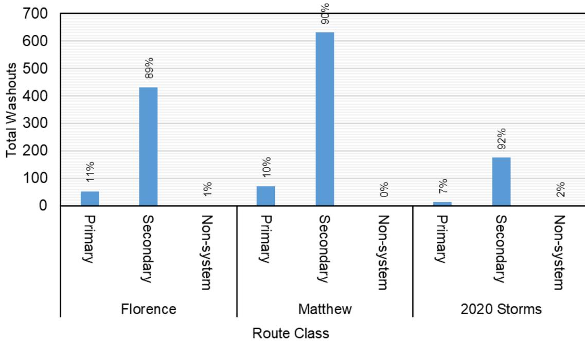
Figure 3-5. Structure washouts by road classification.
