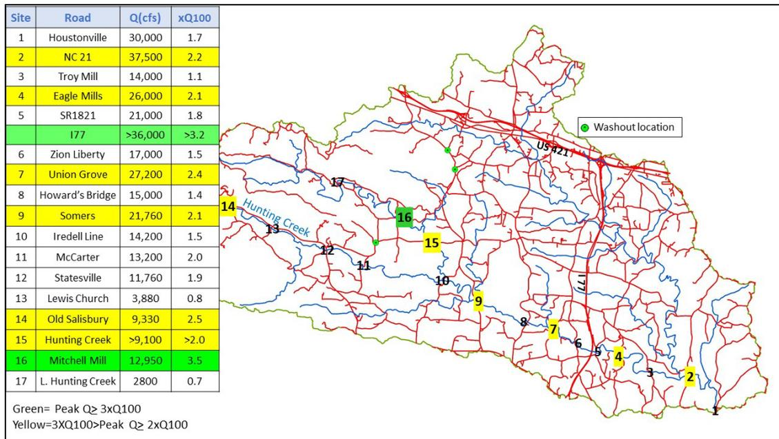
Figure 3-47. Overtopping discharges for Hunting Creek (green highlight is ≥3 times 100-yr Q; yellow highlight is 2-3 times the 100-yr Q; no highlight is <2 times 100-yr Q).
