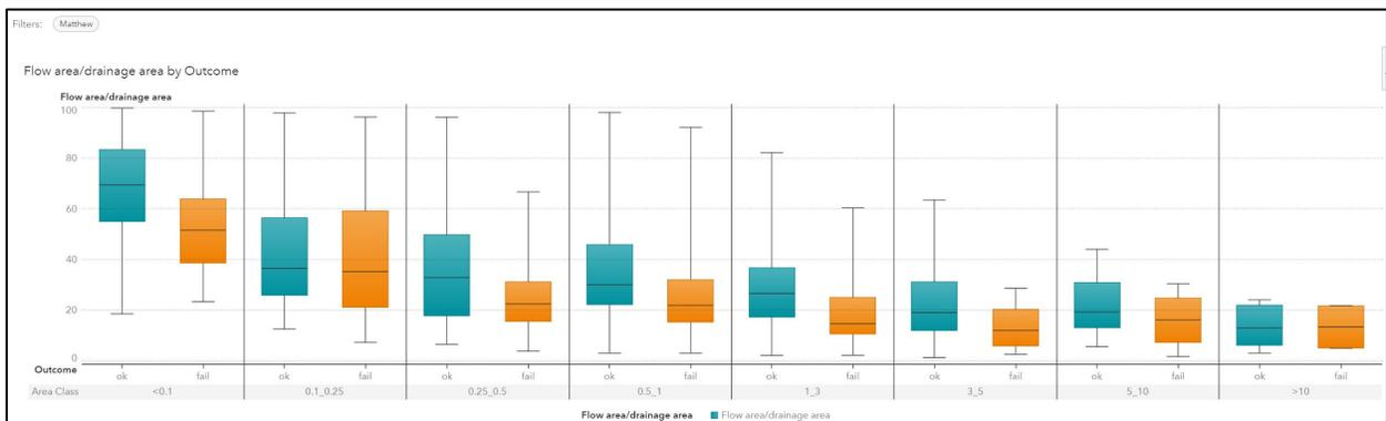
**Figure 3-15. Comparison of flow area to drainage area for washout and non-washout structures sorted by watershed area for Hurricane Matthew**
