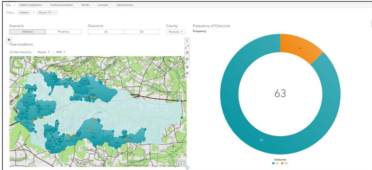
**Figure 3-17. Washout and non-washout locations compared for Subbasin 913 in Wayne County.**
