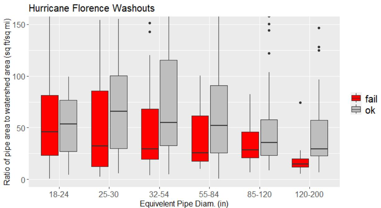
**Figure 3-8. Ratio of pipe area to watershed area for Hurricane Florence washouts versus non-washouts.**
