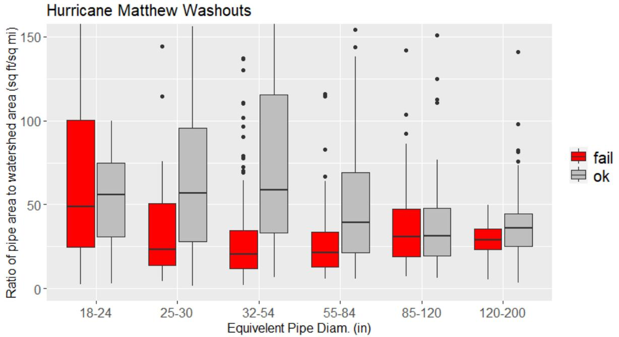
**Figure 3-7. Ratio of pipe area to watershed area for Hurricane Matthew washouts versus non-washouts.**
