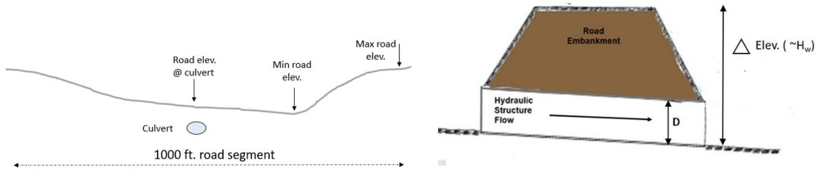
Figure 2-5. Example of elevation data-based parameters
