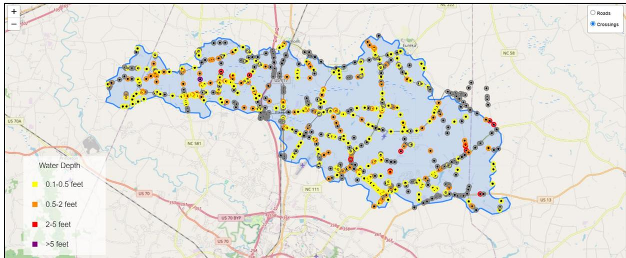
*Figure 3-30. HTML view of structure inundation for the 100-year storm.*
