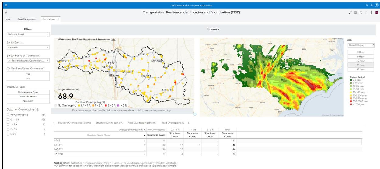
**Figure 3-41. Storm Viewer tab for Hurricane Florence indicating the 24-hour design storm equivalent rainfall (right) and structure and road overtopping summary for all structures in Nahunta Swamp basin and road segments along 68.9 miles of resilient routes.**
