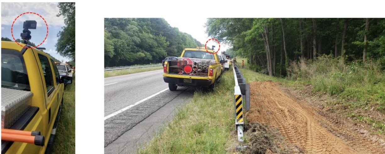
Figure 7 Mounting the sensor on work vehicles
