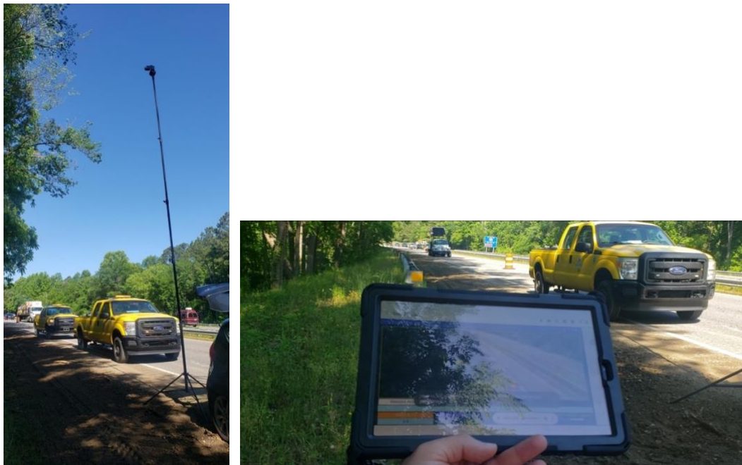
Figure 5 20' tripod stand mount and controlling the sensor via a tablet device
