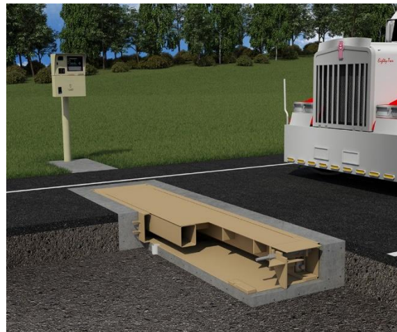
Figure 5 Slow-Speed In-Motion Load Cell-Based Scales
