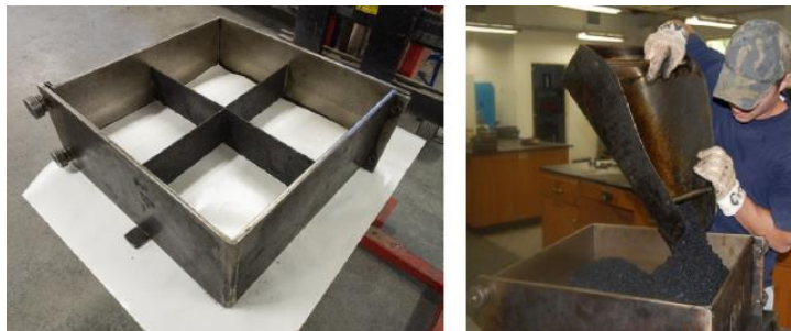
Figure A.15. Technician pouring a batch into the partitioned compaction mold.
