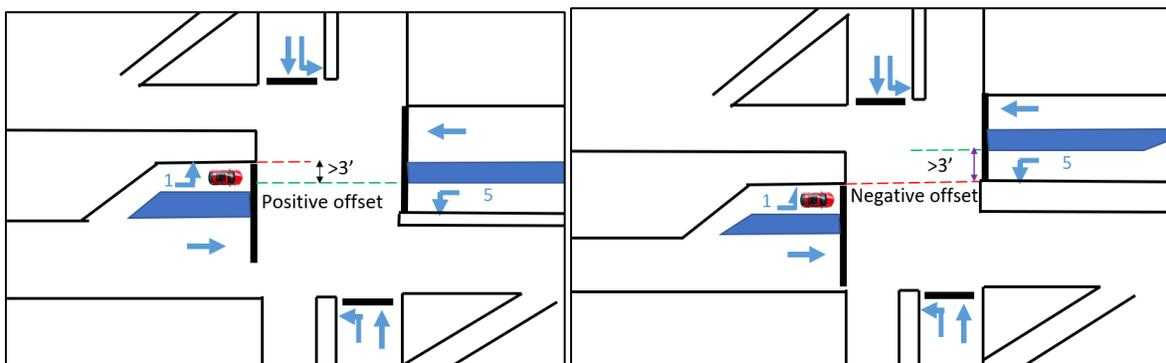
**Figure 3-5:** Lateral offset for permissive and protected-permissive left-turns
