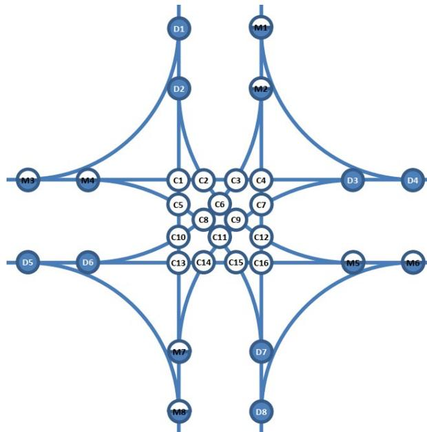
**Figure 3-2:** Conflict point diagram for a conventional four-legged intersection (Rodegerdts et al., 2004)
