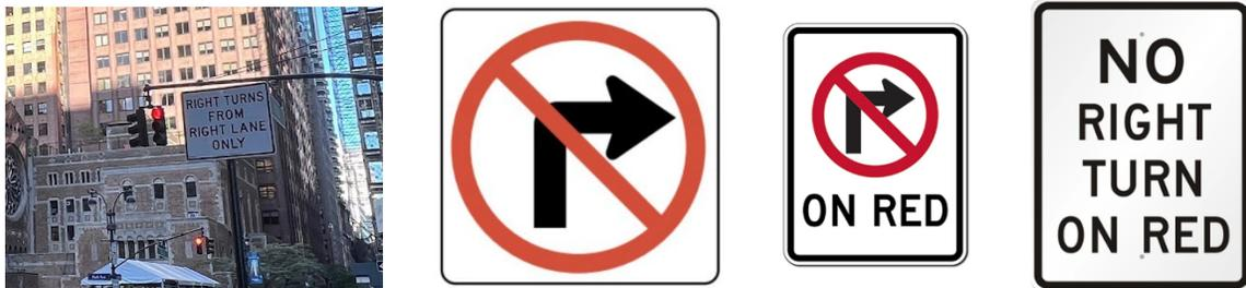
Figure 3-7: Different types of mandatory signs for right-turning traffic
