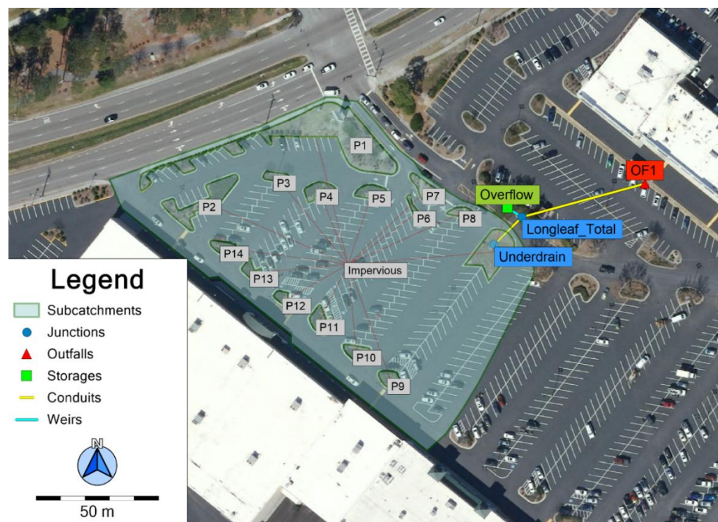
Figure 4. PCSWMM diagram of the DDB site
