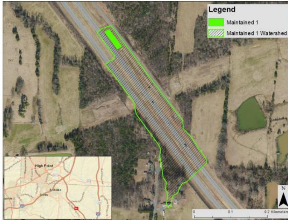
Figure 6. Aerial view of DDB (referred in figure as “Maintained 1”) illustrating the watershed area and area occupied by the DDB (Wissler, 2019)
