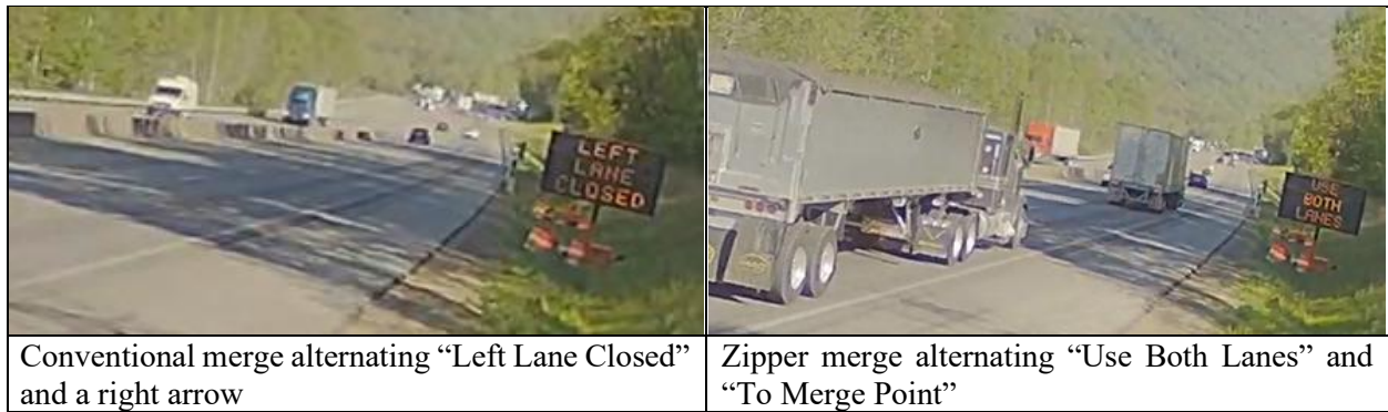
Figure 12. Portable changeable message sign displays prior to, and after, spillback at the choke point.
