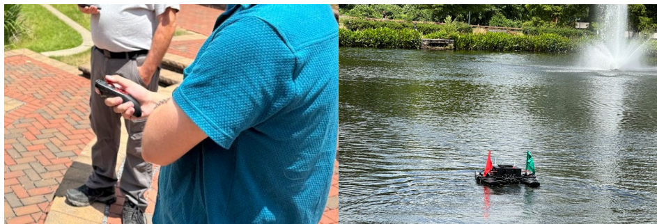
Figure 76: Left: The vehicle is controlled with a one-handed joystick controller by a student, similar to used for remote-control hobby boats. Right: USV deployed on Hechenbleikner Lake on UNC Charlotte's campus.
