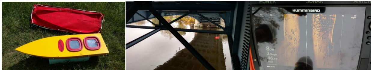
Figure 9: The Sonar EMILY system prior to deployment. Middle: Image of Sonar EMILY near a bridge site. Right: Example of commercial fish finder onboard the Sonar EMILY system and wireless transmitted to operators on shore.
