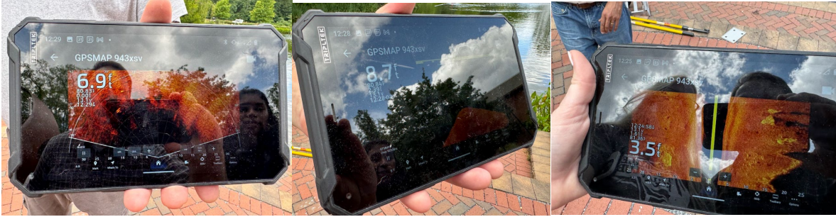
Figure 77: Examples of three modes of the sonar data collection from left to right: LiveScope, ClearVu, and SideVu as observed during the on-campus test.
