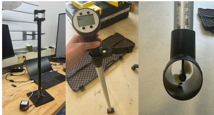
Figure 32. Left: Ultrasonic anemometer, Middle and Right: Water current flow probe.
