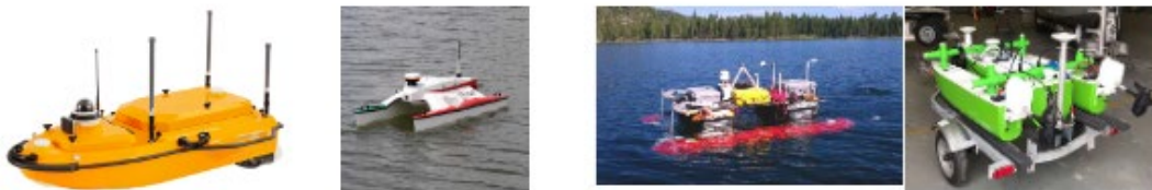
Figure 16: Hull designs of USVs. (Left) Monohull (Image Source: CHCNAV, 2024), (Left-Middle) Catamaran (Image Source: Rasal, 2013), (Right-Middle) Catamaran-SWATH (Image Source: YSI, 2024), (Right) Trimaran (Image Source: Triaddrones, 2024).
