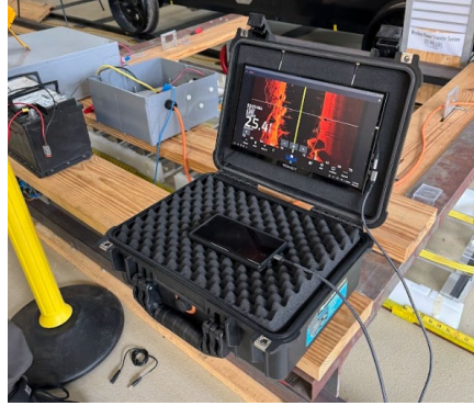
Figure 73: Monitor displaying sonar data in benchtop demo/test mode. The screen can be used to mark GPS locations of objects encountered during the mission as well as to record imagery for later review.
