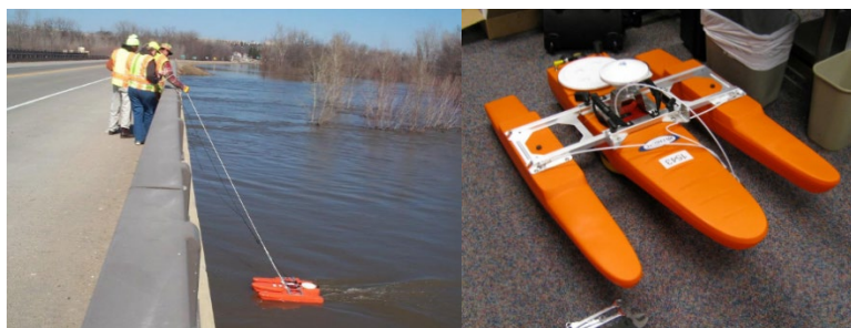
Figure 11: OceanScience Riverboat SP equipped with a TRDI StreamPro acoustic Doppler current profiler being deployed during a flood to measure discharge (Source: Bartelt, 2017)
