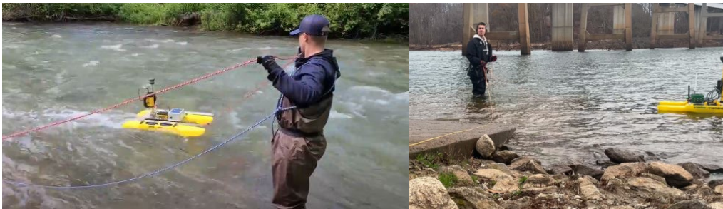
Figure 65: Tethered test in rapidly flowing water.
