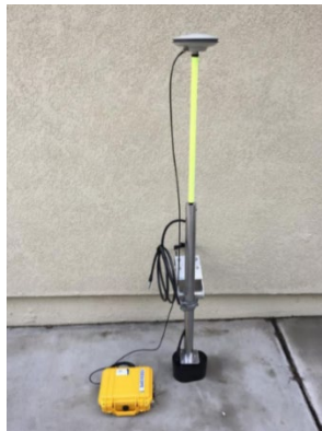
Figure 1. An example single-beam echo sounder (SBES) that can be mounted to a boat for manual surveys. The image shows the CEESCOPE developed by HydroSystems. Image Source: https://ceehydrosystems.com
