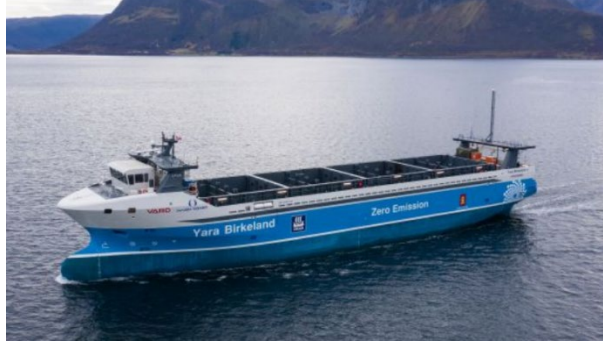
Figure 13: An all-electric container ship, the Yara Birkeland, is capable of operating in fully autonomous mode.
