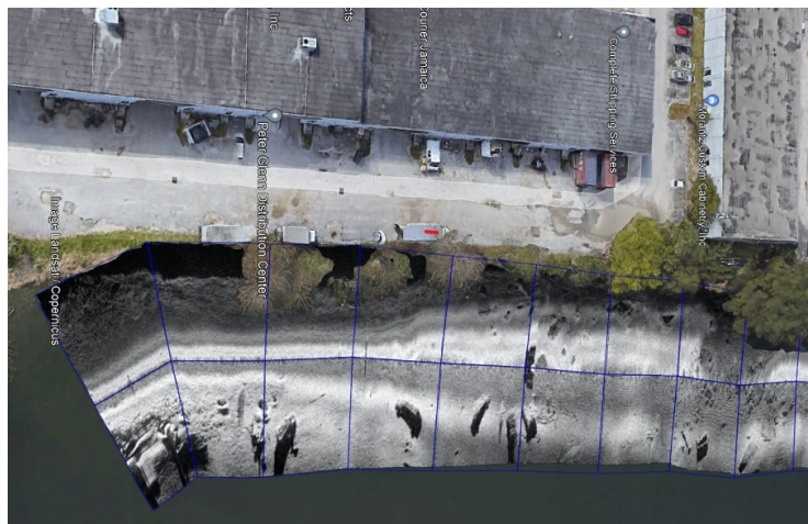
Figure 74: Example side-scan mosaic from Helo & Sub data collected in Florida.
