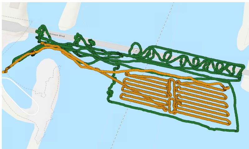
Figure 80: Two data collection runs were executed using the Hydrone USV. The first run (green markers) consisted of a remotely piloted survey in the vicinity of the bridge and an outline of a “box” in which to conduct the second automated survey (orange markers).
