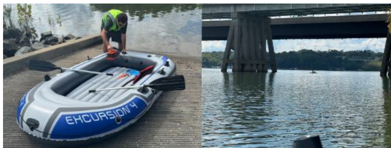
Figure 63: Manned inflatable raft used to transport operators to the survey site (left), and the HyDrone completing an autonomous survey once arrived at the off-site location.
