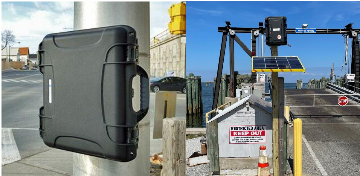
Figure 4: SMATS Hardware Installation Example (without solar panel)[left], SMATS Ferry Sensor 2 Installation [right]
