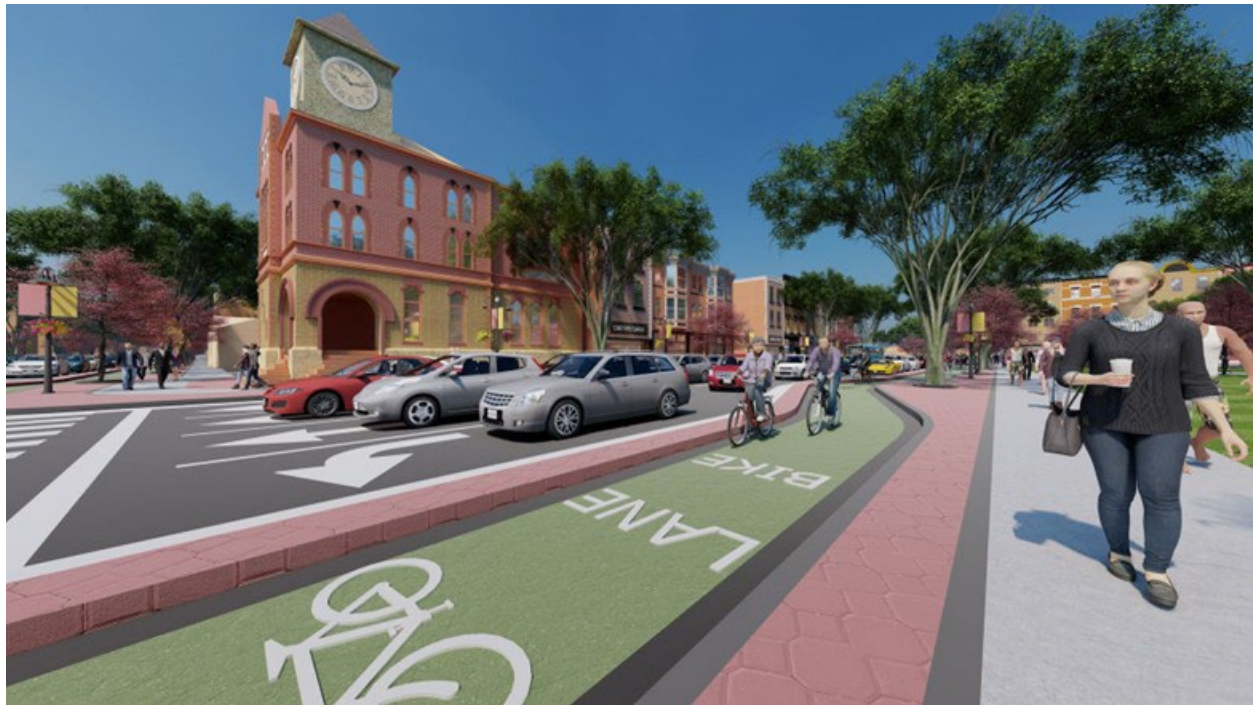
Figure 5-10 One-Ways can make space for protected cycle tracks and street trees.
