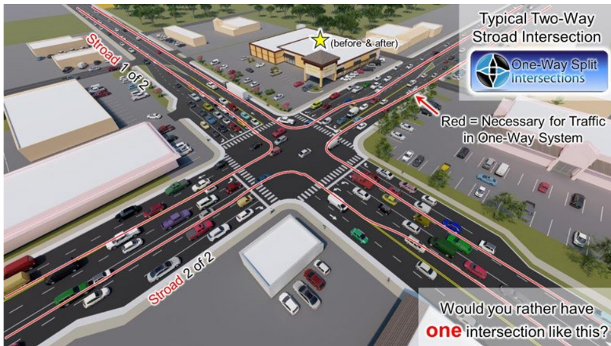
Figure 5-11 Typical Stroad Intersection with Double-Left Turns and Dedicated Right Turn Lane
