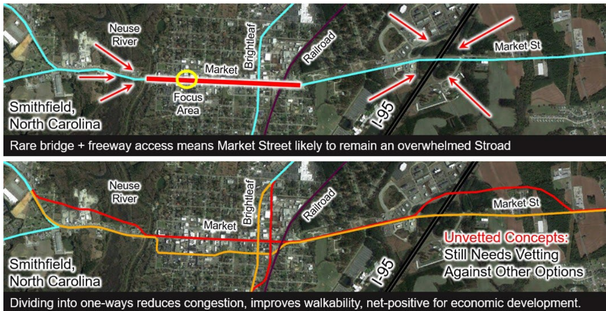
Figure 5-1 As pressure increases on Market St., one-ways could offer win-win for Placemaking and Traffic
