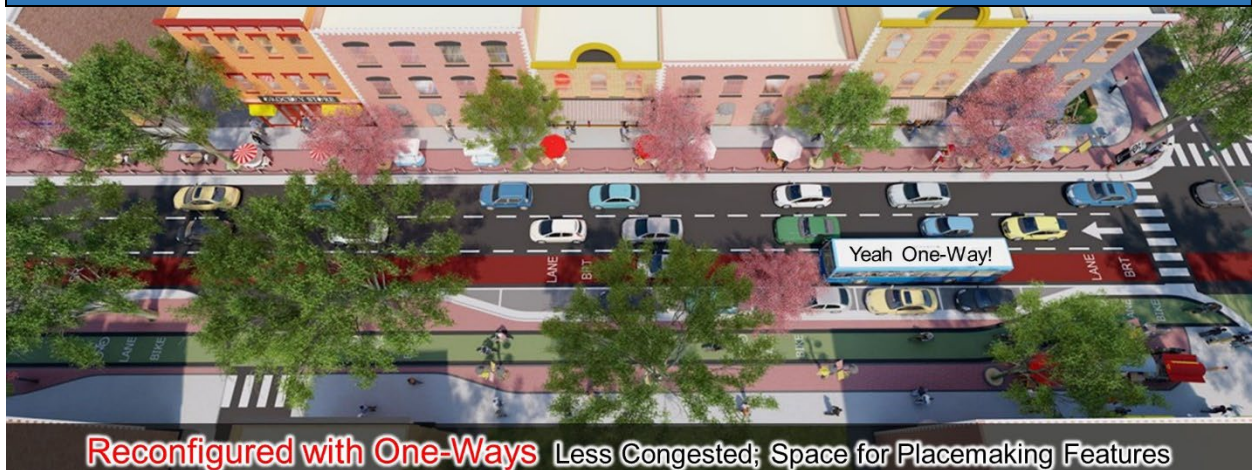
Figure 5-4 Today's two-way Stroad w/Parking, vs default future (5-lane), vs One-ways w/space for other uses.
