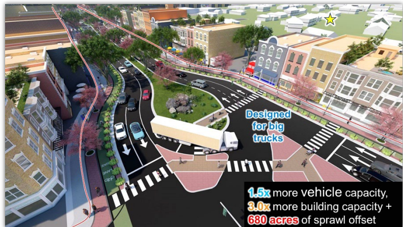
Figure 4-11 Accommodating trucks in a walkable, mixed-use environment.
