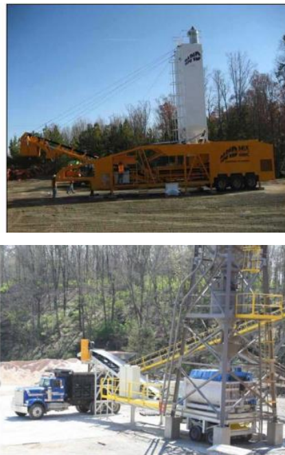
Figure 2.5. Twin shaft mixers used in RCC mix production
