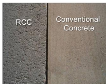
Figure 2.4. RCC surface texture as compared to conventional concrete pavement
