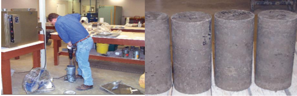
Figure 2.7. Preparation of RCC compressive strength testing cylinders
