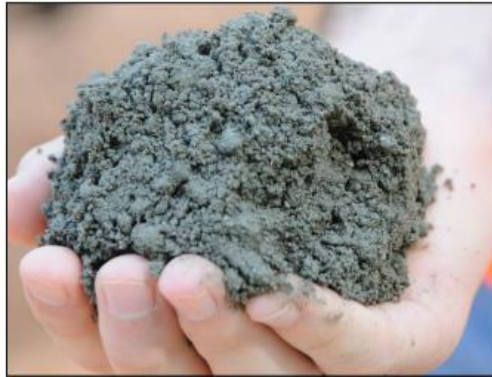
Figure 2.1. Consistency (stiffness) of RCC mixture
