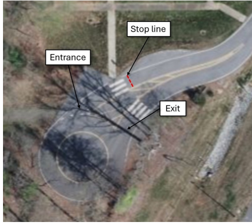
(a) Annotated aerial view of the roundabout showing entrance, stop line location, and exit region used for cooperative vehicle coordination.
