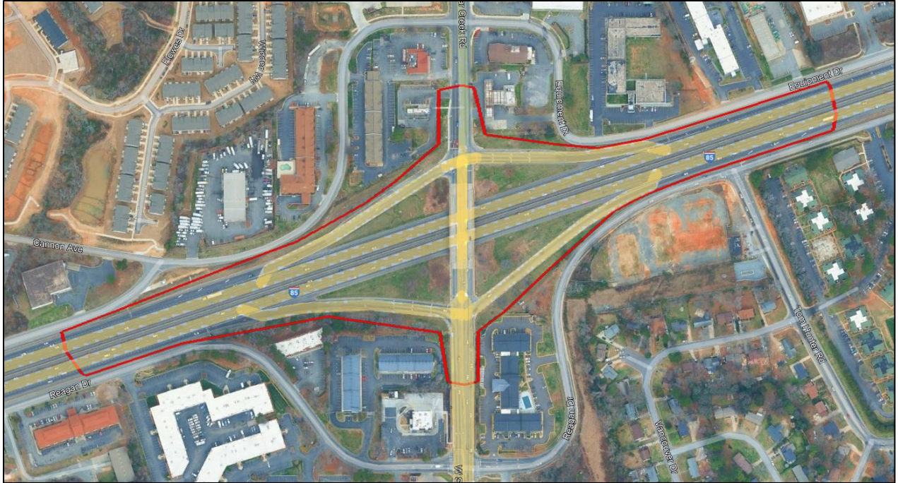
Figure 34. Interchange TSUINTC00336 - I-85, SR-2480, SR-2619, SR-2620, SR-2621, SR-2622, Cannon Av, Tom Hunter Rd (Diamond interchange)
