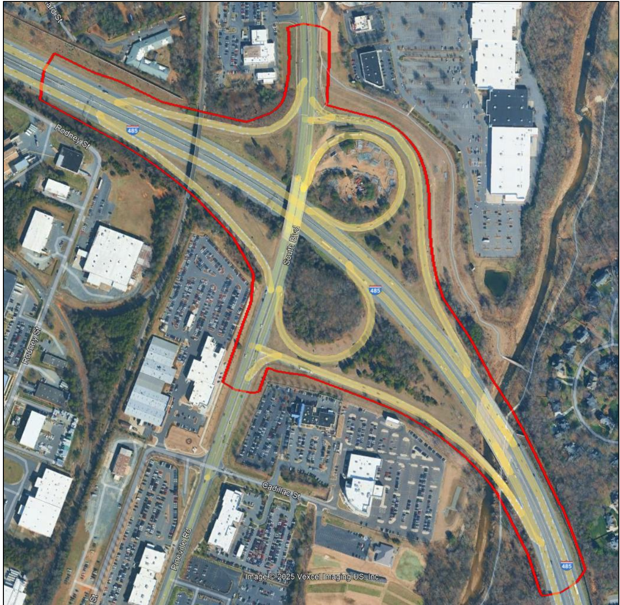
Figure 32. Interchange TSUINTC00295 - I-485, SR-3998, SR-4982, Rodney St, Packard St (PARCLO AB interchange)
