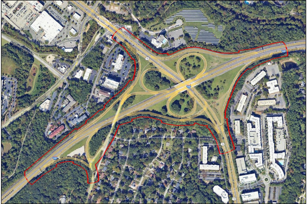
Figure 27. Interchange TSUINTC00098 - I-440, US-70, Ridge Rd, Ridge Rd To I-440 Ramp EB, Varnell Ave, Arrow Dr (PARCLO AB interchange)
