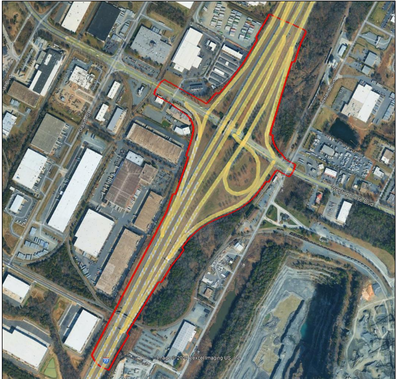
Figure 30. Interchange TSUINTC00206 - I-77, SR-1128, SR-1382, Westinghouse Blvd (PARCLO A interchange)
