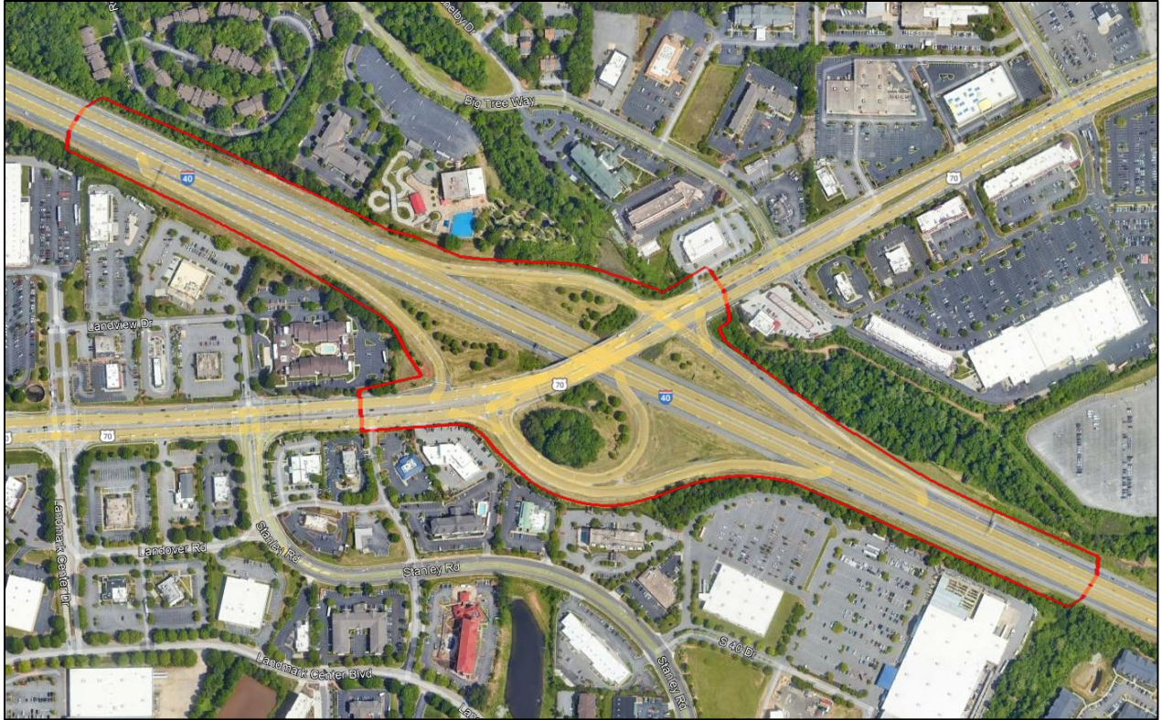
Figure 37. Interchange TSUINTC00617 - I-40, SR-1541, On Ramp I-40e, Lanada Rd, River Oaks Dr (PARCLO B interchange)
