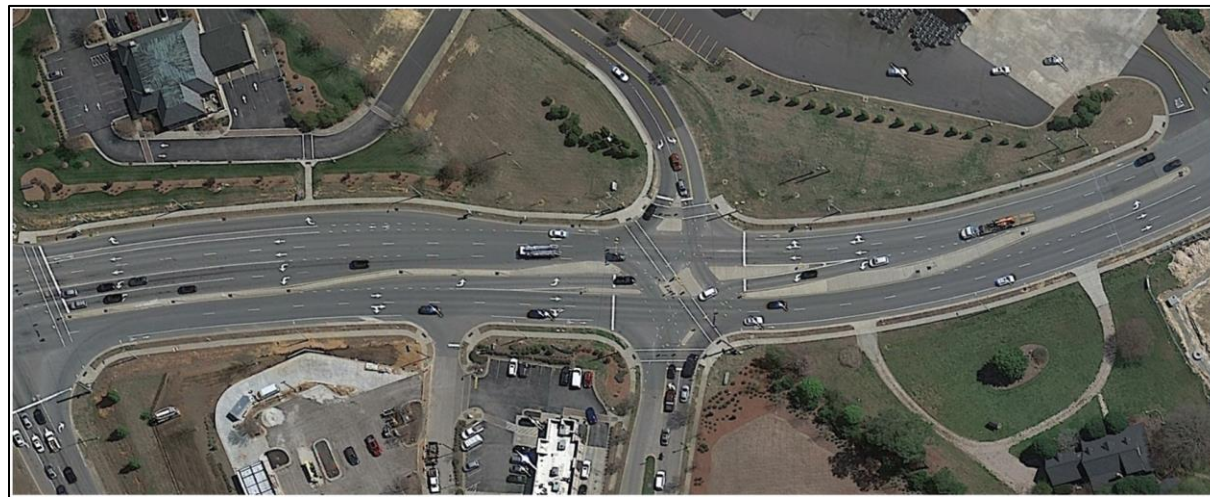
Figure 4.9 An Example of a Thru-cut Intersection without U-turn Crossovers in S Main St and Village Walk Dr in Holly Springs, NC
