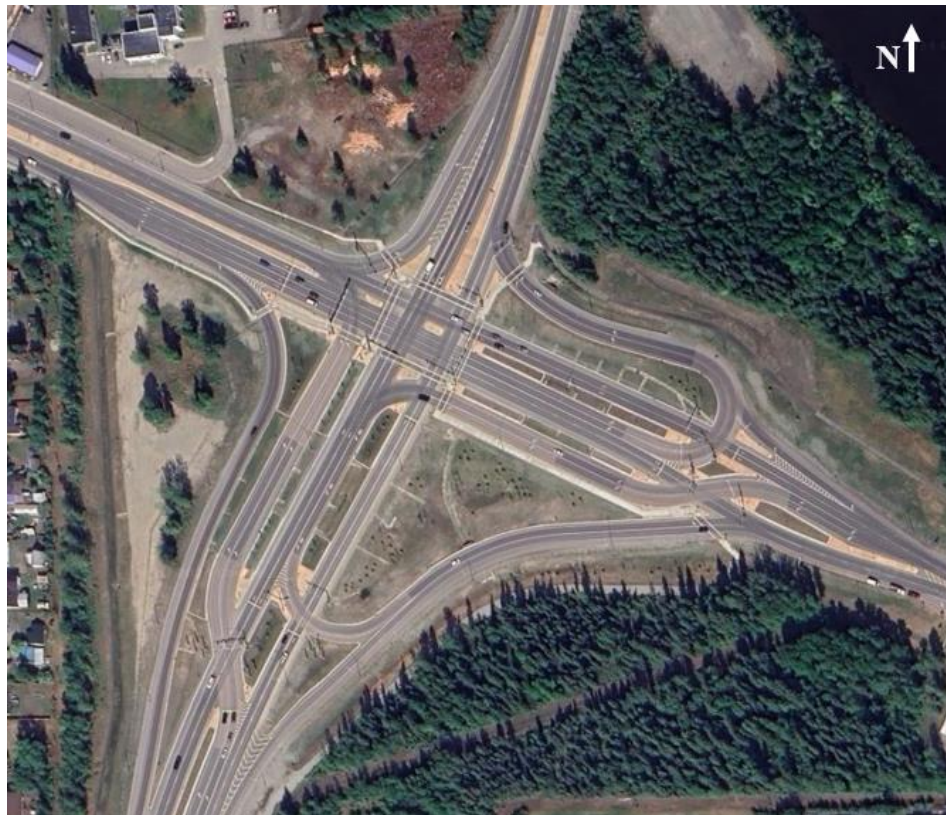
Figure 2.9 Full CFI/MUT Combo at Gaffney Road and Richardson Highway in Fairbanks, AK
