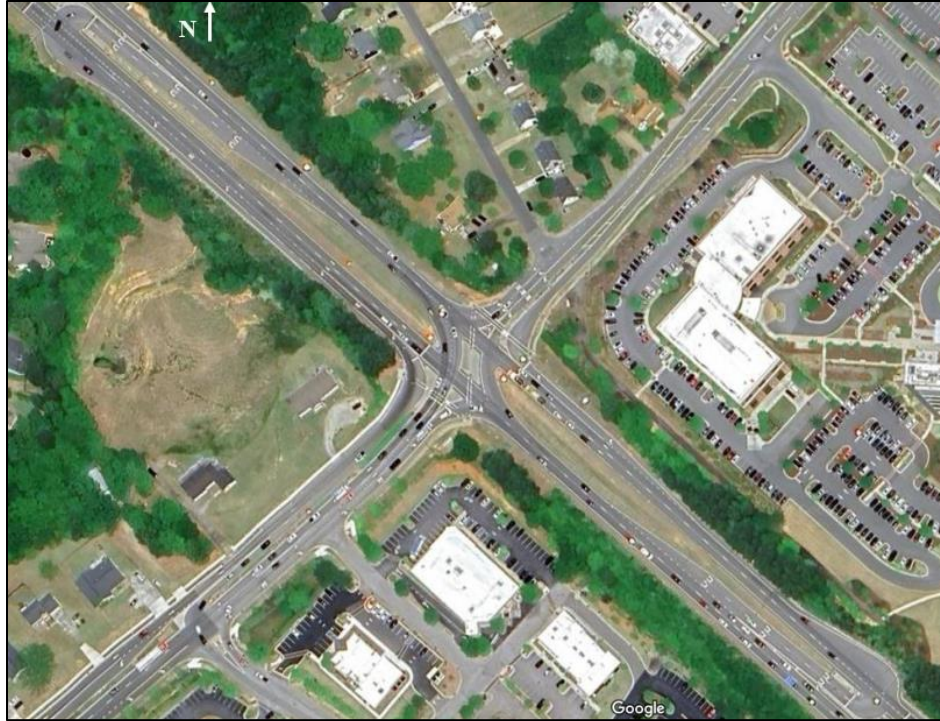
Figure 2.7 Reverse RCI at GB Alford Highway/Avent Ferry Road in Holly Springs, NC
