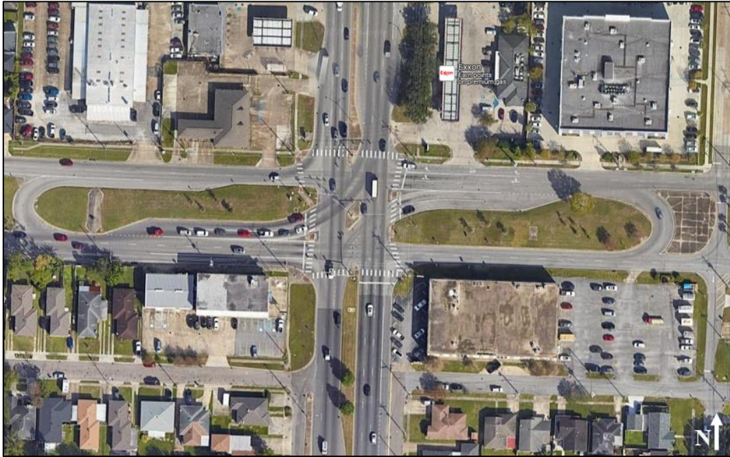
Figure 2.4 MUT Redirect Minor (Partial MUT#2) Located at W Napoleon Ave/N Causeway in New Orleans, LA
