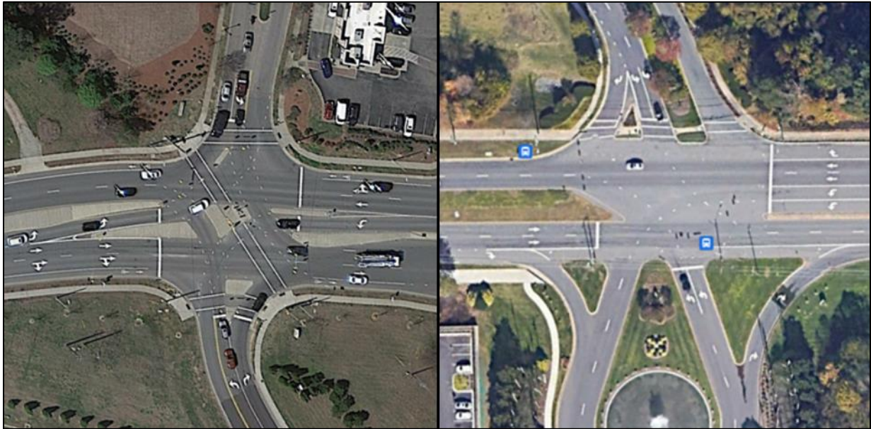
Figure 2.11 Thru-Cut Intersections at Village Walk Dr/S Main St, Holly Springs, NC (Left) and Arrowood Rd/Arrowpoint Blvd, Charlotte, NC (Right)
