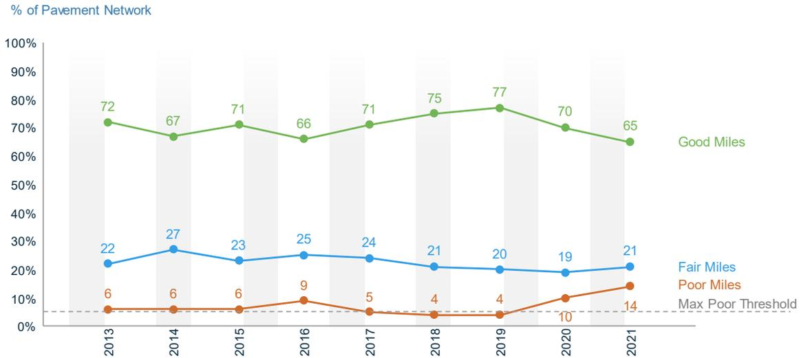
**Figure 5 Primary Network Pavement Condition, 2013-2021**
