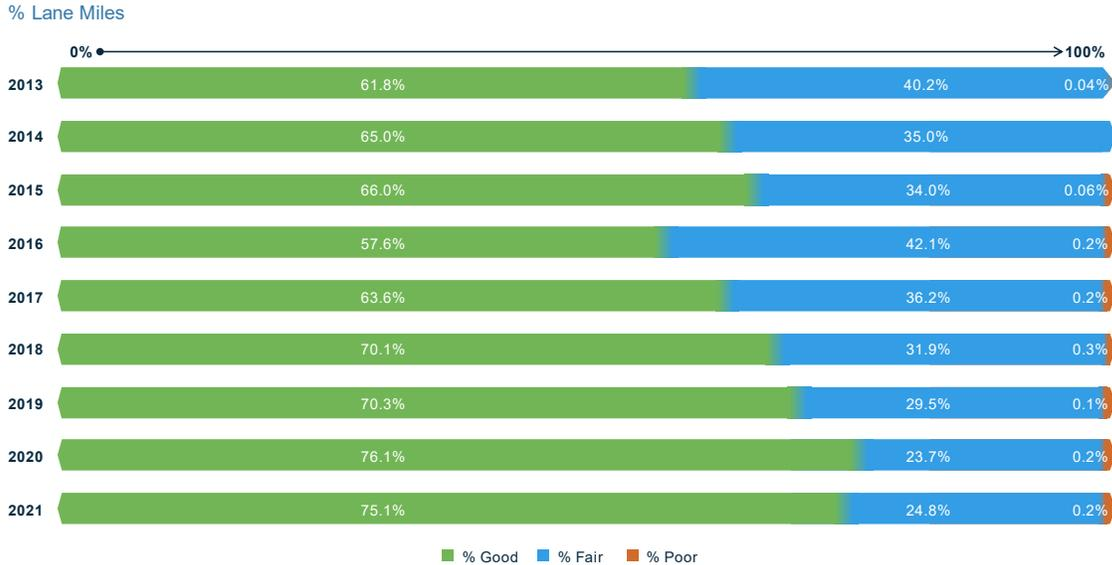
**Figure 7 NHS Interstate System Pavement Conditions**
