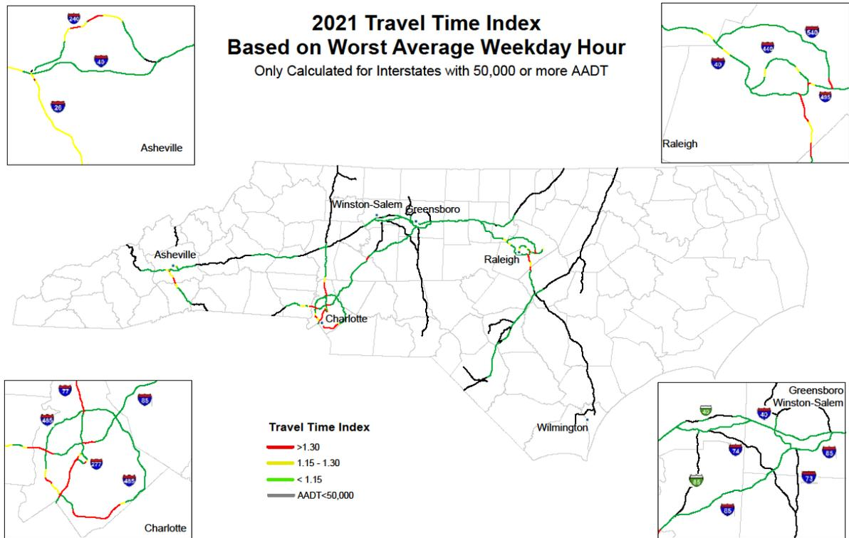
**Figure 11 Levels of Traffic Congestion on Heavily Travelled Interstates**
