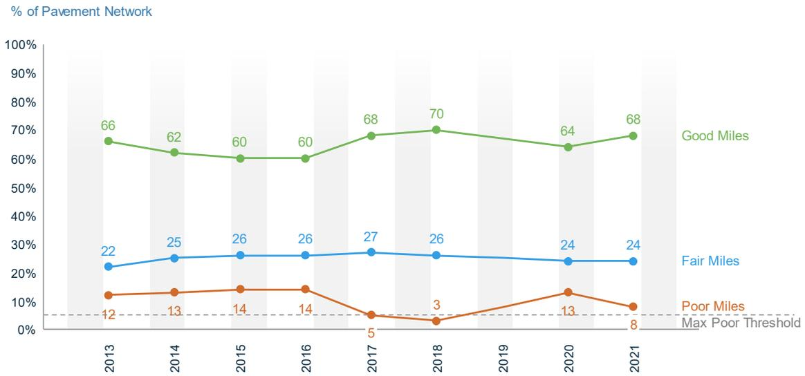
**Figure 6 Secondary Network Pavement Condition, 2013-2021**
