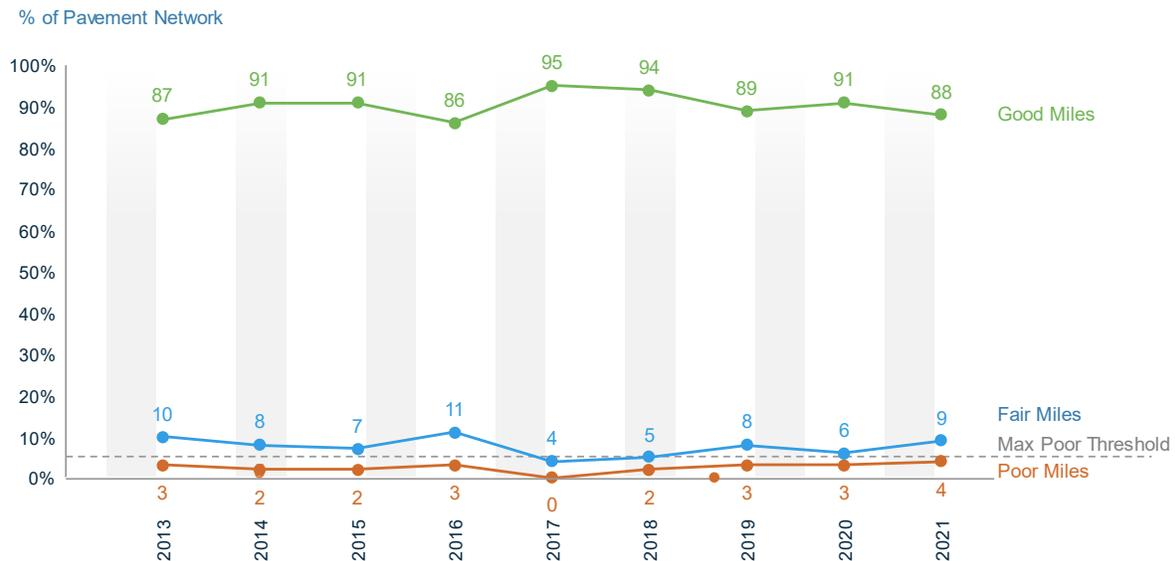
**Figure 4 Interstate Pavement Condition, 2013-2021**
