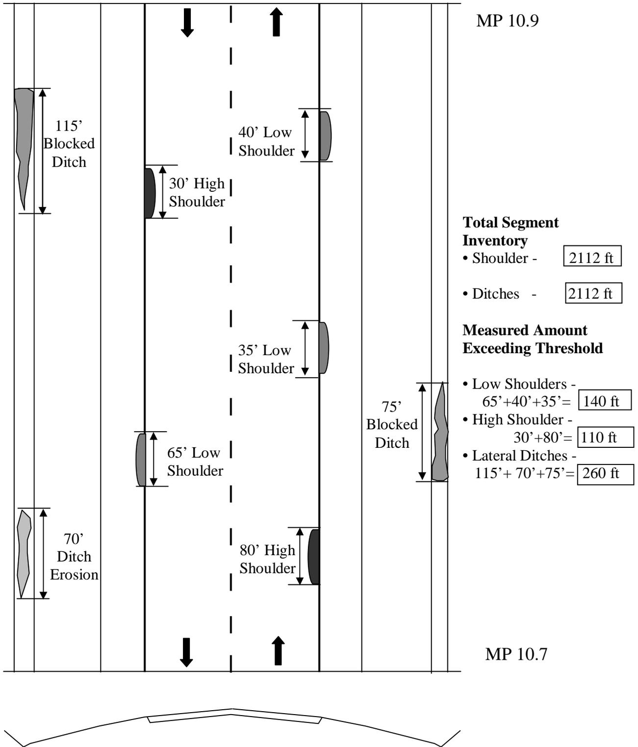
**Figure 3.5 – Example Roadway Conditions for Element 1**
