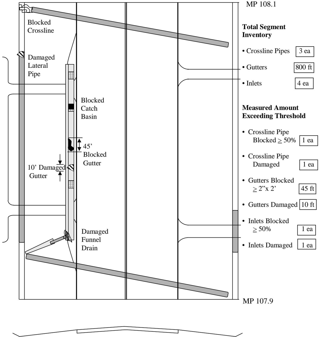
**Figure 3.12 – Example Roadway Conditions for Element 2**
