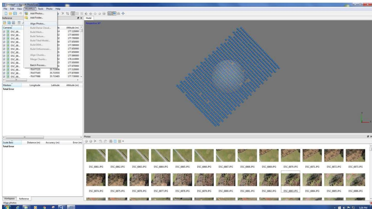
Figure 57: Align Photos Interface in Agisoft PhotoScan
