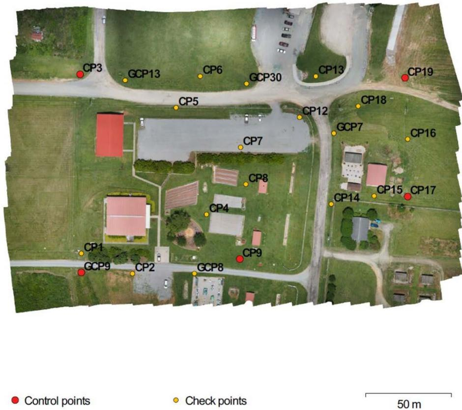
Figure 31: GCP Positions for Accuracy Analysis
