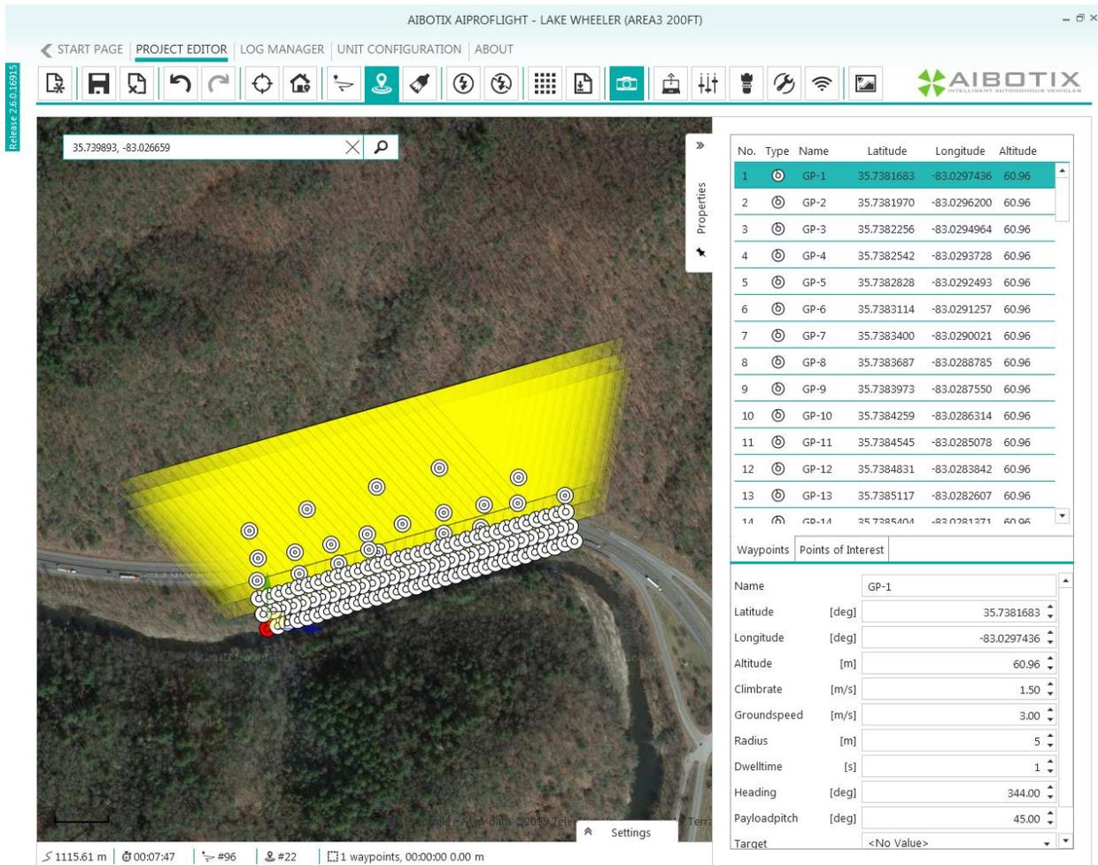
Figure 21: Haywood County Exposure Positions 60.96 m [200ft] AGL (Proposed Locations) (80% Overlap, Sensor Heading 344 Degrees, Pitch 45 Degrees, Aircraft Heading 74 Degrees)
