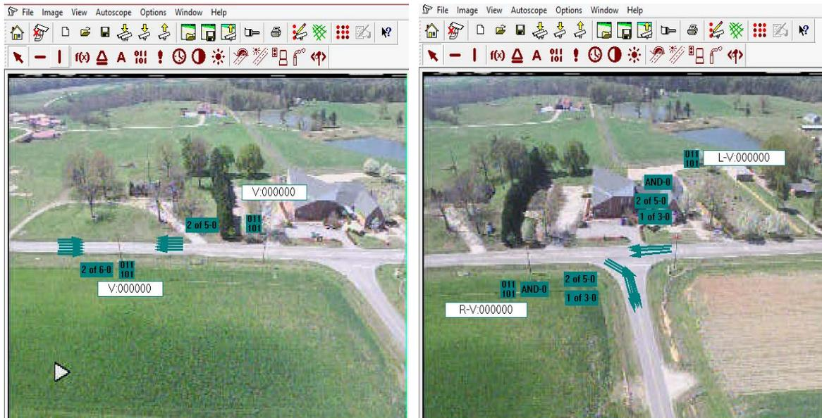
Figure 49: AutoScope thru (left) and turning (right) detectors
