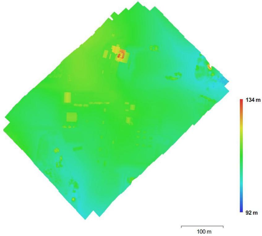
Figure 34: DEM from 200' flight, 60-60 overlap
