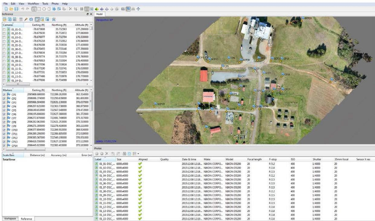
Figure 6: Ground control points view in Agisoft PhotoScan
