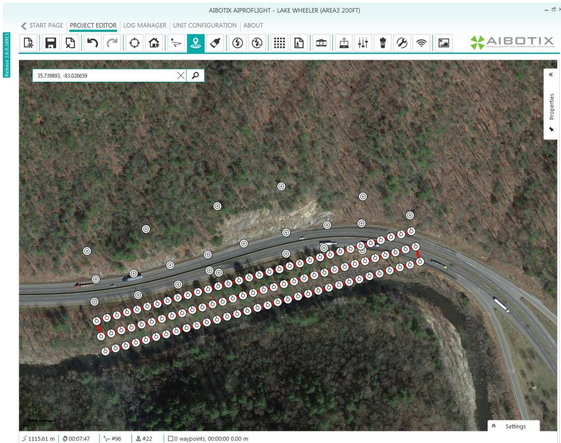
Figure 20: Haywood County Ground Control Points and Flight Plans (Proposed Locations)
