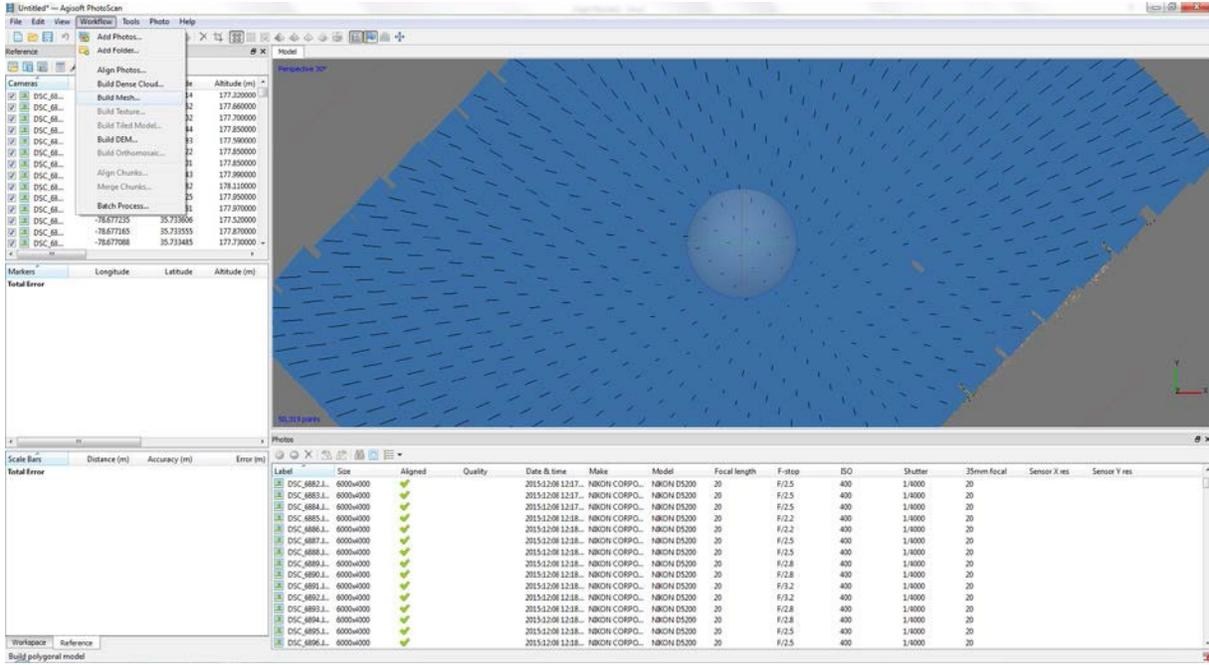
Figure 75: Build Mesh Cloud interface in Agisoft PhotoScan
