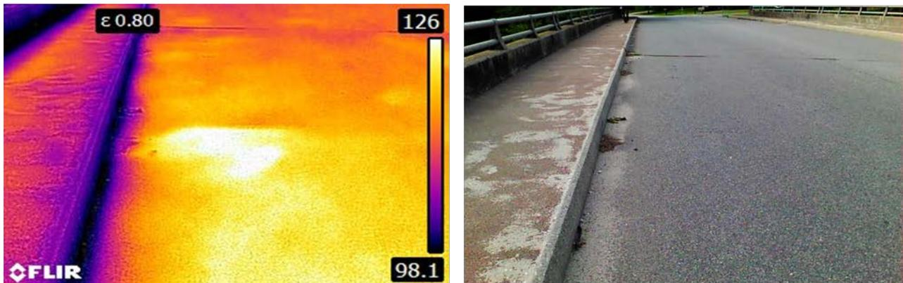
Figure 40: Example 2 of Unknown Damage, Left E4 Thermal and Right E4 RGB Image
