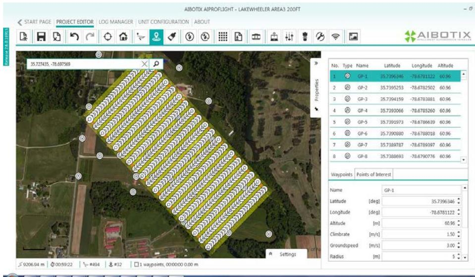
Figure 13: Lake Wheeler FP Elevation 60.96m [200 ft] (70/40% Overlap)
