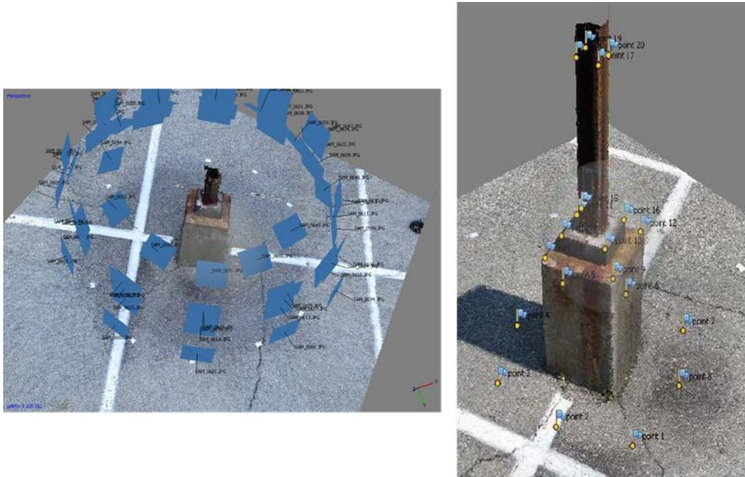
Figure 8: Camera Positions for Samsung NX30 16mm Lens Camera Calibration
