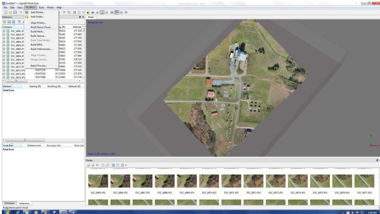
Figure 73: Build Dense Cloud interface in Agisoft PhotoScan
