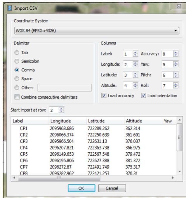
Figure 71: Import a file with the original GCP points
