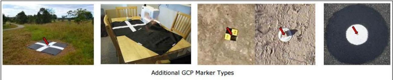
Figure 27: Example Ground Control Points
