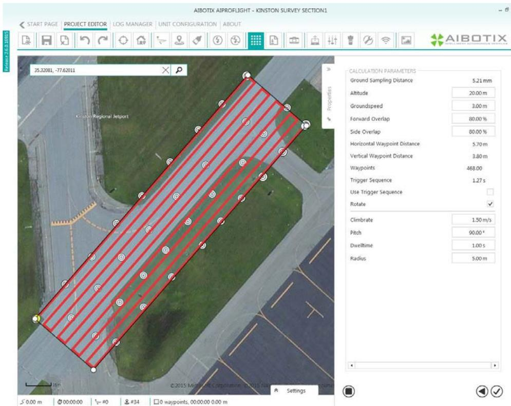
Figure 15: Kinston Area 1 FP Elevation: 20m (Planned)
