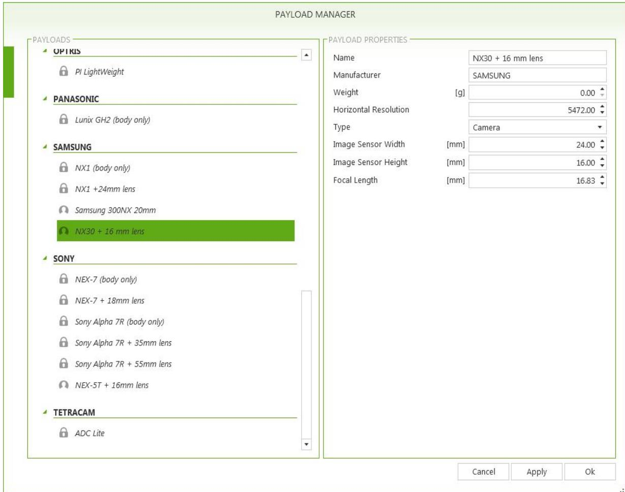
Figure 9: AiProFlight Payload Manager: NX30 16 mm lens Camera Calibration
