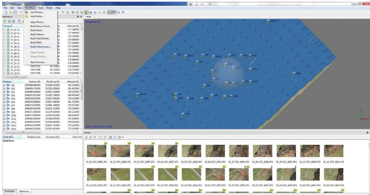
Figure 82: Build Orthomosaic interface
