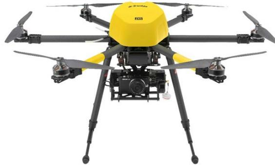
operations the flight is preprogrammed into the GCS and the flight is executed autonomously. It requires two 6600 mAh batteries that gives it an endurance of 20 minutes.
