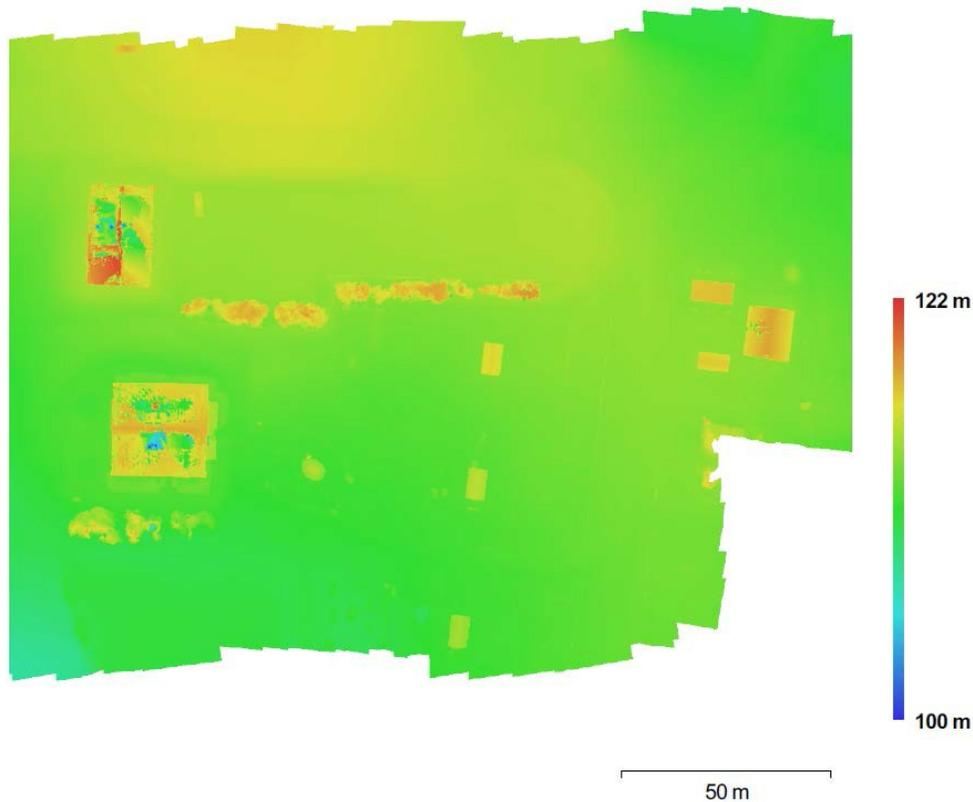
Figure 35: DEM from 67' flight, 60-60 Overlap
