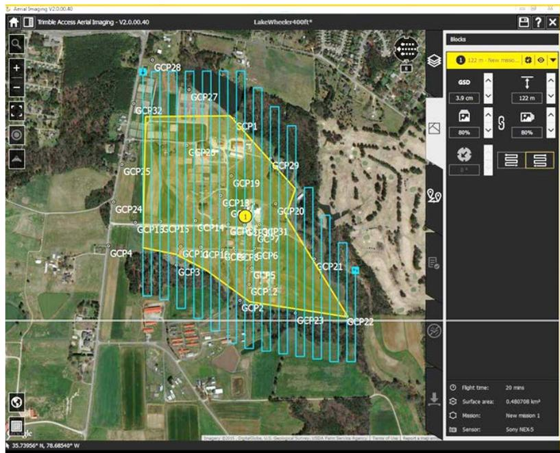
Figure 3: A Sample UX5 (fixed wing) Flight Profile at Lake Wheeler
