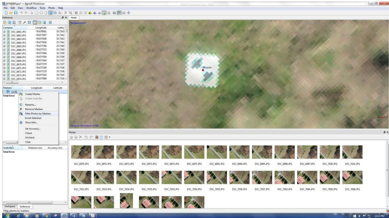
Figure 67: Align photos by place marker
