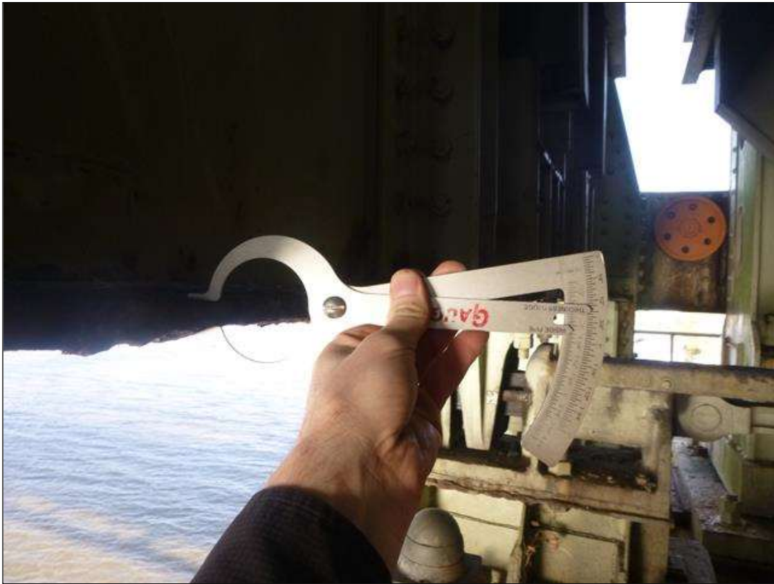
Span 18 Lift Span Floor Beam 12: LOSS OF SECTION .680" WITH .628" REMAINING BOTTOM EAST FLANGE 17' LONG X UP TO 5-1/2" WIDE BETWEEN LEFT LOCK AND CENTERLINE SUPPORT PEDESTAL. (PAR)
