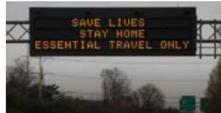
The installation and use of DMS in Cherokee and Swain Counties would alert travelers to delays, detours and hazards during and post-storms and rockslides, accidents and road closures. These electronic signs deployed along this improved route would convey public service messages, state of emergency and current traffic conditions. Additionally, if installed prior to construction, the signs would assist during the construction period to alert drivers of delays and the current construction schedule.
