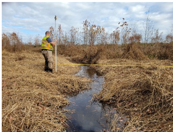
Cross-section survey of the stream channel at R-2554 Claridge Nursery.
