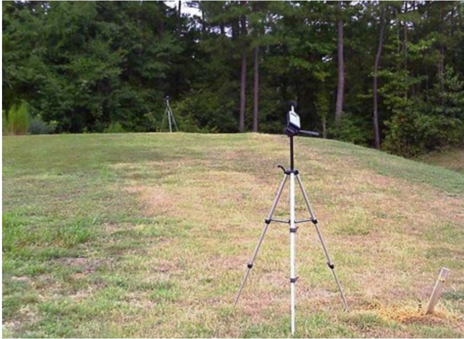
Figure 7-2. Ambient Noise Measurement Set Up
