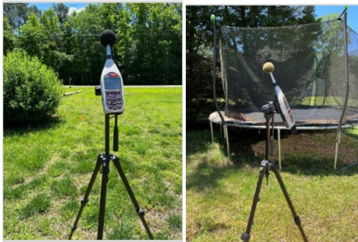
Figure 7-8. SLM Microphone at 90 Degrees or Grazing Incidence
