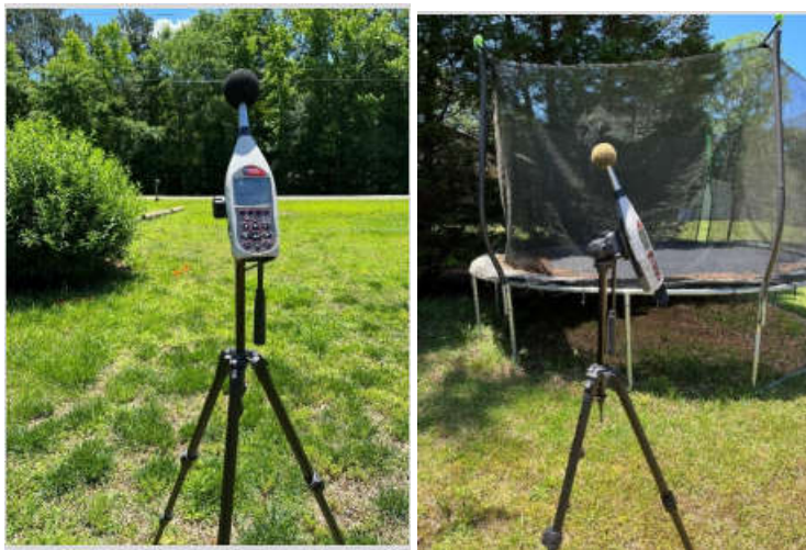
Figure 7-8. SLM Microphone at 90 Degrees or Grazing Incidence
