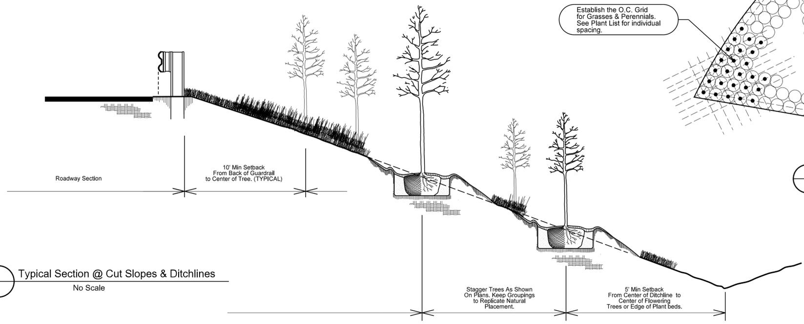
**Typical Section @ Cut Slopes & Ditchlines**
