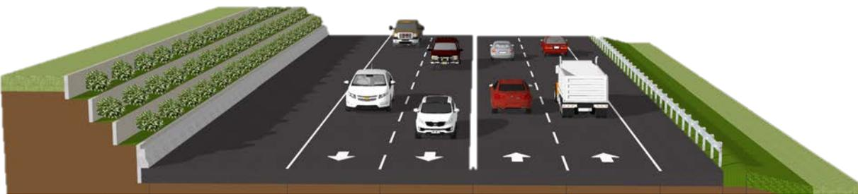
**Figure 3: NC 143 Typical Section at Stecoah Gap.** Climbing lanes in both directions creates a four-lane cross-section at Stecoah Gap, creating a potential hazardous crossing for wildlife, ANST users, and motorists.
