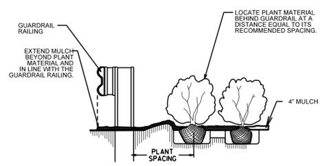
**GUARDRAIL MULCHING DETAIL**
