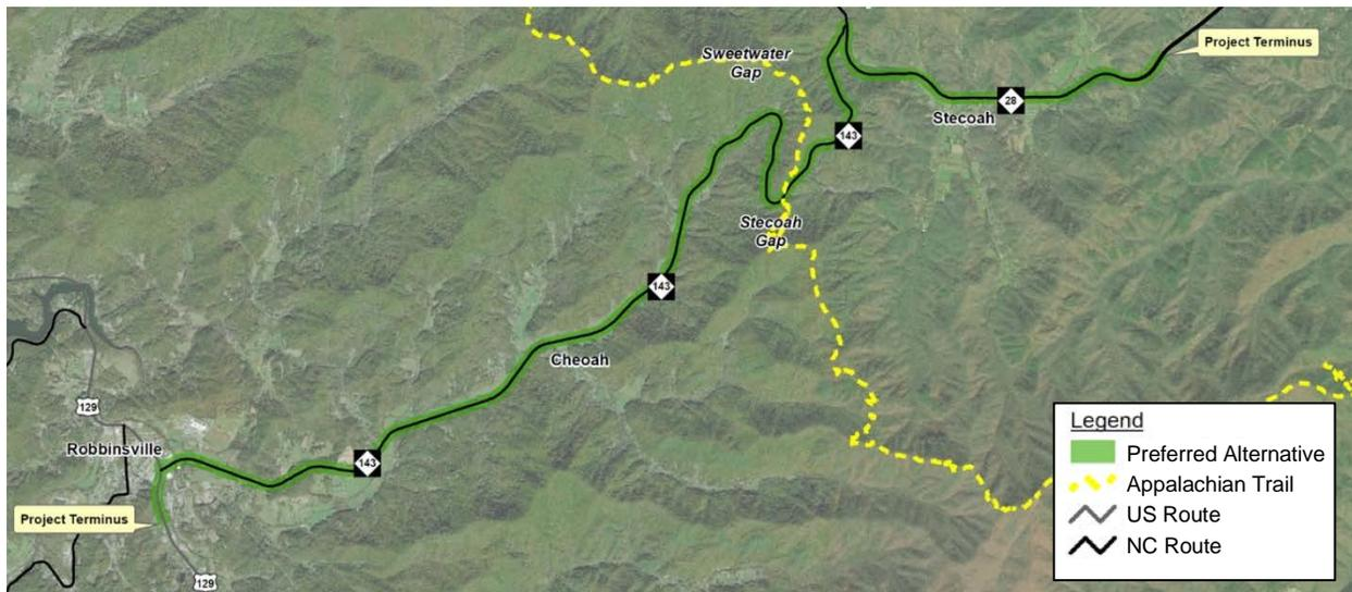
**Figure 2: Project Corridor.** The wildlife crossing will be constructed over NC 143 at Stecoah Gap near the current location of the Appalachian Trail crossing shown here.
