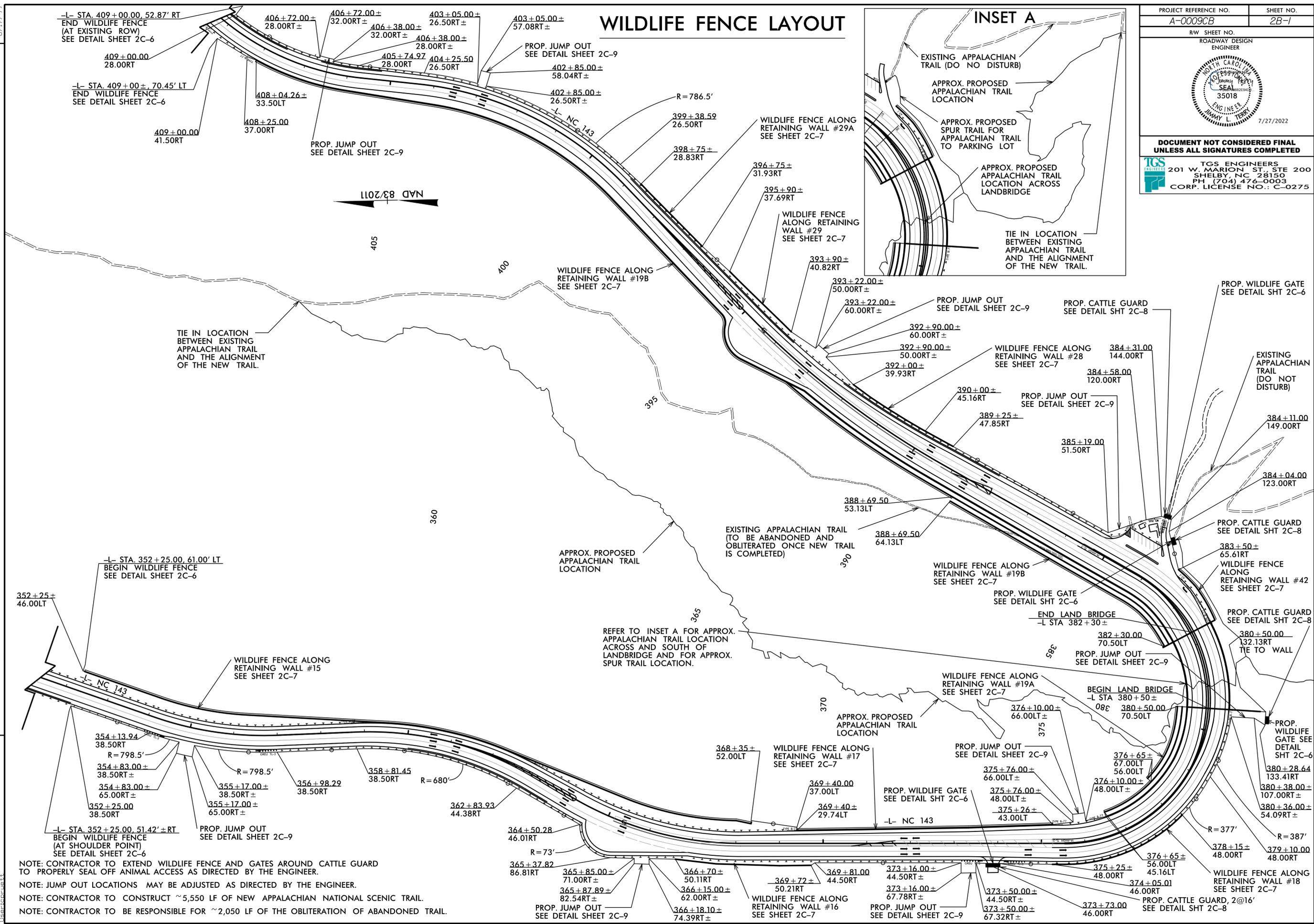
NOTE: CONTRACTOR TO EXTEND WILDLIFE FENCE AND GATES AROUND CATTLE GUARD TO PROPERLY SEAL OFF ANIMAL ACCESS AS DIRECTED BY THE ENGINEER.
