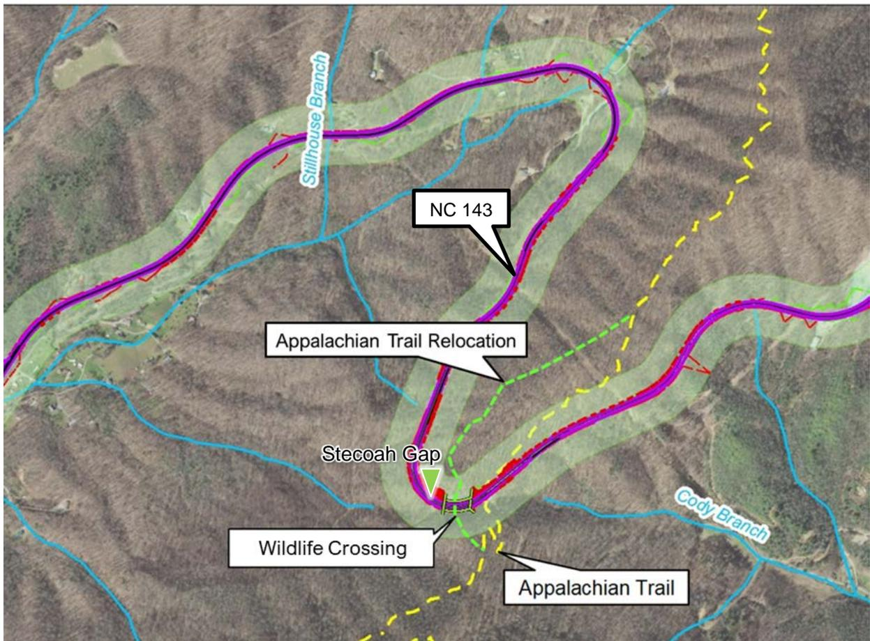
**Figure 5: Wildlife Crossing Schematic.** As part of the Corridor K project, a wildlife crossing is proposed over NC 143 at Stecoah Gap. The ANST (shown in yellow) would be relocated to the wildlife crossing and the realigned for a short distance (shown in green). Fencing will be erected on each side of the wildlife crossing (on both the north and south sides), 0.5-mile on each approach, to direct animals to the crossing.
